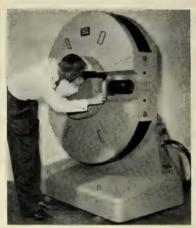
aerodynamic studies, for thermal-barrier studies in ballistic investigations (such as nose cone re-entry problems), for hypersonic wind tunnel instrumentation and for exploring the behavior of rocket propellants.
