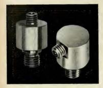
Now you can avoid one of the major causes of false test results – spurious "ground loop" voltages – by using internally ungrounded GLENNITE accelerometers.
