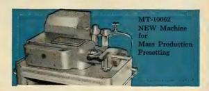
The fully automatic Presetting Machine contributes to production line speed and efficiency in presetting MS(ER)® sleeves. It has single push button control and single air pressure setting of all sizes for fast, easy operation. It correctly presets sleeves on aluminum, carbon or stainless steel tubing in all standard sizes ½8″ through 2″ in diameter.
