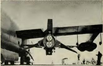
X-15 ROCKET-POWERED high-altitude research craft attached to its pylon under the wing of the B-52 mother ship. Three main fittings secure the X-15 and additional quick disconnect lines allow a launch panel operator in the B-52 to feed nitrogen and LOX to the rocket ship.
