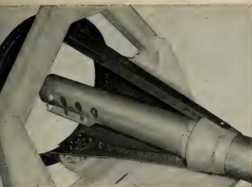
NOSE CONE SPLICE JOINTS ARE FASTENED WITH HS47 PINS, TYPE 431 STAINLESS STEEL, HEAT TREATED TO 125,000 PSI MINIMUM SHEAR. THE HS60M COLLARS ARE R MONEL.
