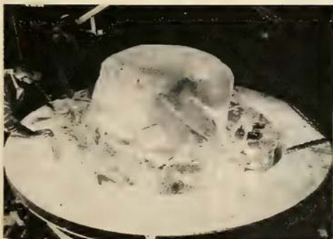
THE FIRST large-sized ribbed disk (84-in. diameter) is made by sagging. Scrubbed clean by sandblasting, glass is now ready for the melting furnace.
