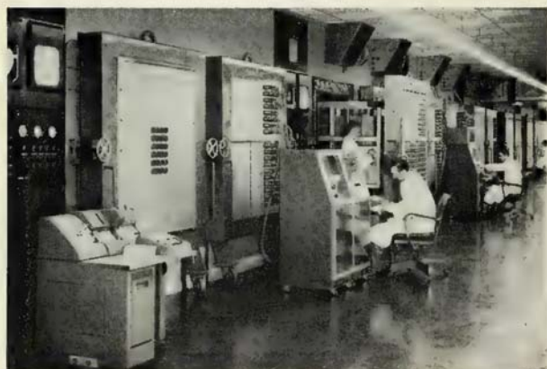
A ROW OF Inland's environmental chambers with automation equipment in front of doors. Accuracy is closely checked.
