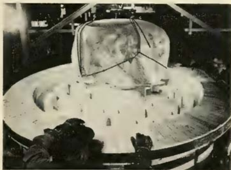
MOLD'S CENTER core had to be reinforced by a steel plate. One reason was this 2796-pound chunk of boro-silicate composition glass.
