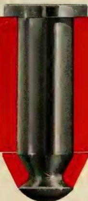
NOSE CONE SPLICE JOINTS ARE FASTENED WITH HS47 PINS, TYPE 431 STAINLESS STEEL, HEAT TREATED TO 125,000 PSI MINIMUM SHEAR. THE HS60M COLLARS ARE R MONEL.
