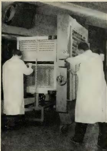
COMPONENTS ARE mounted on frames which are part of a chamber door assembly.
