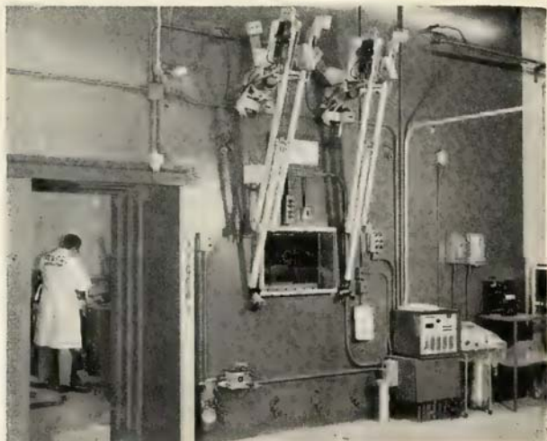
COBALT 60 cells for radiation testing. A gate circuit is used to guard against loss of component identification.
