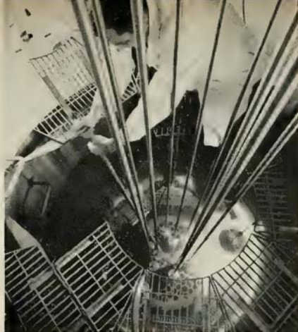
NUCLEAR RESEARCH. At the Westinghouse Testing Reactor, engineers are preparing high intensity radiation tests on a wide range of materials to determine their structural, chemical, and nuclear stability. This is a necessary prelude to using these materials in certain atomic power applications; now under development. Atomic Power Department
