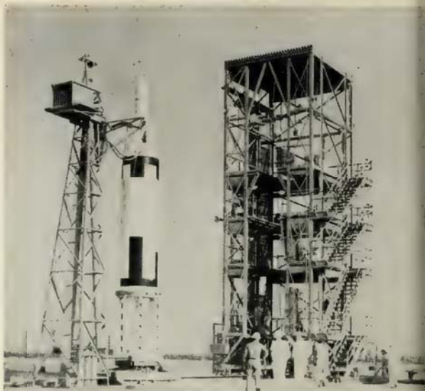
UMBILICAL CORD attached ready to fire, the gantry crane is moved away. The AX-4 was the 26th flight of the Polaris test program. Flight was reported a "partial success" after malfunction caused range destruct.
