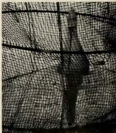
NET CATCHES scale model of Navy's Polaris in underwater launching tests.
