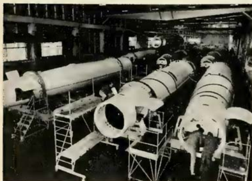
THREE Thors , minus warheads and nose cones, have guidance systems installed on the final assembly line at the Douglas Santa Monica plant.
