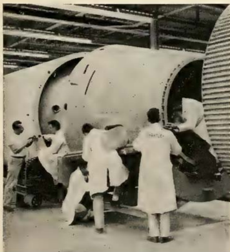
BODY SKIN for Jupiter is rolled and joined by automatic welding equipment in the fabricating tank section of the Chrysler Corp.'s Missile Division.
