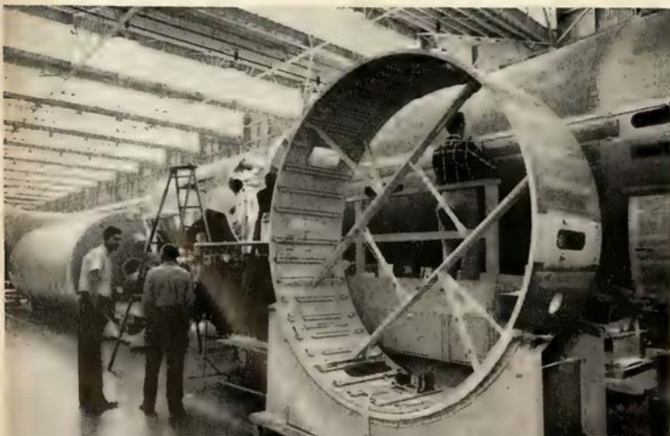
THE 150-165,000-lb. thrust engine system for Thor is joined to the engine body section. Missile is reported to cost between $650-700,000 dollars.
