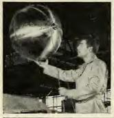
Successful titanium welding techniques have enabled fabricatars to praduce missile prapellant starage battles which resist internal pressures af 8000 psi at -300°F. This all-titanium battle, praduced by Rheem Manufacturing Campany, Dawney, Calif., is Ti-6Al-4V, fusian-welded in an argan atmasphere. Designers say use af titanium battles can add up ta 700 miles to the range of an IRBM.
