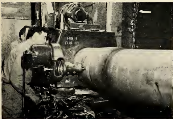
ASSEMBLED epoxy laminated Nike-Ajax booster is secured in jug chuck for drilling access holes.
