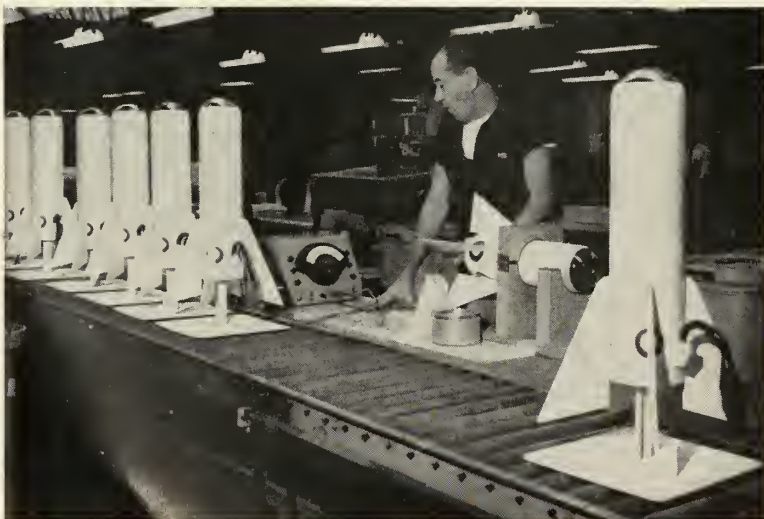
GUIDANCE AND CONTROL sections of the Sidewinder missile in final checkout before shipment by Philco. This is first Sidewinder production view released by the Defense Department. Missile is used by Navy's Sixth and Seventh Fleets and by AF F-104A.
