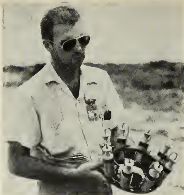
EIGHT VERNIER ROCKETS of third stage adjust its speed after separation.
