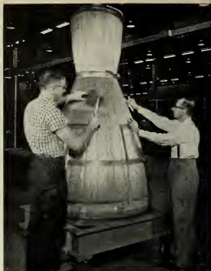
FORMED TUBES are stacked on mandrel.
