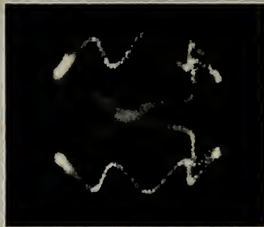
Charged aluminum particle suspended and controlled in a vacuum chamber by an oscillating electric field.
