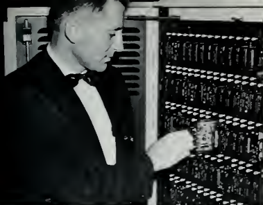
Launching and control order computers for TARTAR Missiles. Electronic and electromechanical portions of this all-transistorized modular computer are shown at left and right.
