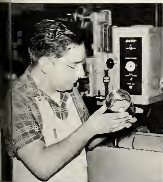
A special machine is used to mill irregular internal contours by an "electrical discharge" method, with extreme dimensional accuracy.
