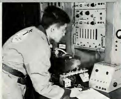
Missile-borne inverter. Vital missile component gets rigorous, precision performance checkout at console. All of the missile products delivered by Ford Instrument undergo full and complete testing procedures.
