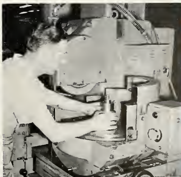
Technician grinds gyro part to a length within 20 millionths of an inch—typical of tolerances being met in missile work at Ford Instrument.
