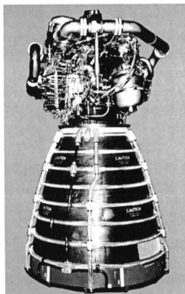
Figure 21: The Space Shuttle Main Engine (SSME). Credit: Authors/USS&RC.
