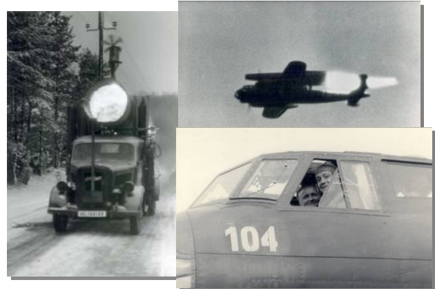
Ramjet trials, first on an Opel truck, later on Dornier planes as flying test beds.
