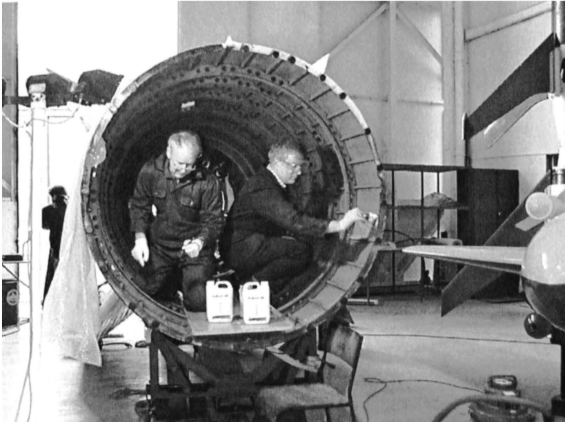
Figure 6: The inside of the tail section being treated with corrosion inhibitor - Trustran 40.
