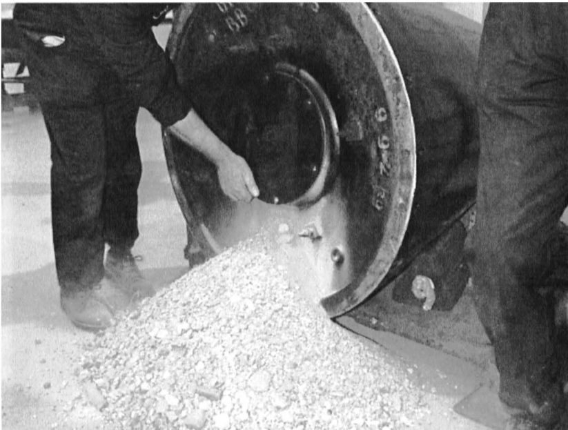
Figure 2: When the warhead was removed it was found to be full of Cuxhaven sand and pebbles, presumably to match the weight of the explosive charge that would have been fitted.
