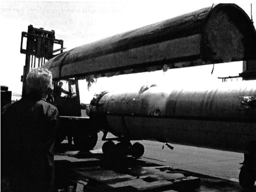
Figure 10: Separating the V-2 tank section body reveals the propellant tanks and the glass wool insulation.
