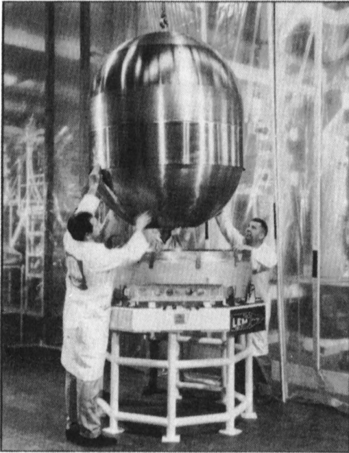
Figure 21 Descent stage tank being mounted in its structural support.
