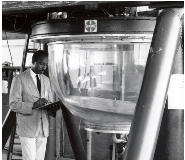
Above: Plexiglas slosch rig at Grumman, 1965. Results from these tests led to the small anti-vortex baffle which was insufficient to cope with propellant slosh. (Courtesy Northrop Grumman History Center)
