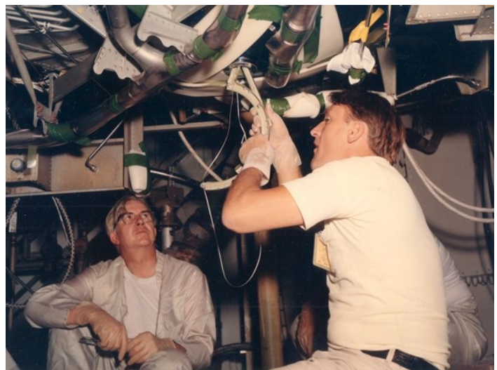
Above: Technicians demonstrating the baffle install technique on a LM Test Article at White Sands, New Mexico. Note the small 2.4 inch diameter hole where the Propellant Quantity Gauge is bolted to the bottom of the tank. (Courtesy Northrop Grumman History Center)
