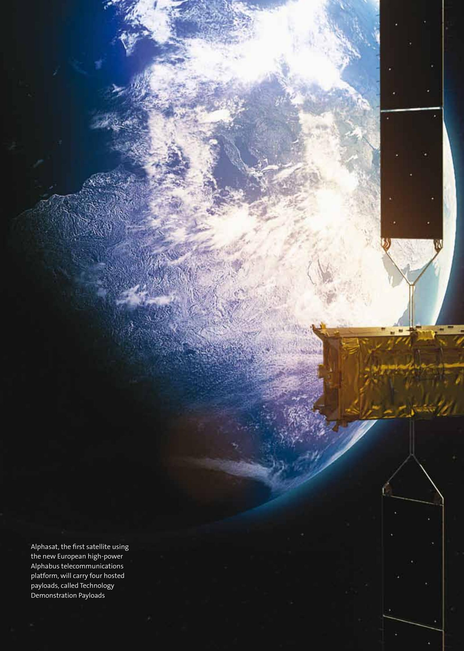
Alphasat, the first satellite using the new European high-power Alphabus telecommunications platform, will carry four hosted payloads, called Technology Demonstration Payloads
