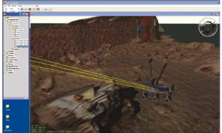
↑ A new software tool known as the 3DROV planetary rover simulation environment allows early-stage virtual modelling and 'shakedown' testing of mobile surface missions for both Mars and the Moon
