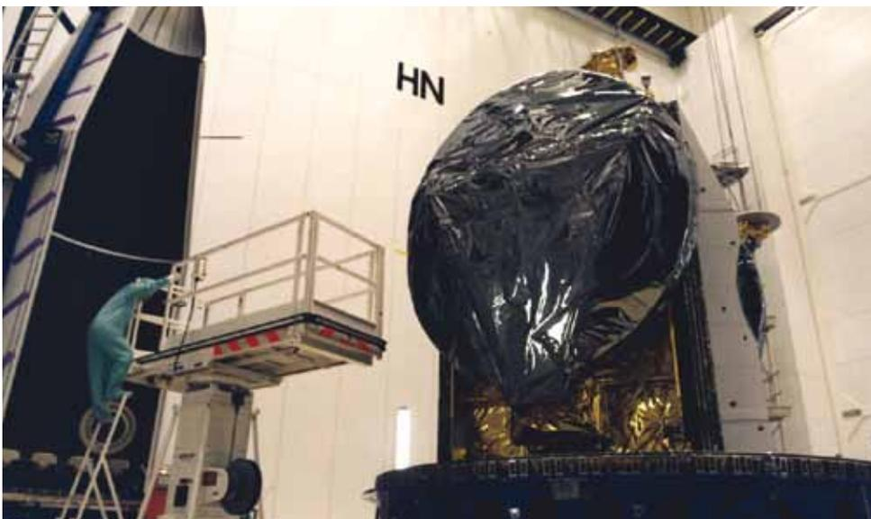
← Eutelsat's Hot Bird 4 satellite carried the Skyplex processor, also supported through ESA's ARTES programme
