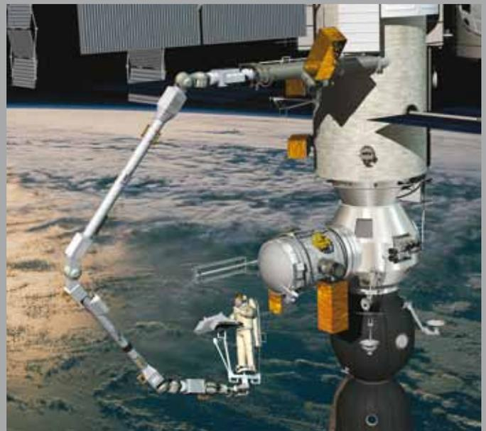
Artist impression of the European Robotic Arm, which will be sent to the ISS with the Russian Multi-purpose Laboratory Module on a Proton launcher in 2013
