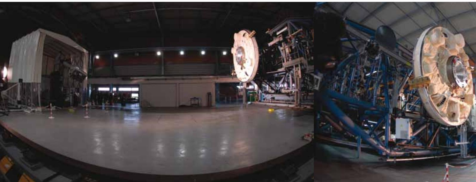
↑ ↗ Automated Transfer Vehicle (ATV) physical docking simulator at Val de Reuil, France
