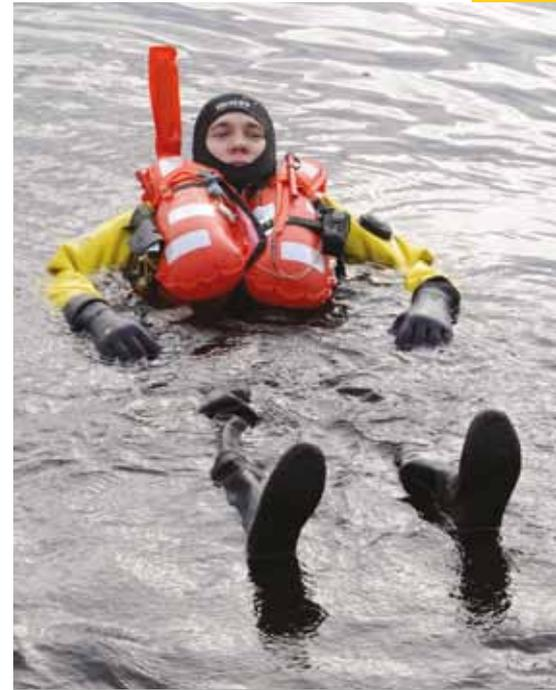
↑ A life vest with an incorporated search and rescue antenna being tested in a field trial in Finland
