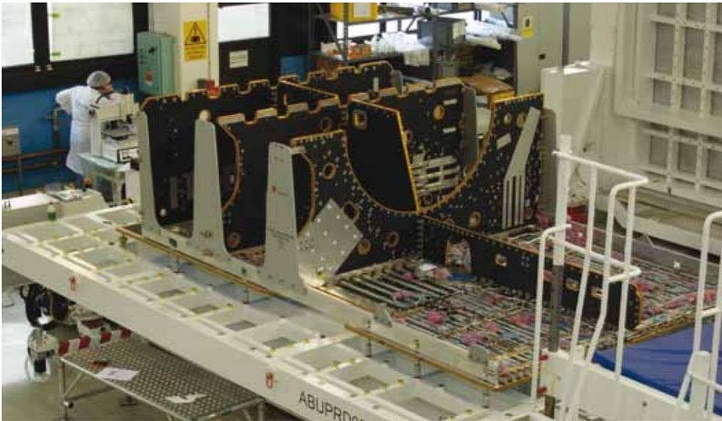
← Half of the repeater module of Alphasat during construction at Thales Alenia Space Italy in 2009
