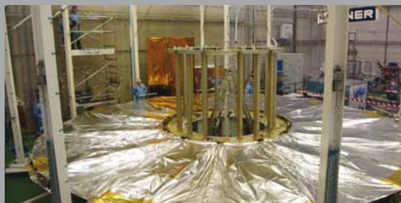
The Gaia Sun Shield fully deployed in the Sener clean room
