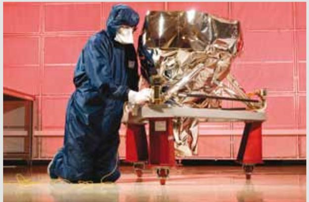
MIRI optical system Flight Model after cryogenic testing
