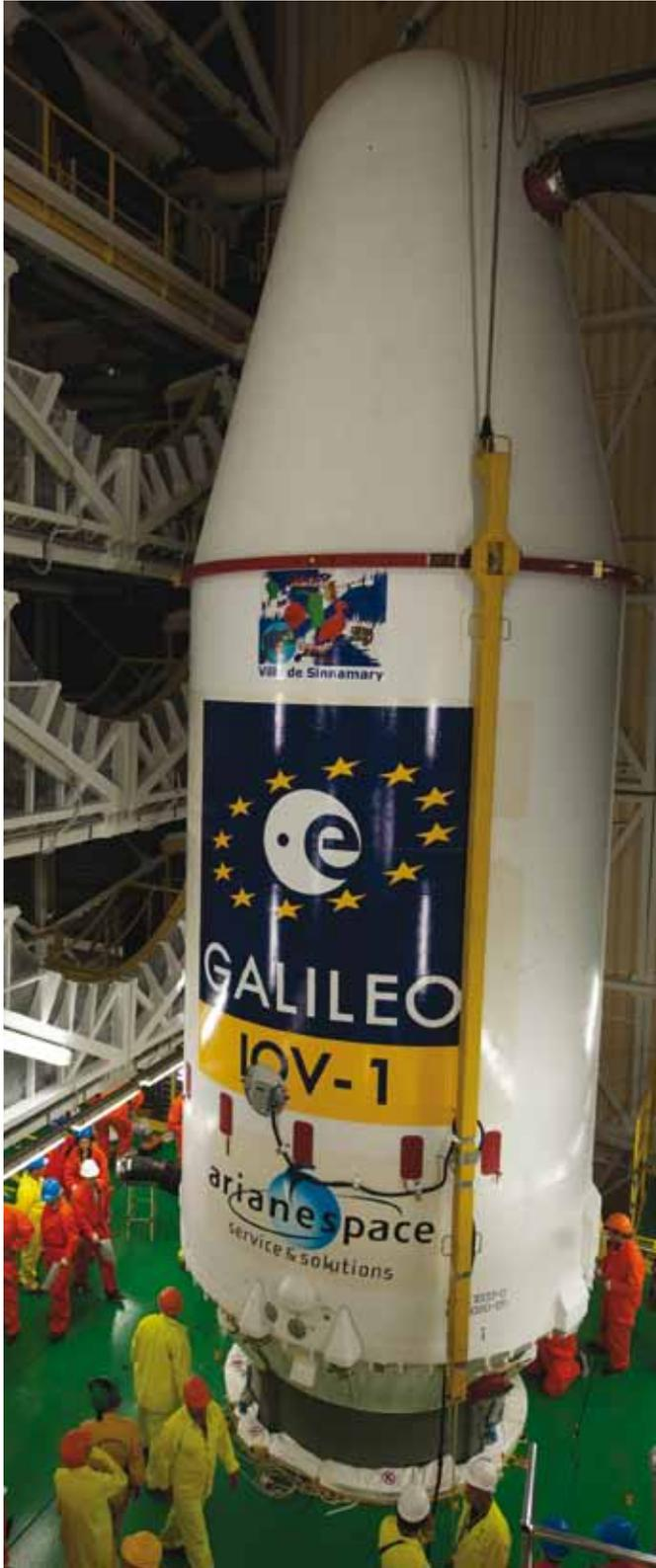
↑ The 'Upper Composite', comprising the Fregat upper stage, the Galileo satellites and fairing, put on top of the Soyuz launcher, completing the very first Soyuz vehicle on its launch pad at Europe's Spaceport
