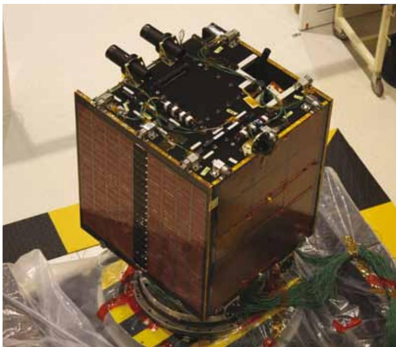
↑ Proba-V Structural and Thermal Model during testing in Toulouse, France, in 2010 (Intespace)
