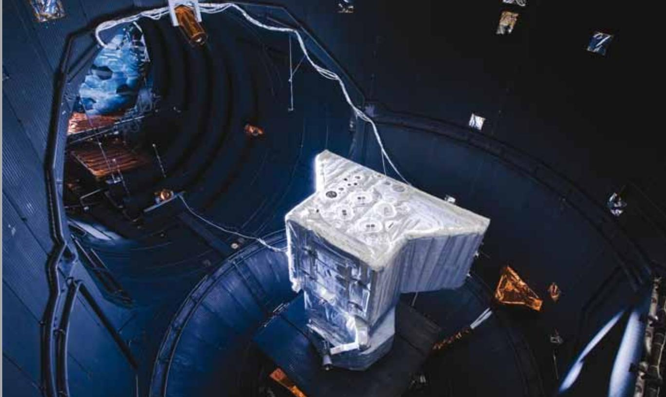
BepiColombo's Mercury Planetary Orbiter STM in the Large Space Simulator at ESTEC
