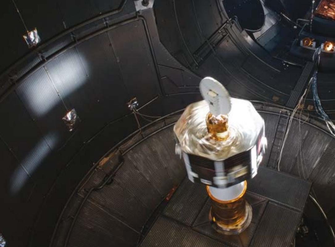
BepiColombo MMO Thermal Model in the Large Space Simulator at ESTEC
