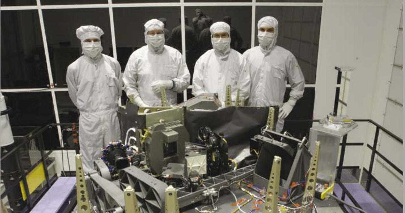
Complete integrated NIRSpect flight instrument before cover integration
