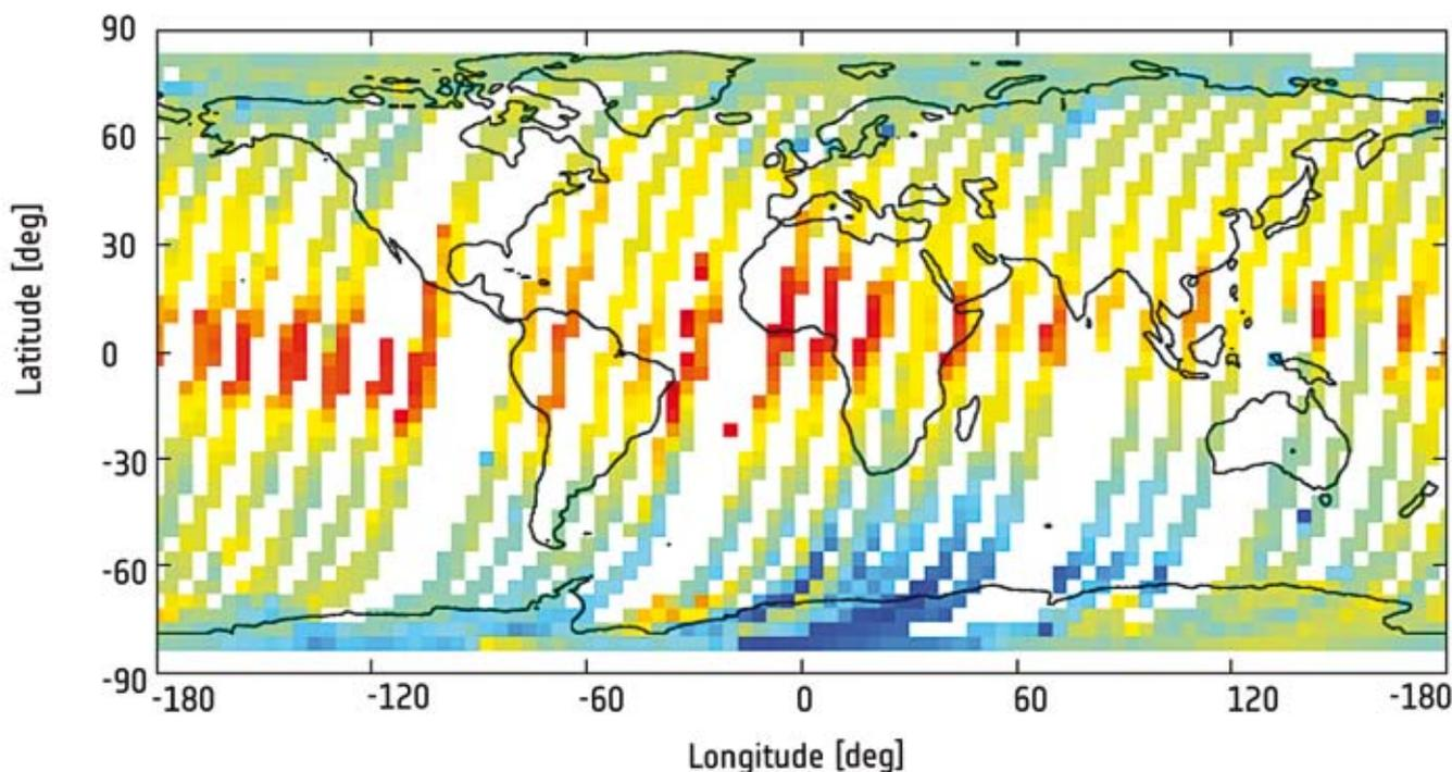
↑ Electron density map based on DSLP measurements
