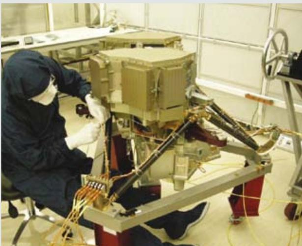
MIRI instrument ready for vibration test
