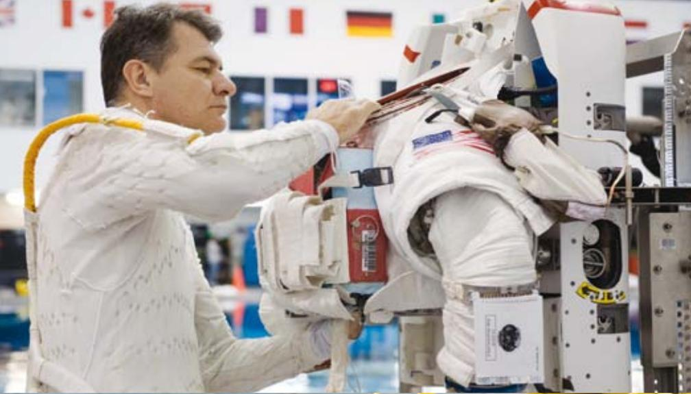
← The full Extravehicular Activity (EVA or spacewalk) training for the ISS is traditionally done in the giant pool of NASA's Neutral Buoyancy Laboratory, Houston. Here Paolo gets into a training version of his 'Extravehicular Mobility Unit', his white spacesuit worn during spacewalks which is like a personal 'mini-spacecraft'
