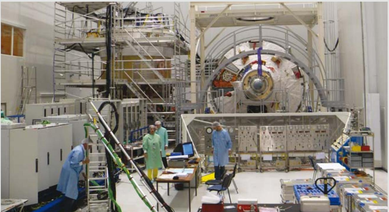
The mating of ATV *Johannes Kepler's* Service Module and the Integrated Cargo Carrier took place at the end of October. Here, all the components are being prepared for mating in the S5C hall at Kourou, French Guiana
