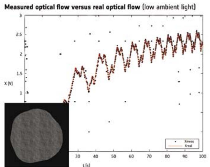
↑ Example of the performance of one of the elementary motion detectors studied (from the group at the Université de la Méditerranée in Marseille) during a fast spiral descent on a virtual asteroid (lower left corner) under critical lighting conditions as simulated using the software PANGU. Light direction is assumed for simplicity to be always at zenith. The total avionics payload of the sensor would have a mass of less than 10 g and consume less than 1W of power.
