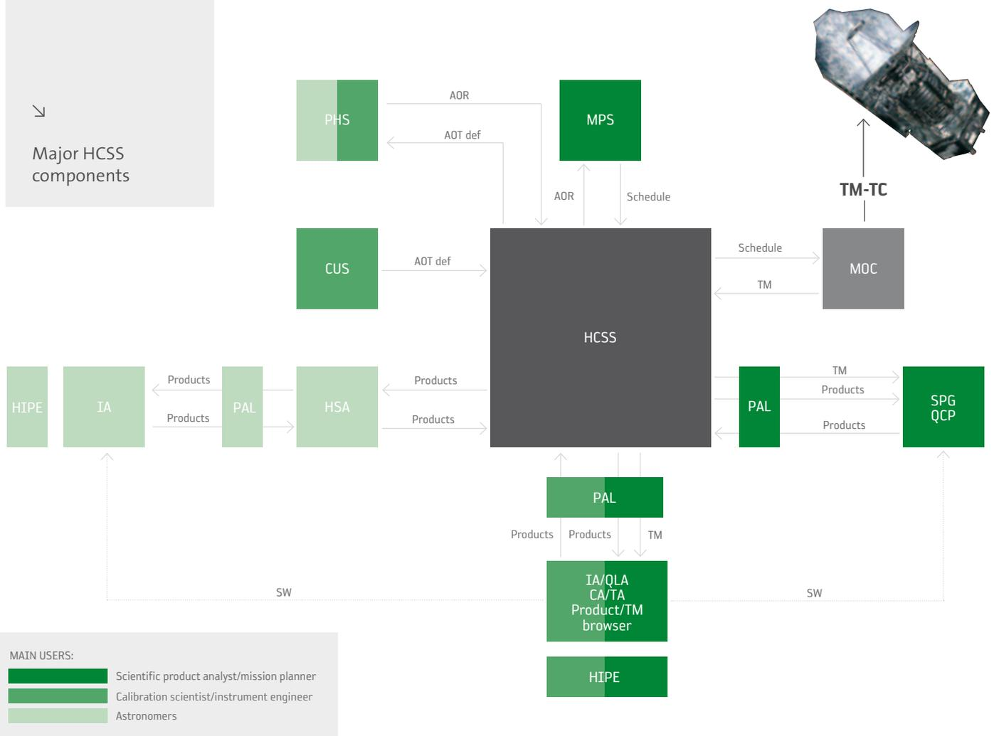
for a particular observation converts the AOT into an Astronomical Observing Request (AOR) that is stored in the database.
