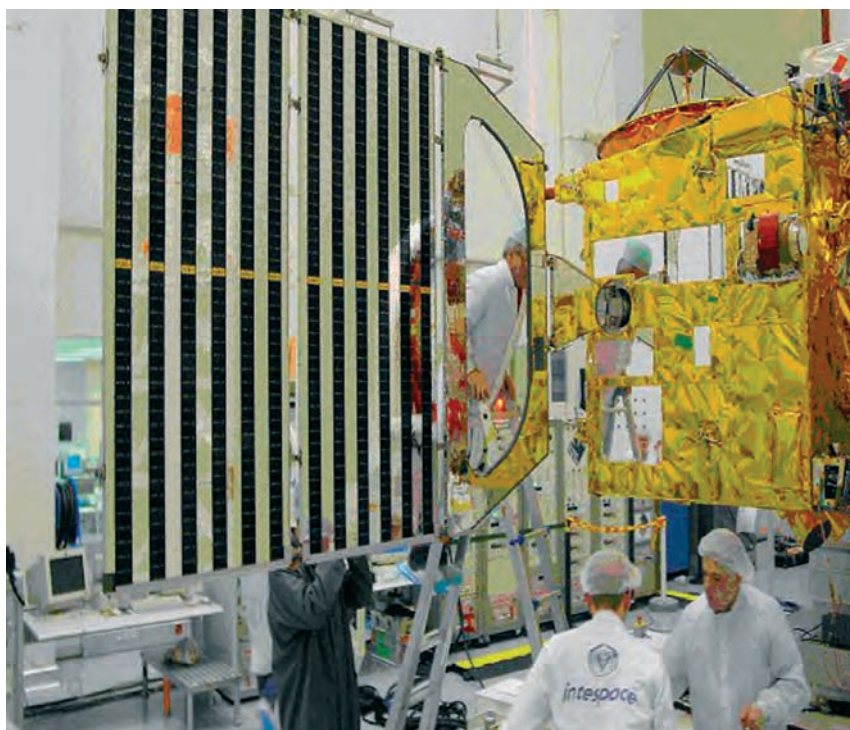
One of the solar-array wings after a successful deployment test at Interspace in Toulouse (F)
