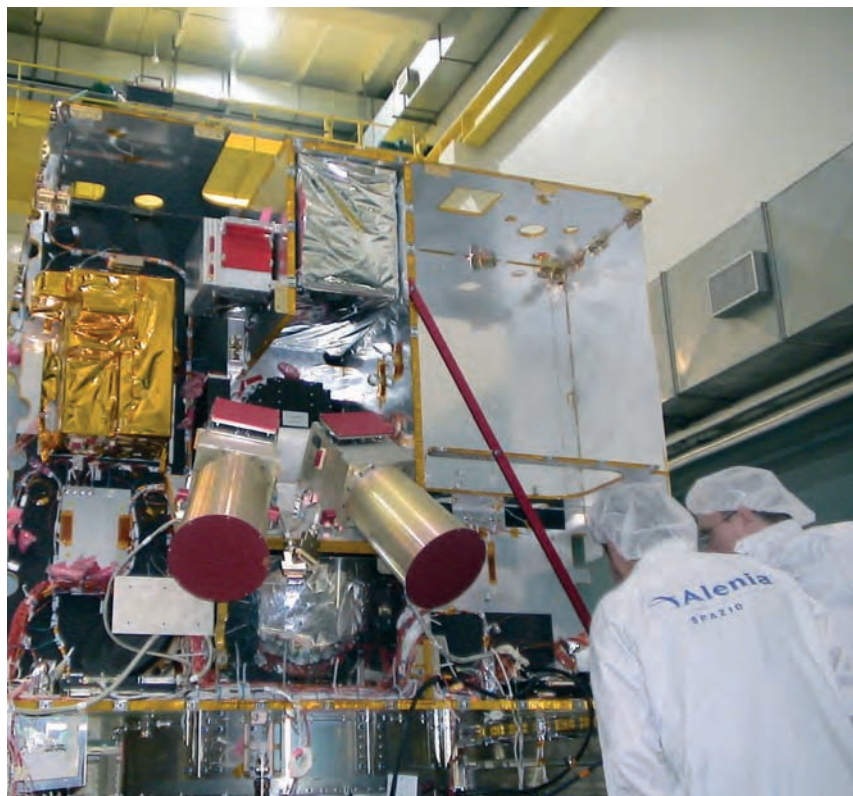
The spacecraft undergoing integration at Alenia in Turin (I)
