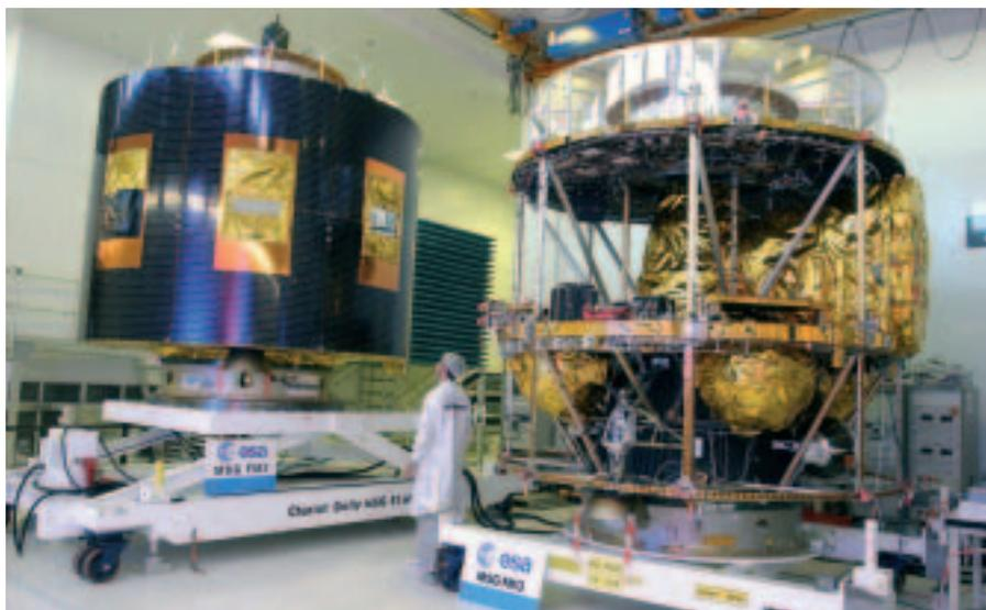
Flight models of MSG-2 and MSG-3 in the clean room at Alcatel Space in Cannes (F)
