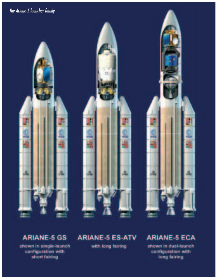
launcher is protected by a payload fairing during the atmospheric flight phases. It is a lightweight carbon-sandwich structure and is produced in three lengths to accommodate different sizes of payloads. The fairing length may be further increased in height by adding cylindrical sections (Adaptateur Cylindrique, or ACY).
