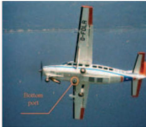
The SmartScan airborne flight-test configuration
