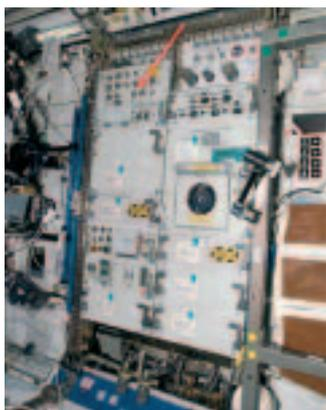
Housed within the Human Research Facility #2, the Pulmonary Function System installed in the ISS's Destiny laboratory
