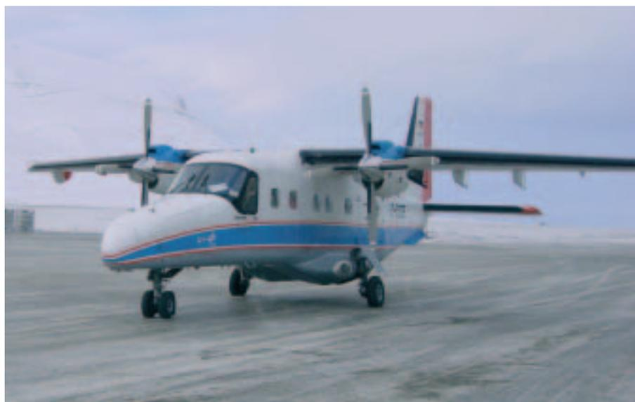
*The AWI Dornier 228 aircraft carrying the ESA radar altimeter ASIRAS along with a laser altimeter. This aircraft was used for 2004 pre-launch validation experiments focused mainly on land-ice validation*
