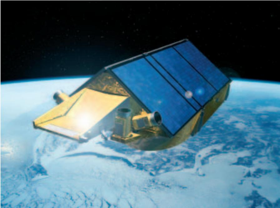
*Artist's impression of CryoSat in orbit, flying almost towards the viewer. The prominent features visible are the solar arrays, giving a roof-like appearance, and the three star trackers which are mounted on the rigid structure supporting the SIRAL antennas. The structure forming the 'nose' at the very front of the satellite is a thermal radiator for the heat generated by the SIRAL instrument*
