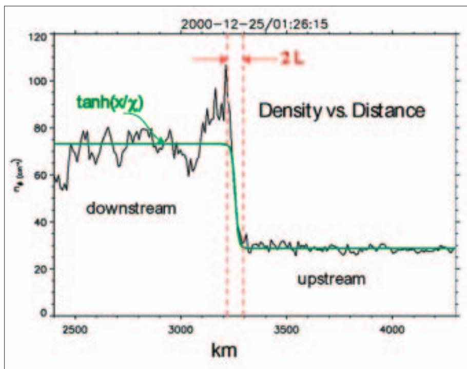
Density transition from downstream to upstream across the Earth’s bow shock in the solar wind. The green line is a theoretical fit; the red vertical lines show the thickness of the shock (Courtesy of S. Bale, University of California at Berkeley)
