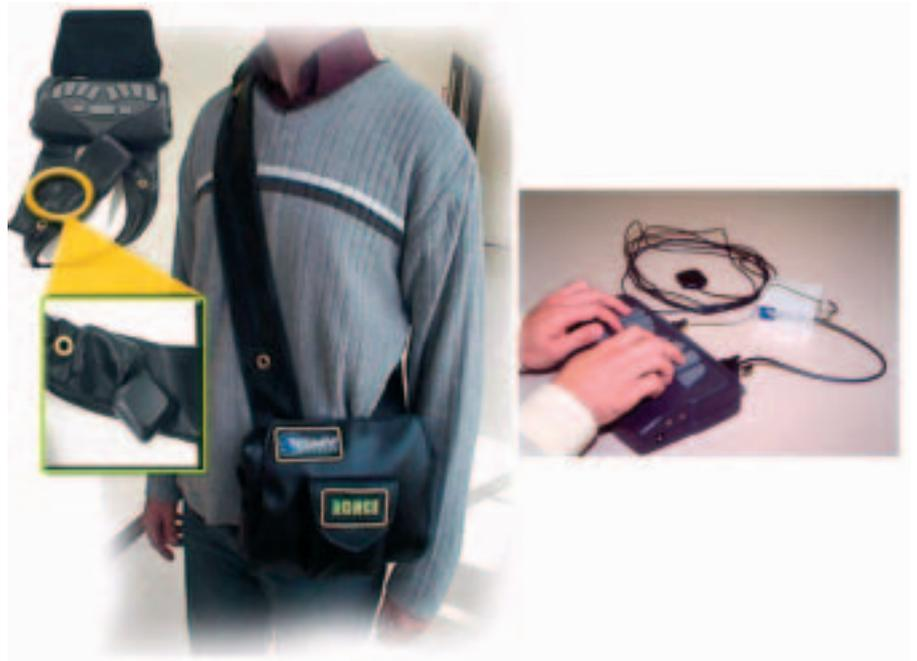
*TORMES: A personal navigator for the blind, enhanced with SISNeT capabilities, developed by GMV Sistemas (Spain) and ONCE (the Spanish Organisation for the Blind). This device has highlighted the immense benefits that the synergy between Satellite Navigation and Communications can bring to visually impaired people*
