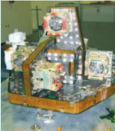
*GOCE Gradiometer structural thermal model's core*
