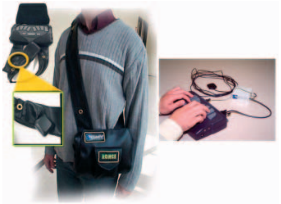
TORMES: A personal navigator for the blind, enhanced with SISNeT capabilities, developed by GMV Sistemas (Spain) and ONCE (the Spanish Organisation for the Blind). This device has highlighted the immense benefits that the synergy between Satellite Navigation and Communications can bring to visually impaired people
