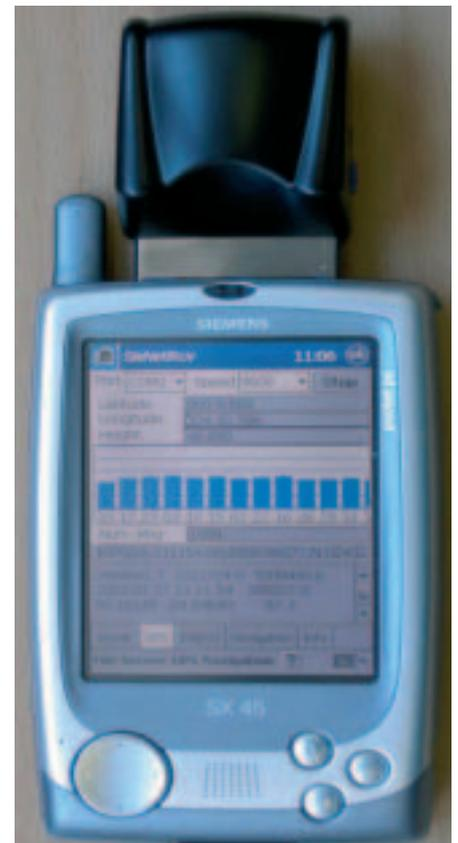
During field testing in Finland, the new receiver delivered horizontal positioning accuracies of 1-2 metres and vertical accuracies of 2-3 metres. In a further step, the device has been integrated into a Siemens SX45 mobile phone.
