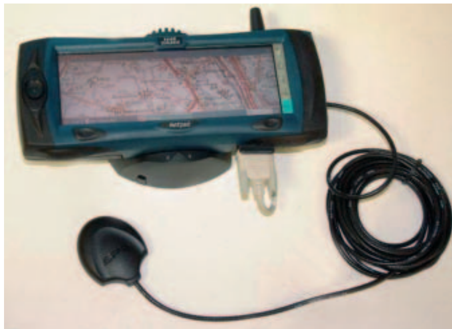
SISNeT receiver based on a PDA device, integrating a GPS receiver and a wireless link to the Internet in a single box. It has demonstrated the benefits of the ESA EGNOS-SISNeT technologies for urban bus-fleet management systems. This receiver has been developed by Navocap (France) under ESA contract
