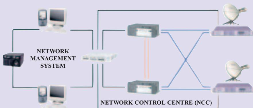
Connection-control management functions both support permanent connection set-ups and handle on-demand connection requests, such as call establishment, call modification and call release.
