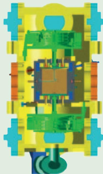
*The LTP inertial sensor. The proof mass is surrounded by the electrode housing and is located in a vacuum enclosure. Optical windows allow the laser beam to be reflected by the face of the cube. UV optical fibres within the enclosure illuminate the cubes in order to discharge any charging produced by cosmic rays. The proof mass is kept in a safe position during launch by a 'caging' mechanism.*
