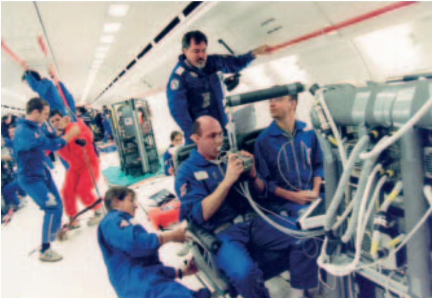
*The ARMS equipment was used onboard the Airbus A300 'Zero-G' for several respiratory experiments in 1999. Here Prof. G.K. Prisk (Univ. California, San Diego, USA) is monitoring ESA astronaut Andre Kuipers acting as the test subject*
