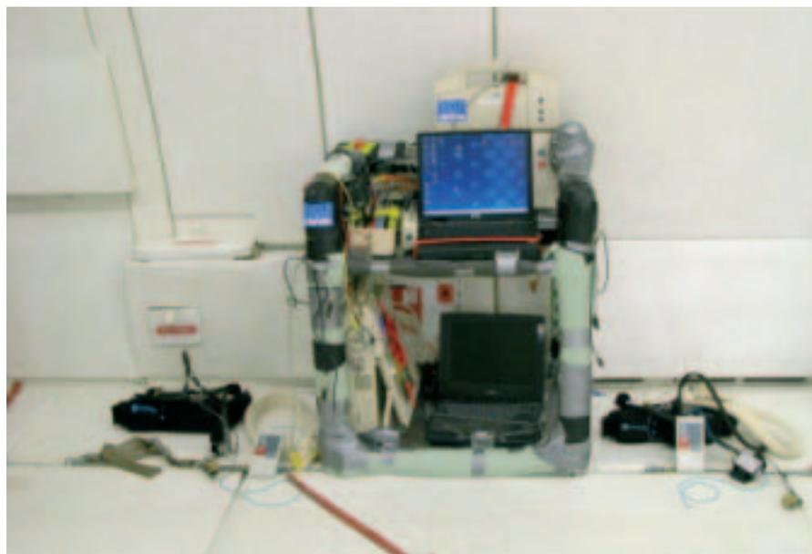
A typical instrumented rack for cardiovascular measurements as used by A.E. Aubert et al. during the 36<sup>th</sup> ESA Parabolic-Flight Campaign in March 2004 (photo A.E. Aubert)
