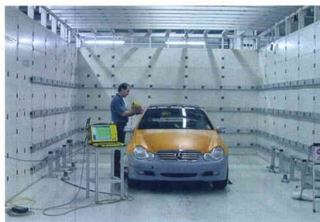
Preparing for ProCam measurements on a vehicle to be crash-tested with reference points on the walls of the measurement chamber
