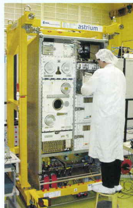
The flight model of Biolab during its testing in the Columbus Rack-Level Test Facility (RLTF) in Bremen, Germany
