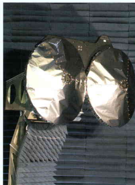
The CryoSat SIRAL antennas ready for electrical performance testing at Saab (S)
