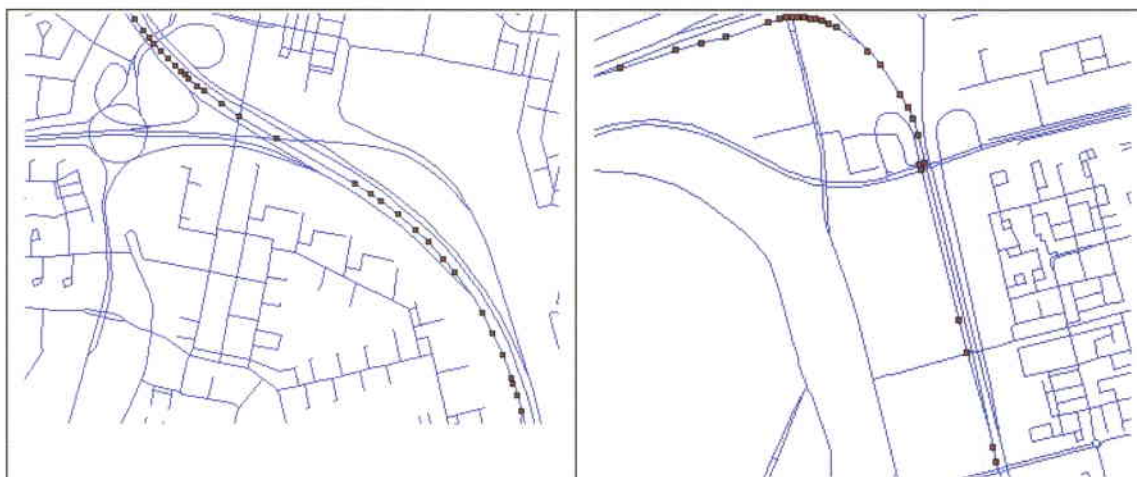
Examples of a good map match (left) and a failed match (right) in a complex motorway situation where the vehicle is erroneously located in the exit lane rather than in a motorway lane
