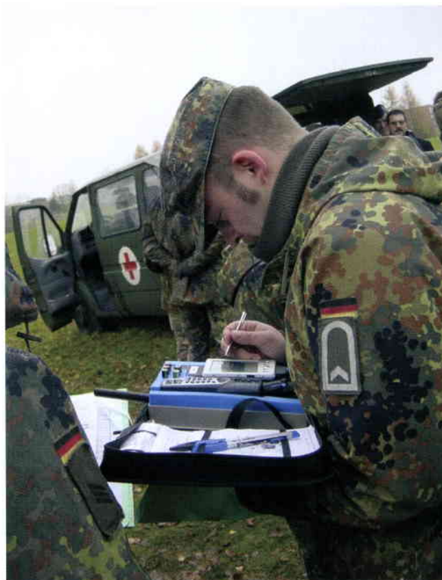
Project DELTASS: the portable terminal used by the Search & Rescue (SAR) teams to fill in the electronic patient record card. The link with the coordination centre is via the Globalstar satellite system
