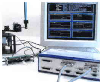
xPC Target and xPC TargetBox enable real-time rapid control prototyping of embedded designs.
