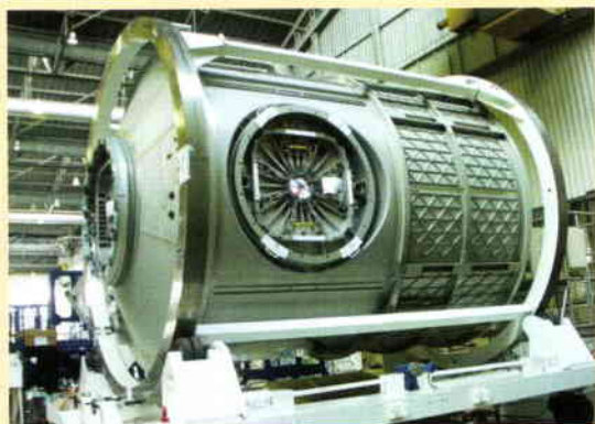
The primary structure of the Node 2 flight unit at Alenia in Turin (I)
