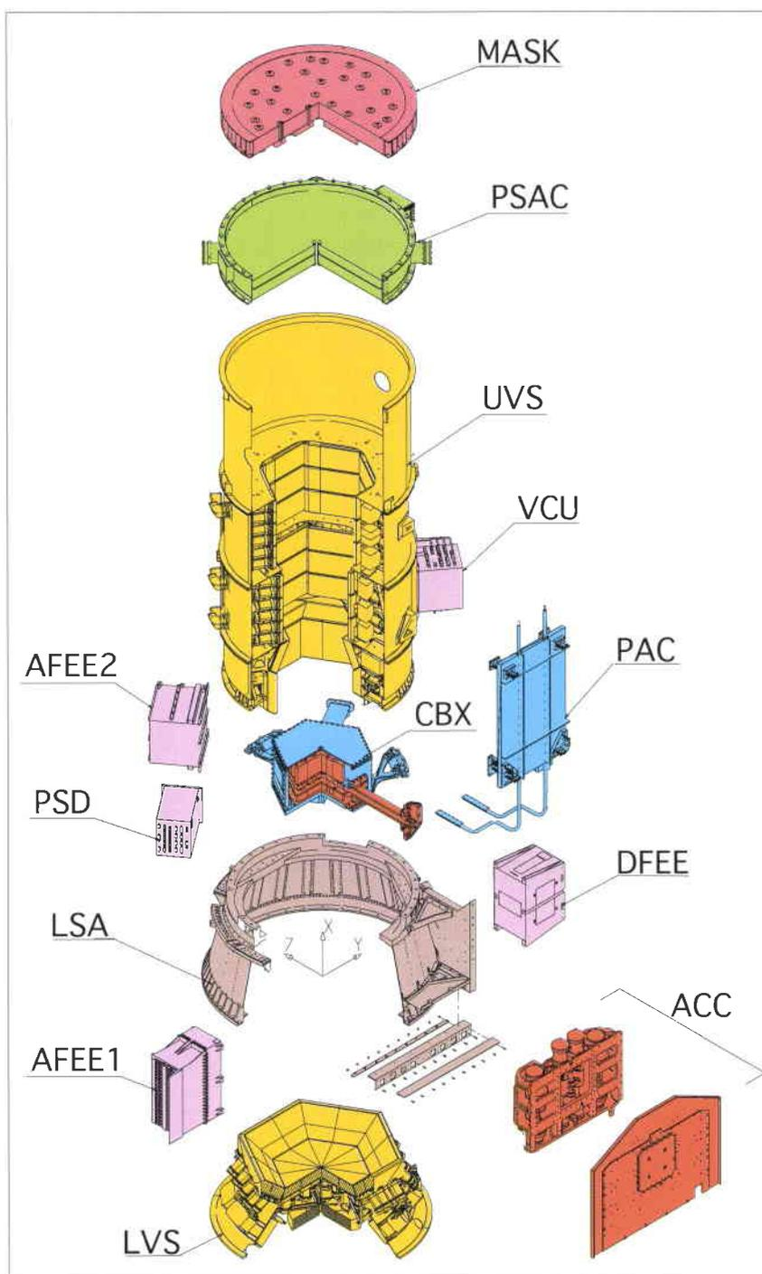
Figure 4. Exploded view of the Spectrometer (SPI), with the core of the instrument, the detector element, housed in a cryostat (courtesy of CNES)
