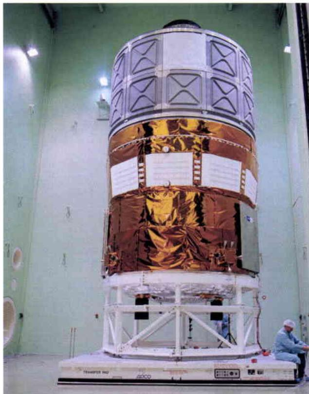
ATV with a total mass of 15 t (low loaded configuration) was mated with the Acoustic Uncoupling Stand (AUS, Fig. 4). This adapter dynamically uncouples ATV from the ground, as well as positioning it inside LEAF's homogeneous acoustic field. Uncoupling was achieved at the top of the adapter through rubber isolator mounting pads. A dry-run test involving the AUS alone was performed a few weeks before the STM test itself.
