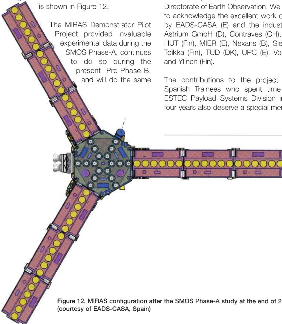
Figure 12. MIRAS configuration after the SMOS Phase-A study at the end of 2001 (courtesy of EADS-CASA, Spain)
