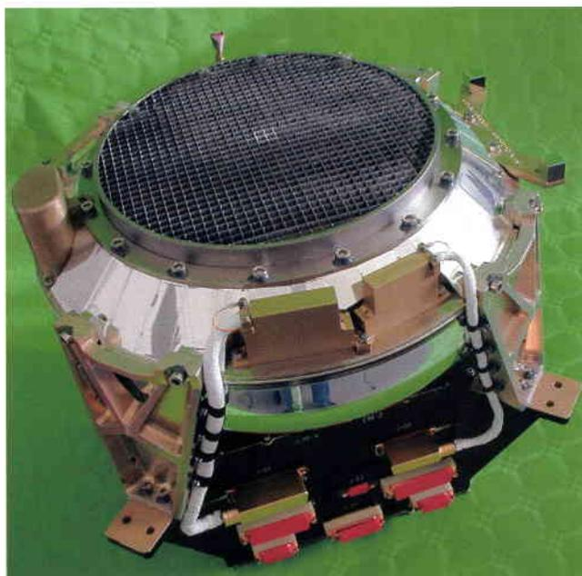
**Figure 10.** The JEM-X detector assembly. The upper element is the detector vessel, whilst the lower, black element is the Digital Front-End Electronics (DFEE). The square pattern of the collimator can be seen on the top of the detector vessel (courtesy of DSRI)
