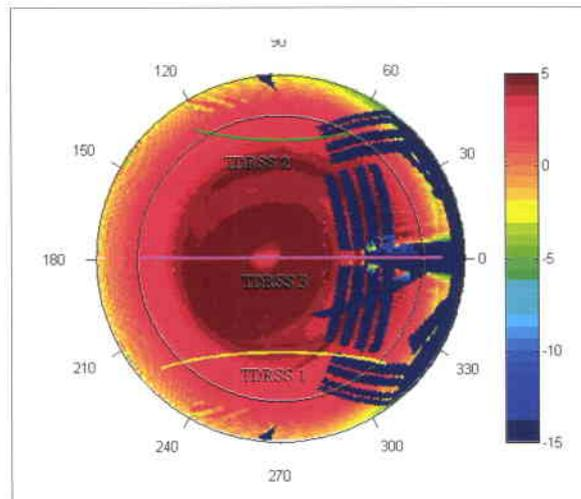
**Figure 10. Radiation of the ATV helix antenna towards the relay satellites, showing the shadow of the ISS. Possible data-relay-satellite trajectories are shown**
