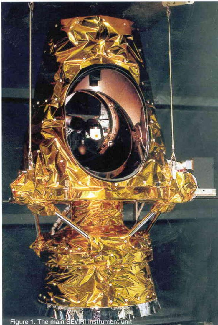
Figure 1. The main SEVIRI instrument unit
