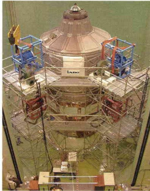
Figure 5. Lateral modal survey test set-up with ATV on MIF
