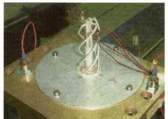
Figure 6. The quadrifilar helix antenna on the ATV
