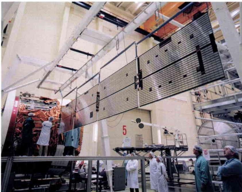
Figure 10. Solar wing under the deployment rig
