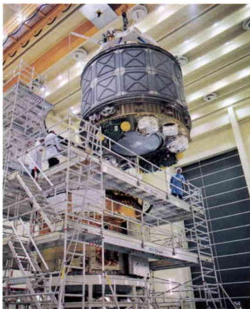
Figure 14. Preparing for the first mechanical integration of ATV
