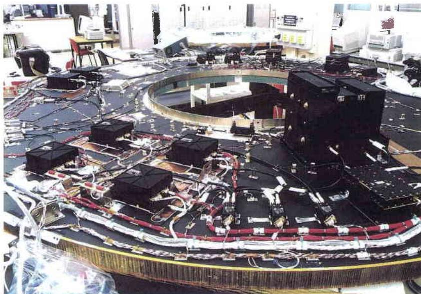
Figure 3. Integration of the first flight-model MCP Transponder
