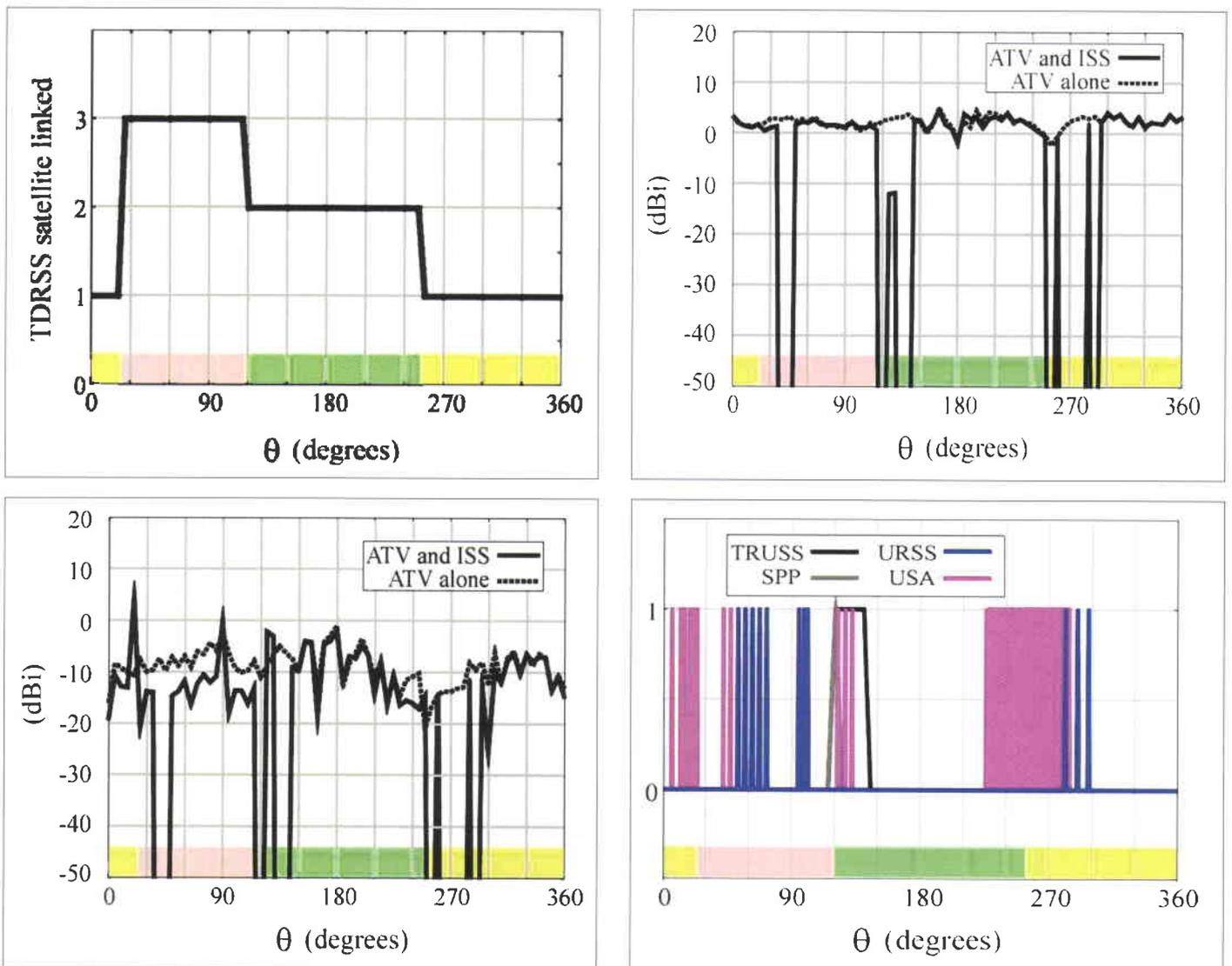
Figure 11. Detailed analysis of the ATV-TDRSS link - the worst-case scenarios for:
