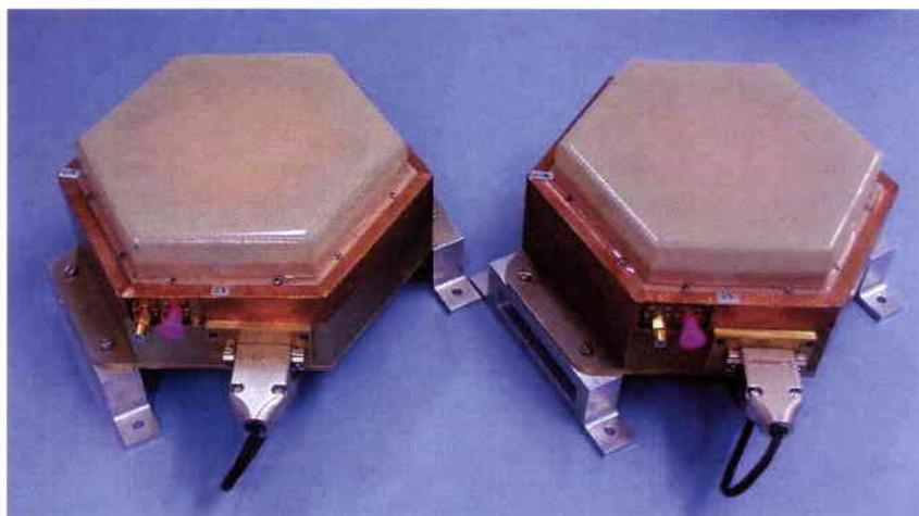
Figure 2. First-generation LICEF-1 antenna-receiver units (courtesy of MIER, Spain)
