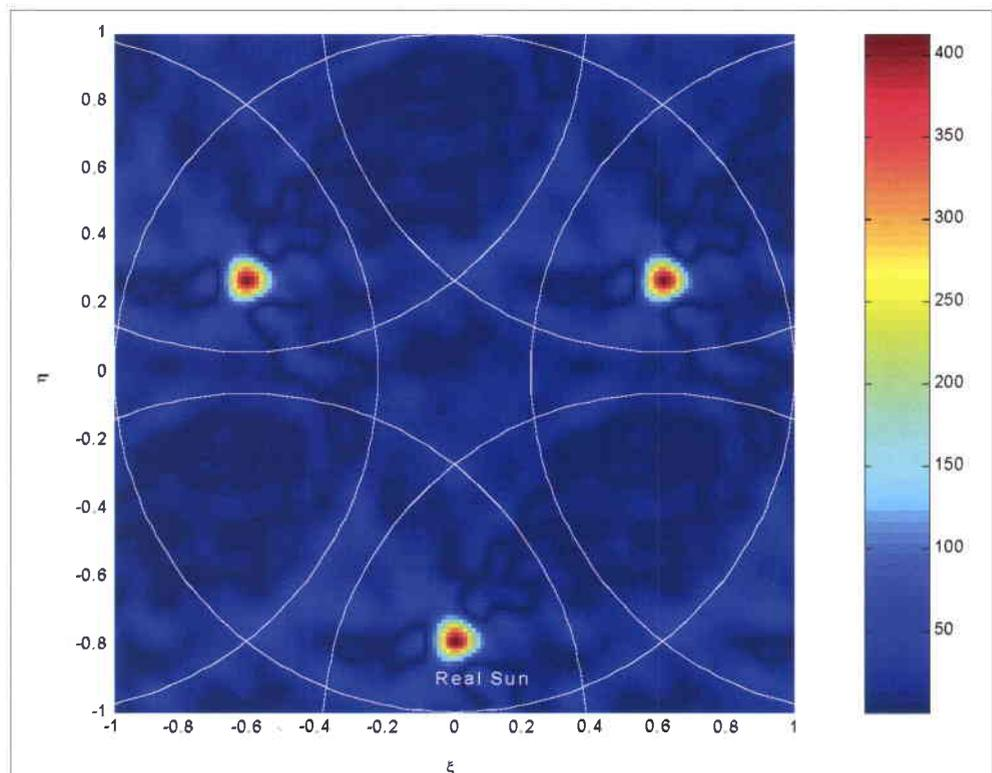
Figure 11. Solar image acquired using the LICEF-1 receivers and the DICOS-3 correlator unit. The real Sun is at 6:00; those at 10:00 and 2:00 are aliases, as expected
