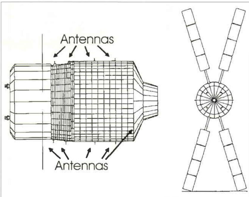
Figure 4. The geometrical modelling of the ATV and its antennas
