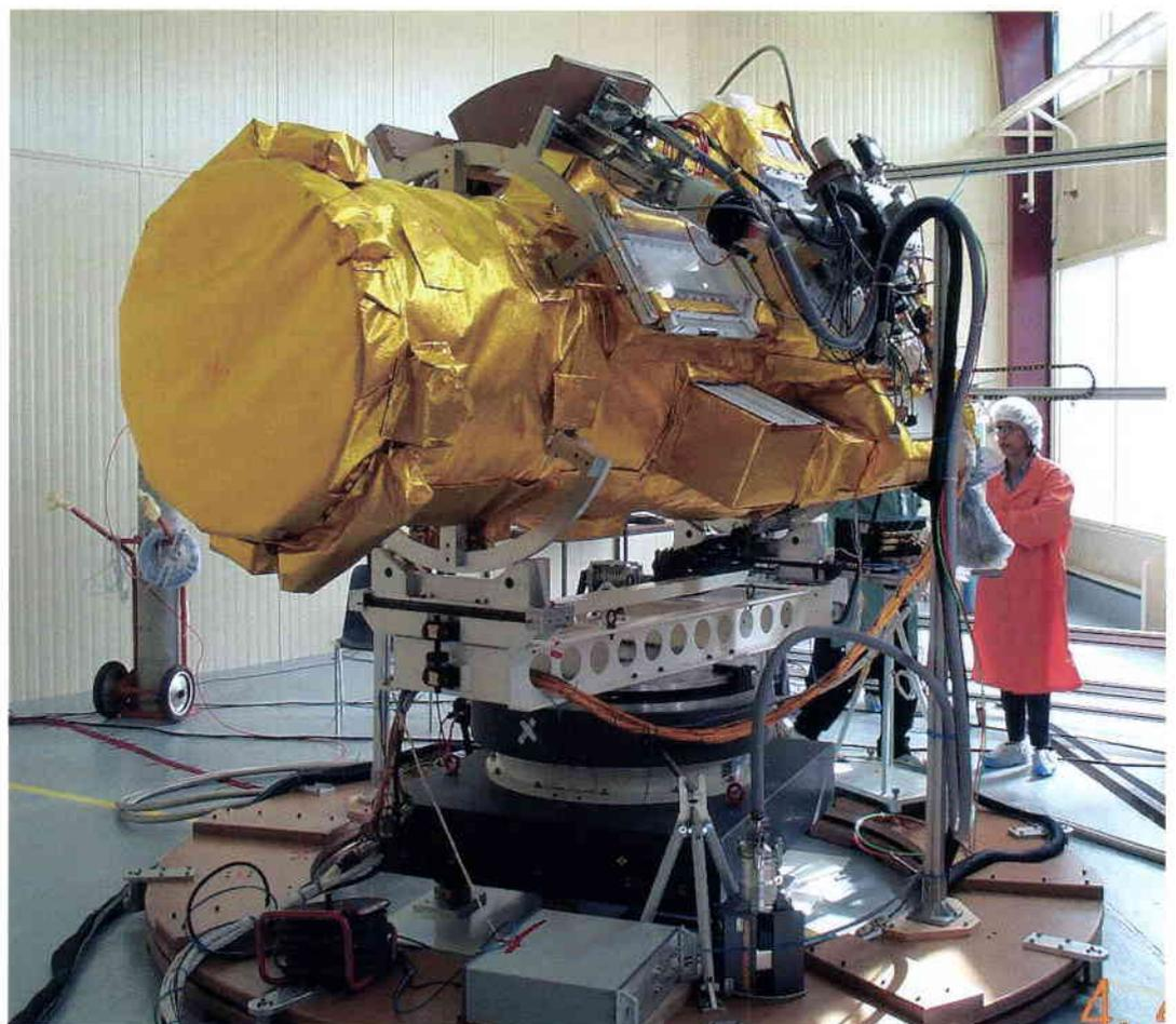
Figure 6. The SPI during calibration activities at the Centre d'Etudes Atomiques in Bruyères le Chatel (F) (courtesy of CESR/CEA/CNES)
