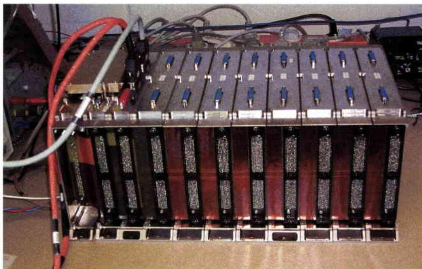
Figure 3. First-generation DICOS-1 digital correlator unit (courtesy of Astrium GmbH, Germany)
