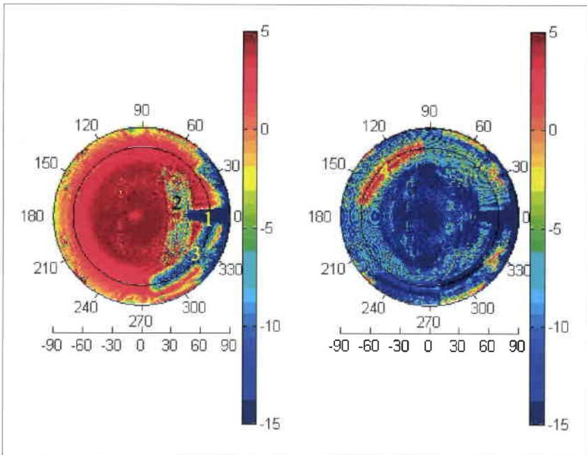
**Figure 8. Representation of the co-polarised (left) and cross-polarised (right) radiation from the helix antenna mounted on the ATV docked on the ISS, with solar panels horizontal**
