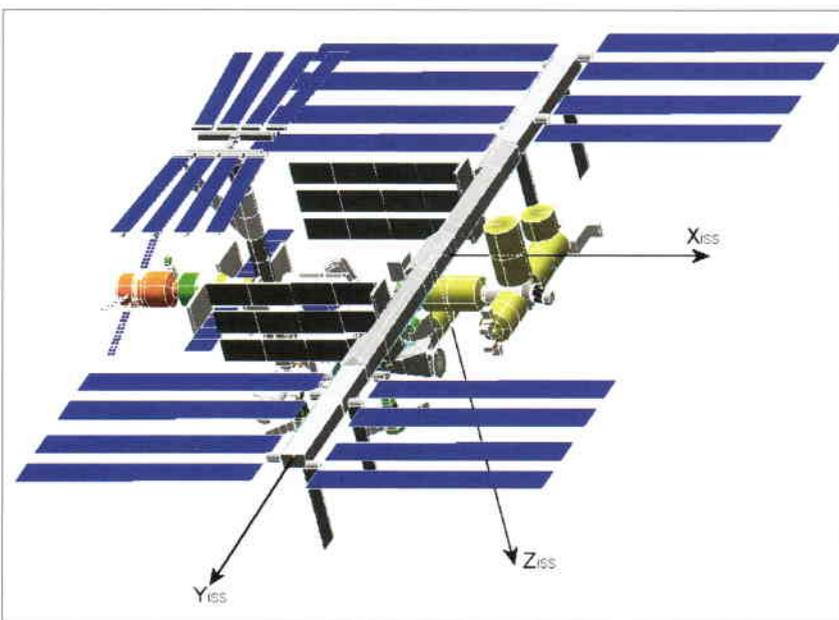
Figure 5. Elements included in the electromagnetic model of the ISS
