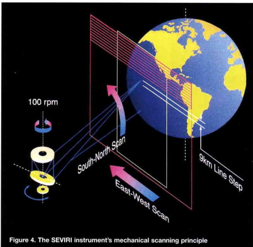
Figure 4. The SEVIRI instrument's mechanical scanning principle
