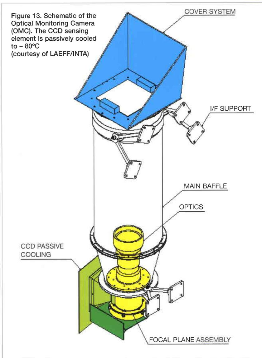
Figure 13. Schematic of the Optical Monitoring Camera (OMC). The CCD sensing element is passively cooled to - 80°C (courtesy of LAEFF/INTA)
