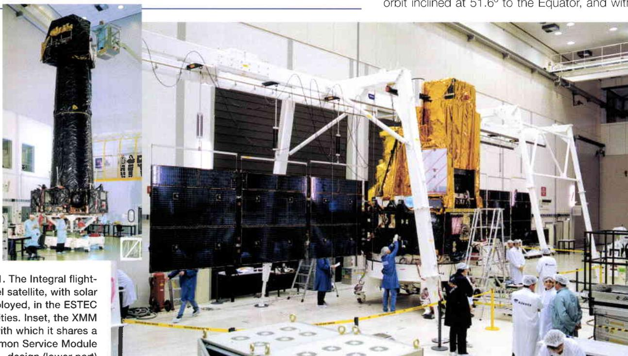
Figure 1. The Integral flight-model satellite, with solar arrays deployed, in the ESTEC test facilities. Inset, the XMM satellite with which it shares a common Service Module design (lower part)
