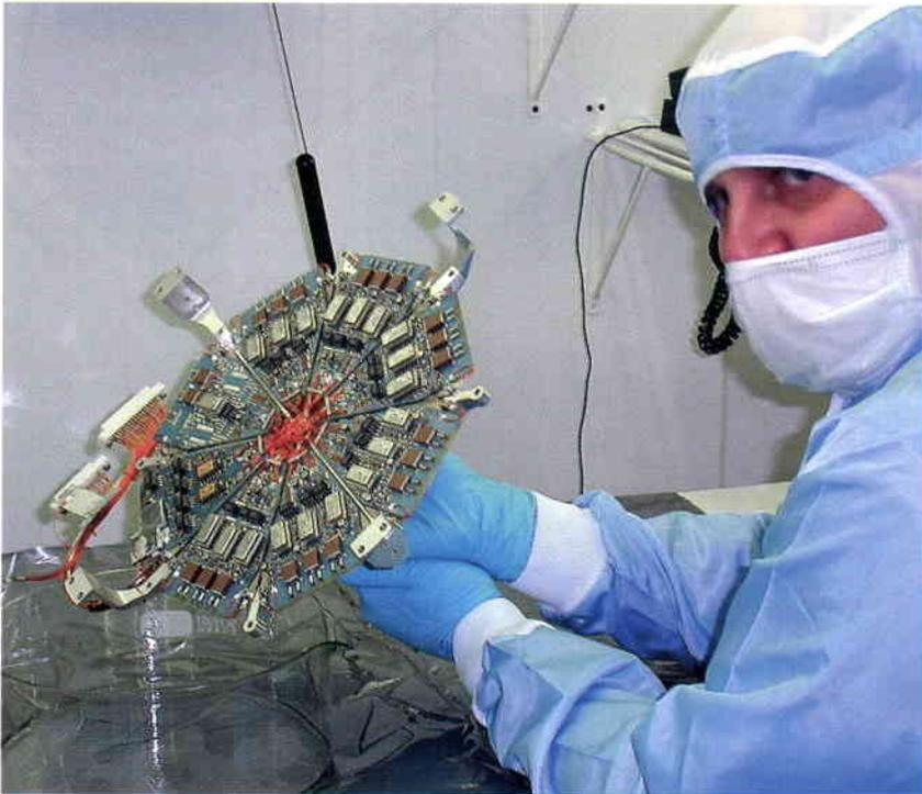
**Figure 12.** The micro-strip plate and its associated electronics are the core elements of the JEM-X detector. Due to their extreme sensitivity to contamination, all assembly operations have been carried out in an extra-clean environment (courtesy of DSRI)
