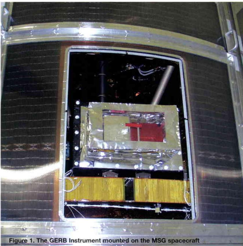
Figure 1. The GERB Instrument mounted on the MSG spacecraft
