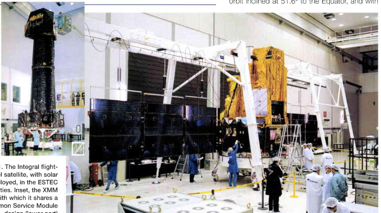
Figure 1. The Integral flight-model satellite, with solar arrays deployed, in the ESTEC test facilities. Inset, the XMM satellite with which it shares a common Service Module design (lower part)
