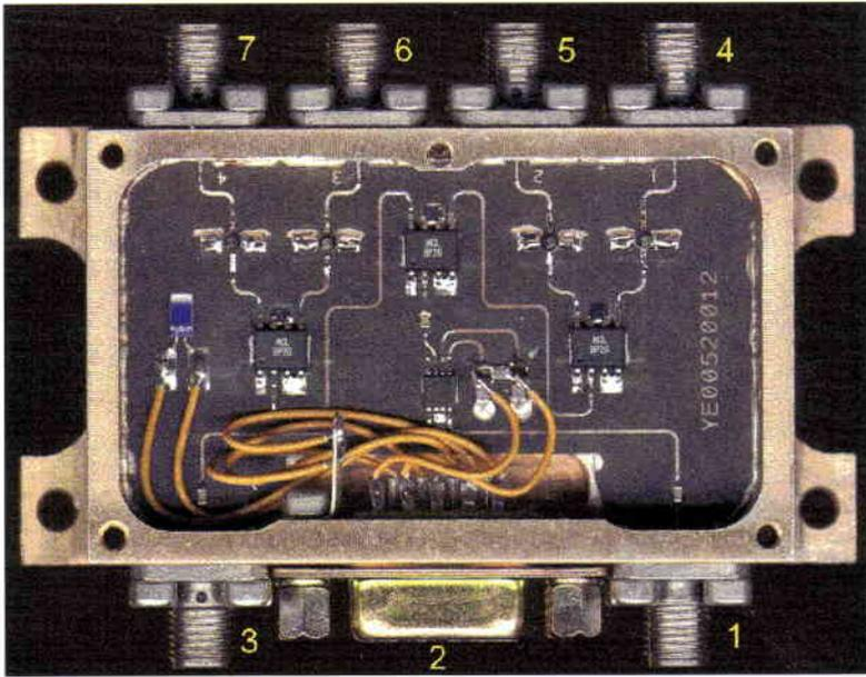
Figure 8. On-board calibration system (CAS) hardware, with the Power-divider (left) and Noise-diode (right) housings (courtesy of Yliinen, Finland)
