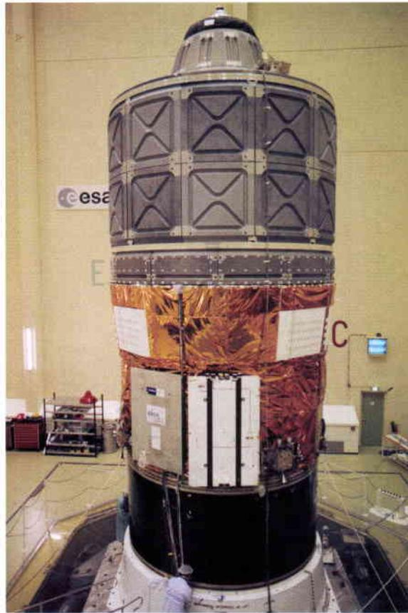
Figure 8. ATV (with SDM) modal tests on HYDRA
