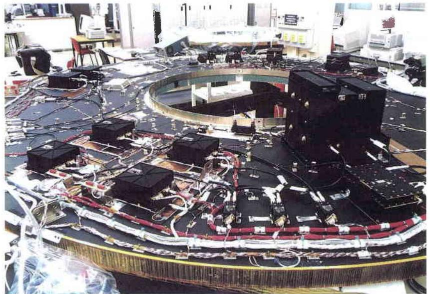
Figure 3. Integration of the first flight-model MCP Transponder
