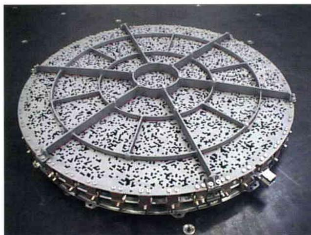
**Figure 11.** The JEM-X mask is made from a thin tungsten plate. The coded pattern is provided by a regular combination of small hexagonal holes. Supporting ribs are provided to carry the launch loads (courtesy of Univ. of Valencia/Sener)
