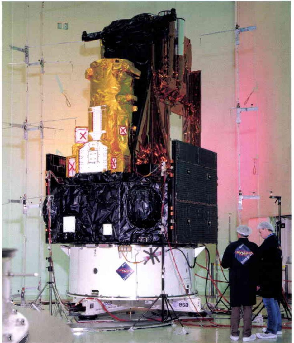
Figure 4. Integral in the Acoustic Test Facility at ESTEC
