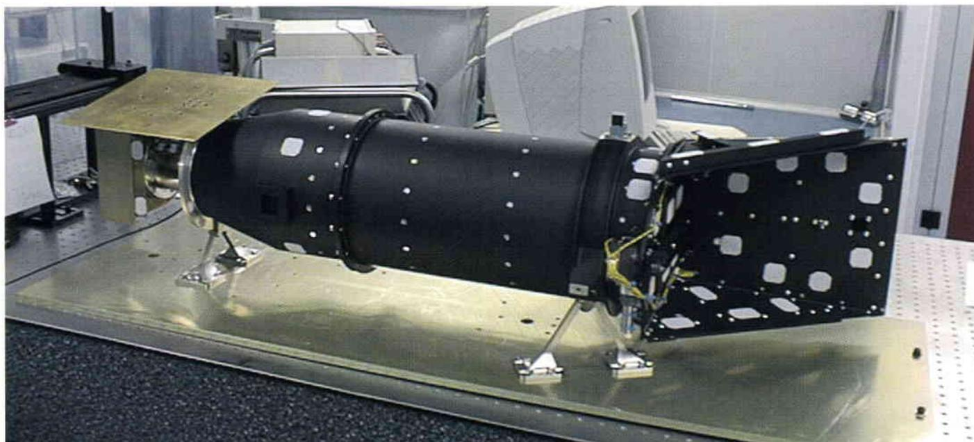
Figure 15. The OMC focal-plane assembly, showing the CCD at the top (courtesy of LAEFF/INTA)
