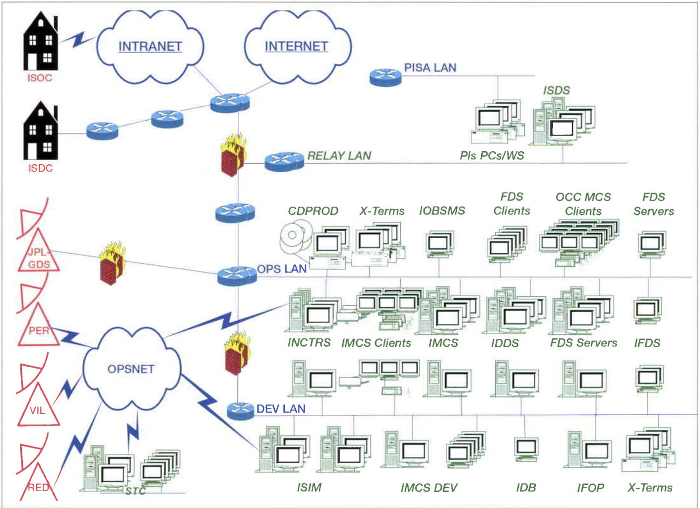
**Figure 3. The Integral Mission Operations Centre computer-system configuration**
