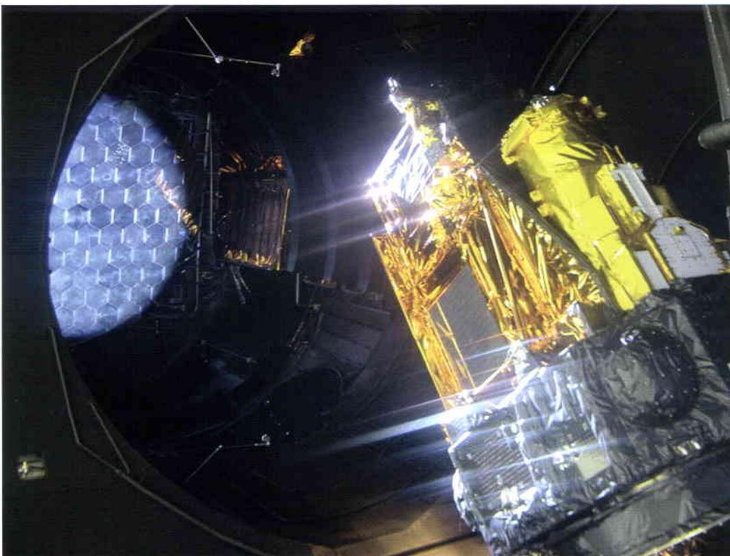
Figure 5. Integral in ESTEC's Large Space Simulator (LSS) for thermal-vacuum testing
