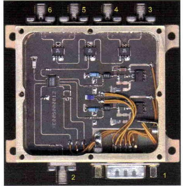
Figure 9 shows the Serial Optical Transmitter Receiver (SOTR) unit.
