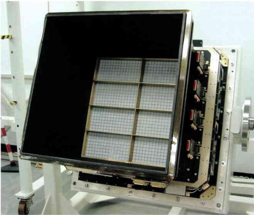
**Figure 8.** The IBIS detector unit. The eight modules of the upper detector layer can be seen at the bottom of the collimator. Each module is made up of 2048 sensing elements. (courtesy of CNR-IAS/CEA and Laben)
