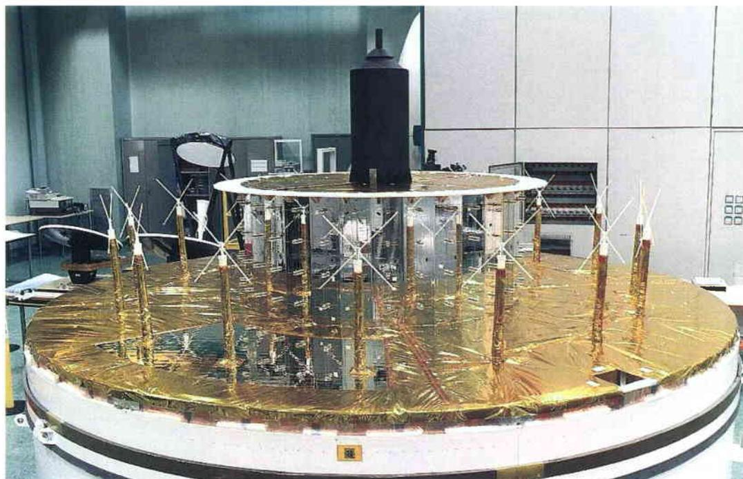
Figure 1. The flight-model MCP Antenna Subsystem
