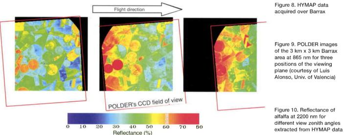
The different aspects of the three images are due to the different view-target-Sun configurations (the Sun is located to the bottom-right of the images). The image sequence shows the hot spot, characterised by a sharp increase in surface directional reflectance when illumination and viewing geometry are in coincidence. The processing of all images acquired during the flight permits the full BRDF of every 20 m pixel of the area to be reconstructed.
