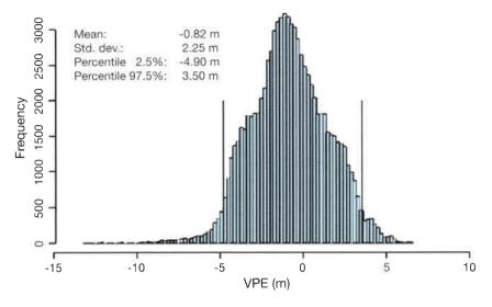
Figure 7. Typical ESTB vertical-error histogram
