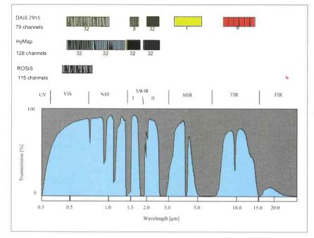
The complementary nature of the various instruments is illustrated in Figure 5, which shows their different spectral layouts in the context of atmospheric transmission.
