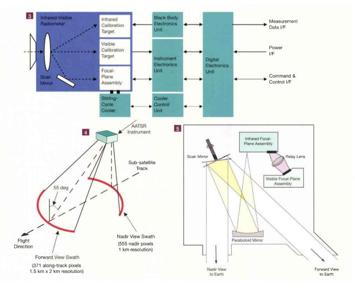
an angle close to vertical (the nadir view) as the satellite moves forward. These observations are separated in time by 150 sec, or approximately 1000 km on the ground, at the sub-satellite point.
