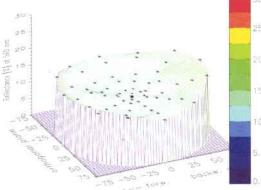
Anisotropic effects can be assessed via the experimental Bidirectional Reflectance Factor (BRF), which is the ratio of the directionally reflected radiance from the surface target and the nadir radiance of a Lambertian-scattering reference target. The Bidirectional Reflectance Distribution Function (BRDF) describes the angular behaviour of the surfaces, and it can be assessed by measuring the BRF.
