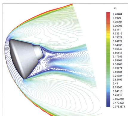
Figure 3. ARD oil flow patterns in the ONERA S4 facility at Mach 10 (incidence angle 20 deg) and the corresponding computed skin friction lines
