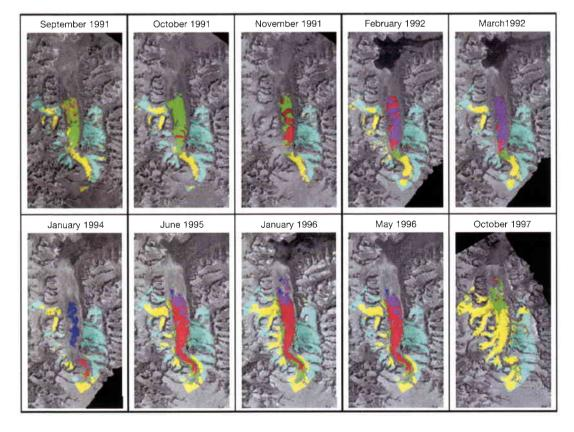
Figure 12. Temporal sequence of geocoded displacement maps of a glacier in Svalbard (24 km x 45 km). The magnitude d (in m/day) of the threedimensional displacement rate is shown with the following colour scale: d < 0.1 cyan, 0.1 < d < 0.4 yellow, 0.4 < d < 0.7 green, 0.7 < d < 1 red, 1< d < 1.3 violet, d > 1.3 blue (courtesy Univ. of Wales, Gamma Remote Sensing, Univ. of Leeds)
