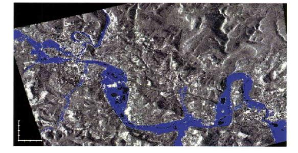
Figure 10. Flood-extension map of a portion of the River Meuse (F), which was subject to flooding in 1993/94 (blue) and 1995 (cyan). The map was generated from a multitemporal combination of ERS SAR images (courtesy of SERTIT)
