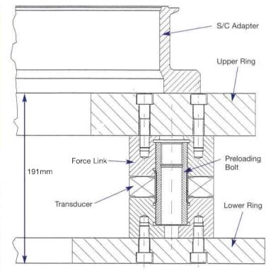
an acceptance test, which also provided the opportunity to verify the good functioning of the FMD. The test set-up consisted of the sliptable, FMD, load spreader, and a 2085 kg dummy specimen. The aim with the load spreader was to increase the load capability of the slip-table. The interface forces and moments were measured with the FMD, as well as computed.
