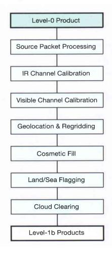
Figure 8. The AATSR Level-1b processing steps
