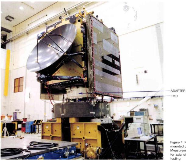
Figure 4. Rosetta STM mounted on the Force Measurement Device (FMD) for axial sine vibration
