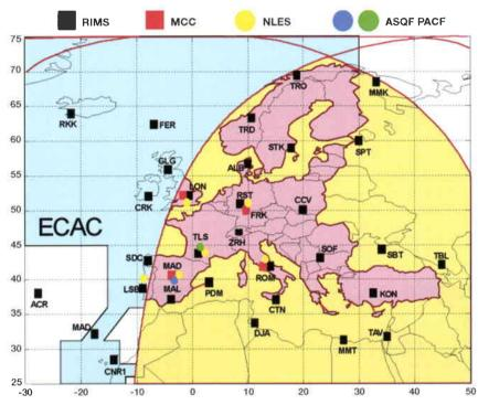
Figure 4. Planned sites for the various EGNOS Ground Segment elements
