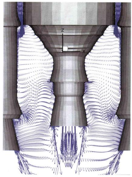
Figure 9. Predicted unsteady velocity vectors in the base region of the Ariane-5 model at Mach  $0.7\,$
