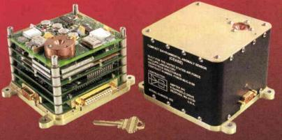
**CEASE** is a compact, radiation hard, low power, space "weather" hazard sensor developed to monitor the local radiation environment and to provide autonomous real-time warnings of:
