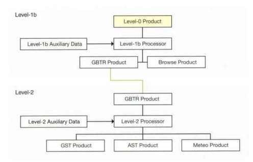
Figure 7. Relationship between the AATSR products and processing levels Figure 7 summarises the relationship between the AATSR products and processing levels.
