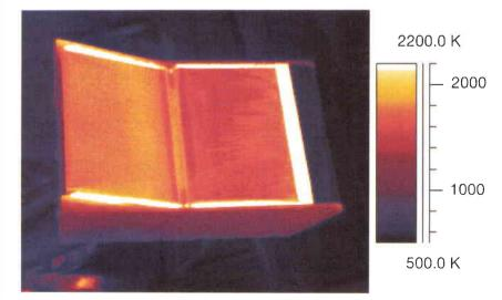
Figure 7. Surface-temperature distributions in the TETRA X-38 body-flap model with closed and open gaps in the L3K facility at DLR in Cologne
