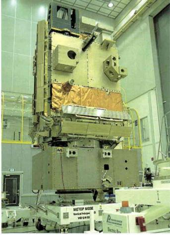
The MSG-1 SEVIRI optical instrument during integration at Astrium in Toulouse (F)
