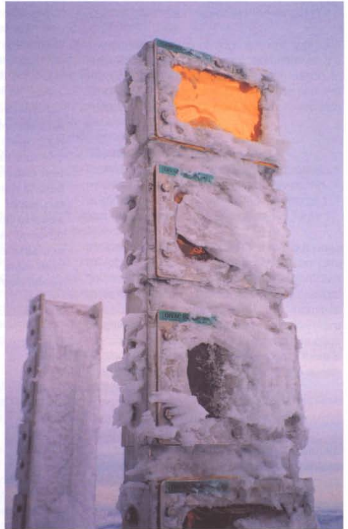
Figure 10. The test panels partially cleared of rime ice (right)
