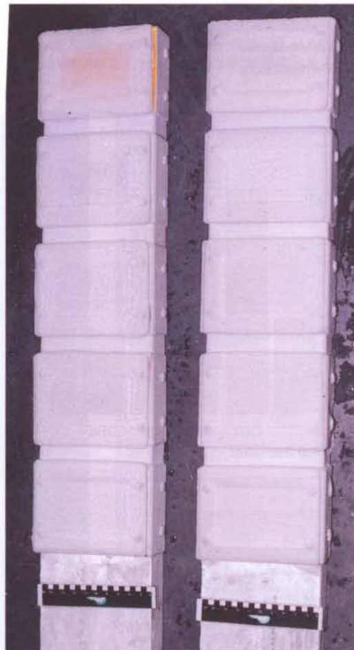
Figure 5. Advanced materials with ice-phobic properties subjected to ice (left and below) and snow (right) accretions in the laboratory
