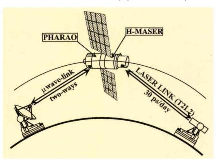
Figure 4. The ACES concept; Pharao is the laser-controlled atomic clock and the hydrogen maser serves as the reference clock
