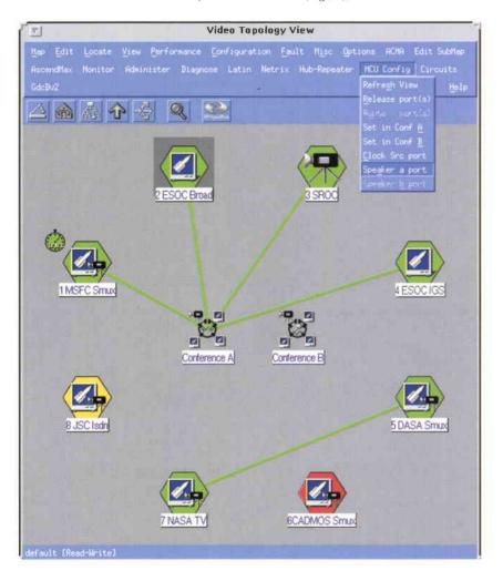
Figure 7. Video Service Management view The device can establish two-party conferences in which both connected codec devices receive signals from each other, It also supports up to two multi-party conferences ('A' and 'B'), represented by the two central icons,
