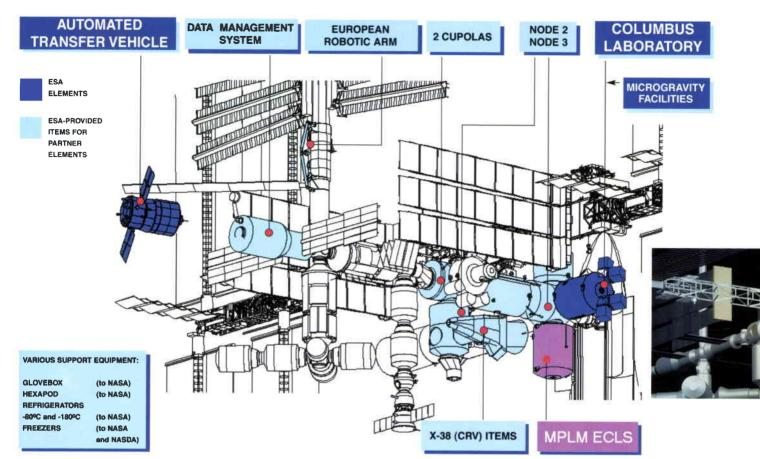
ESA's contributions to the ISS. MPLM is highlighted in pink; the other ESA-provided items for Partner elements are in light blue. Right: MPLM remains berthed only while the Space Shuttle is docked to the Space Station – the spaceplane is omitted here for clarity. (ESA/Alenia Aerospazio)
