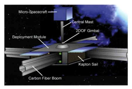
Figure 5. Sailcraft baseline concept, partially deployed
