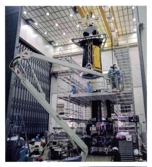
(top) Infinite precaution is taken during the mating of the upper and lower halves of ESA's X-ray astronomy satellite, XMM, at ESTEC (middle) The two halves are sealed by 64 bolts around the 6 m diameter interface plane (bottom) To mark this new milestone, the first of the 64 bolts, specially made of gold, is inserted by Dr Hubert Hofmann (right) of Dornier Satellitensysteme, assisted by Robert Lainé, ESA's XMM Project Manager
