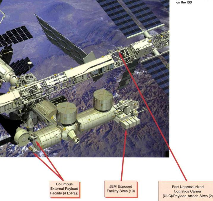
Figure 1. Locations for attaching external payloads on the ISS The ISS offers a choice of several external sites for mounting payloads to be exposed to the surrounding space environment:
