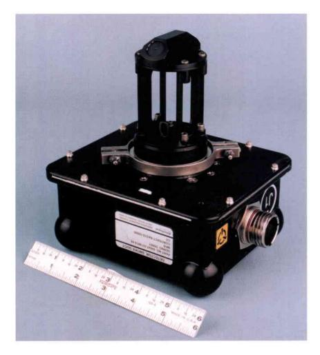
A single Duct Smoke Detector (DSD) on a cabin air duct alerts the MPLM data management system if it detects smoke the carbon dioxide from a single extinguisher would reduce the oxygen concentration in any one below the minimum (10,5% by volume) necessary for sustaining a fire,
