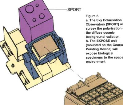
0 00 **Observatory (SPORT) will** survey the polarisation of (mounted on the Coarse specimens to the space
