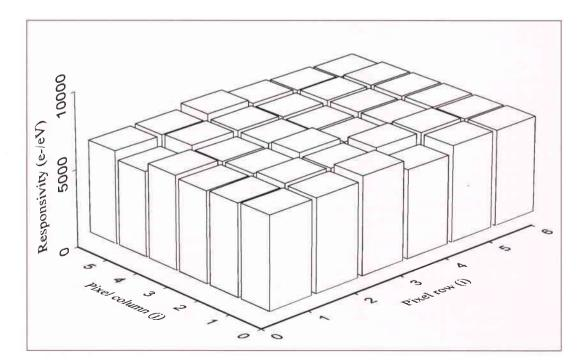
Figure 2. Mapping of the array's responsivity (36 elements)
