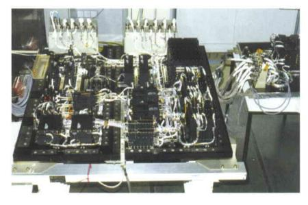
Figure 6. RA-2 flight-model panel after the completion of its acceptance test programme
