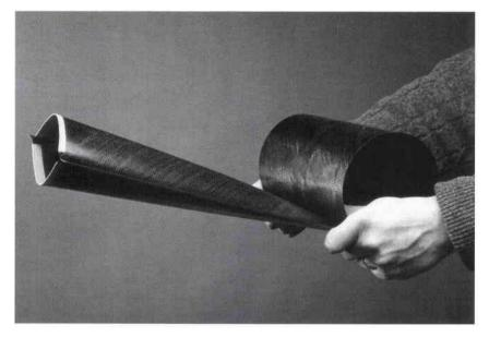
Figure 6. A CFRP deployable boom
