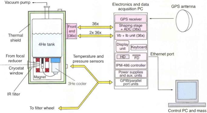
Figure 4. S-Cam block diagram: cryostat, front-end and data-acquisition electronics
