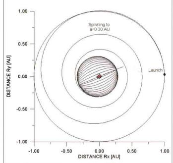
Figure 3. A solar-sail 'dual solar photonic assist' transfer to Pluto
