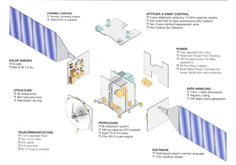
cylindrical element is the Launch Vehicle Adapter. The remaining structural items are principally flat, standard panels with aluminium skins and aluminium honeycomb.
