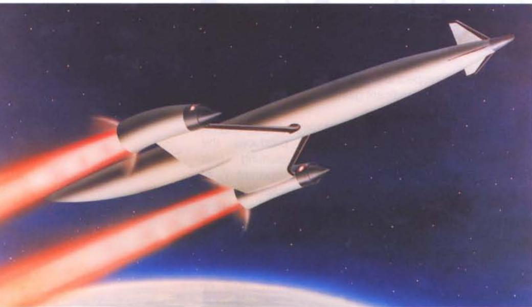
**Figure 2. A possible single-stage-to-orbit launcher with combined air-breathing and rocket propulsion**
