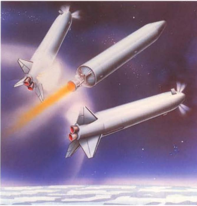
In the DRL mode, the first stage provides a larger share of the total  $\Delta V$  and is allowed to land down-range of the launch site after separation and re-entry. The first stage returns to the launch site at a later time. The TARANIS, studied by Aerospatiale for ESA in the early 1990s (Fig. 7) was this type of vehicle.
