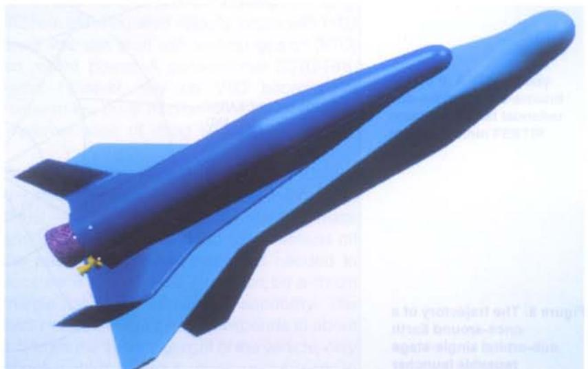
Figure 7. TAKANIS: a fully reusable rocket launcher with down-range landing of the first stage
