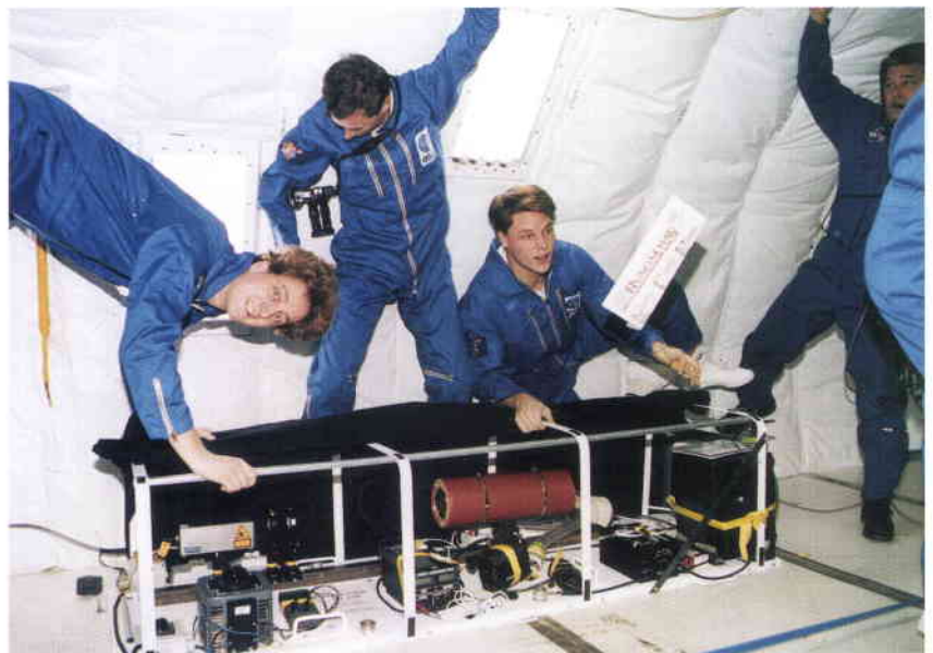
Figure 2. Students from Austria attempt to produce a large air lens inside a hot tube and observe it with a laser
