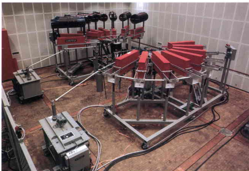
Figure 2. The lightning current simulator with its two impulse current generators
