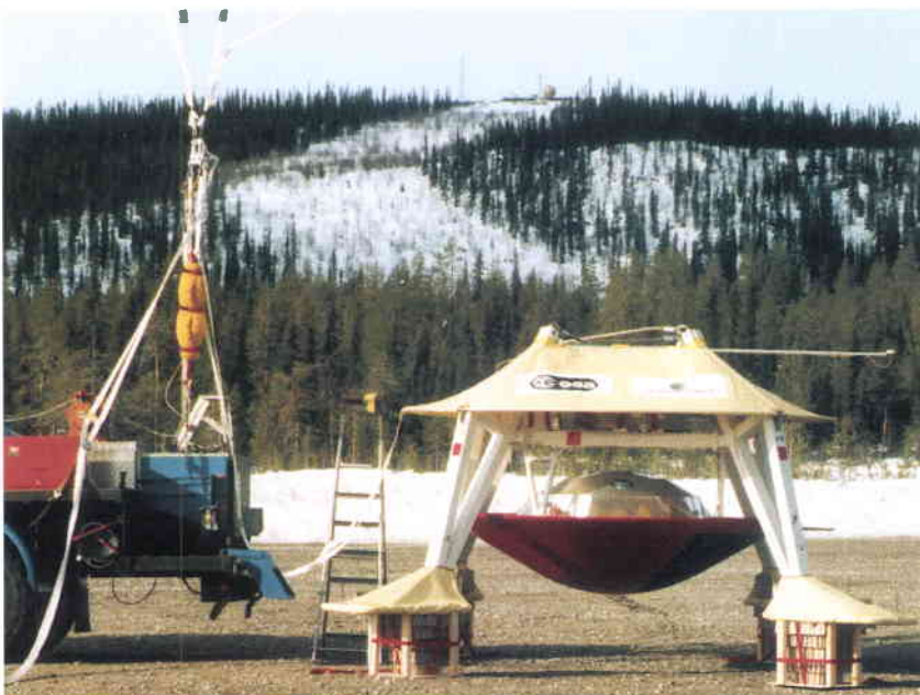
Figure 2. The Huygens Probe and gondola assembly prior to suspension from the auxiliary balloon
