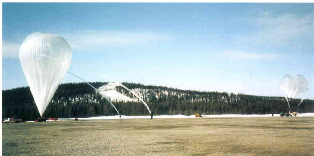
Figure 3. Auxiliary and main-balloon filling on the 'launch pad'
