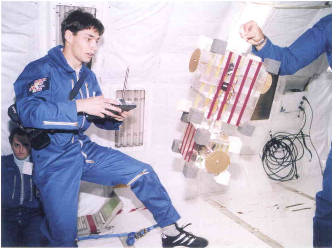
Figure 4. Students from Delft practise rotating an artificial 'cat' in weightlessness, by remotely controlling its feet and body
