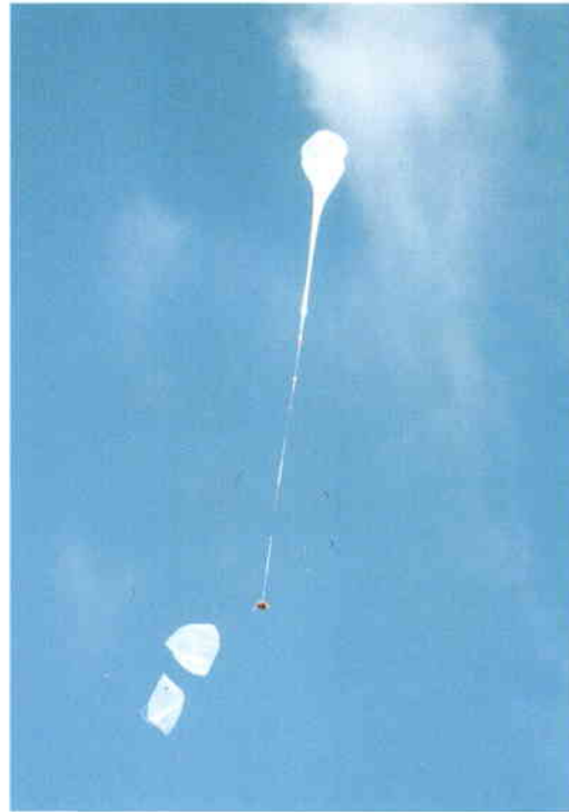
Figure 4. Probe/gondola ascent at the moment of auxiliary balloon release
