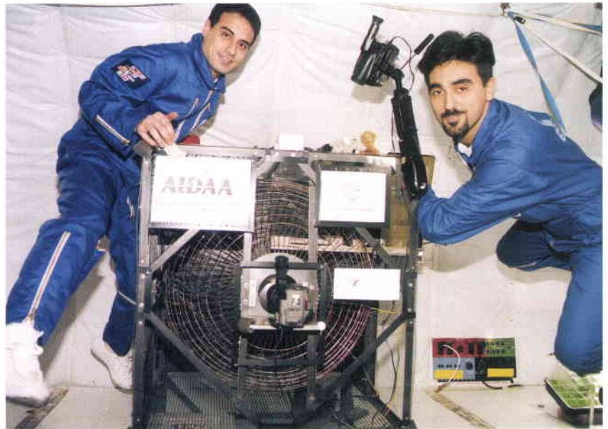
Figure 1. Two Italian students perform an orbit simulation using a small mass attracted by the high electrical potential of a central sphere
