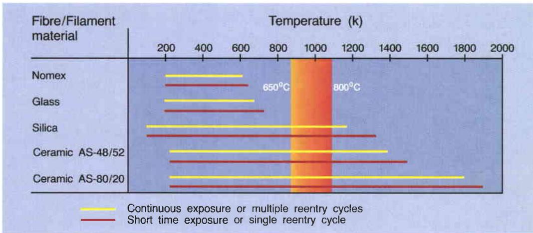
Figure 5. Material/ component selection guide
