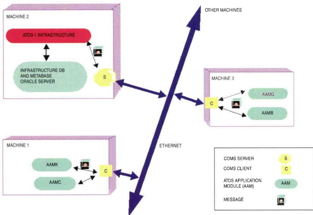
**Figure 6. Physical architecture of ATOS-1**
