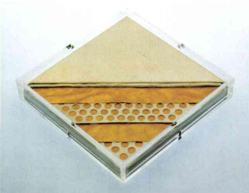
Figure 15. High-temperature multilayer insulation demonstration sample
