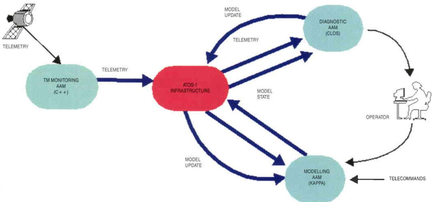
**Figure 7. Architecture of AMFESYS, a prototype with three AAMs built to demonstrate the viability of a modelling approach to spacecraft control**
