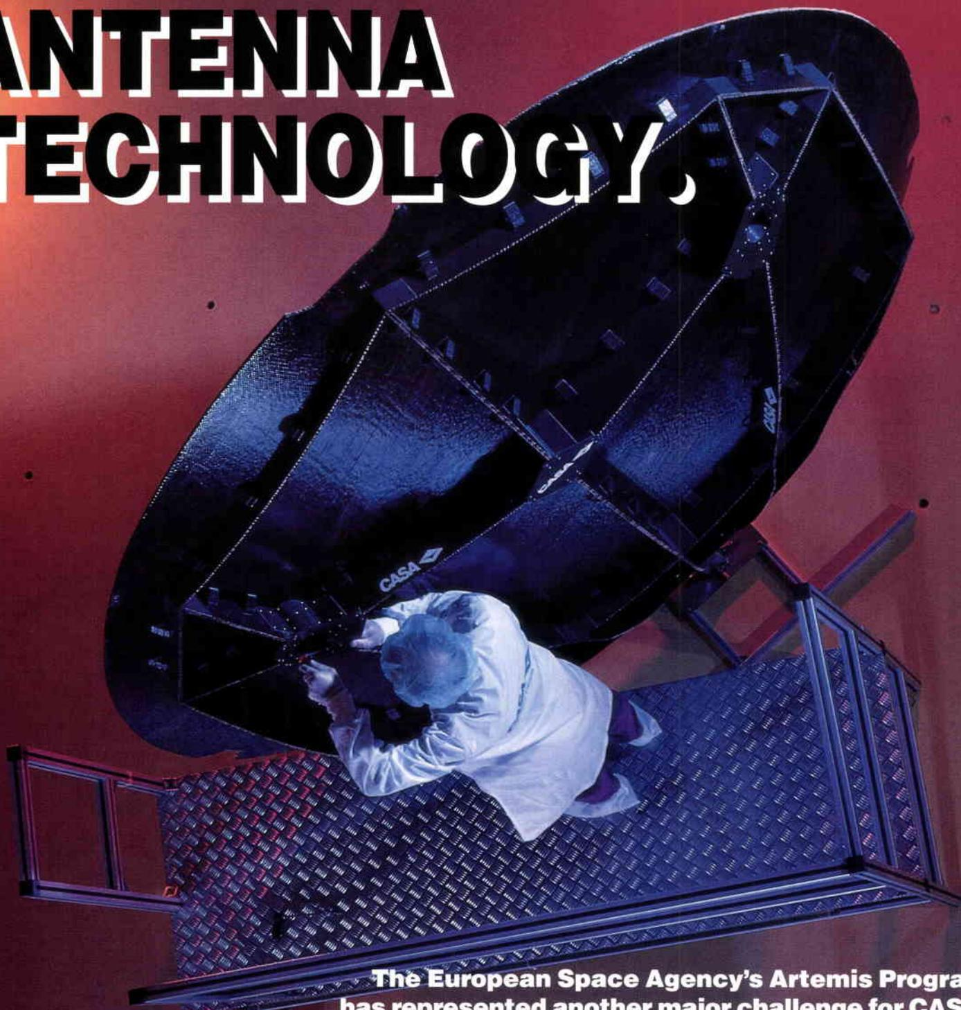
**The European Space Agency's Artemis Program has represented another major challenge for CASA. CASA is developing the Common Large Reflector Dish for communications links between Artemis, other Leo users and Earth. The 2.8 x 3.3 meters Antenna Reflector is designed with the latest CFRP technology, achieving a very low level of Thermal Distortions. Yet another good reason why CASA is the best choice for light structures with high-dimensional stability in space.**
