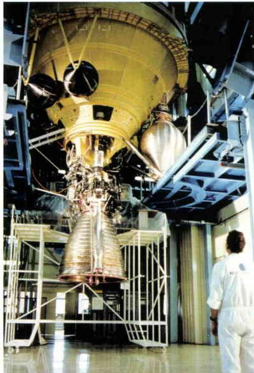
**Figure 6. The cryogenic stage's upper skirt during a static test**
