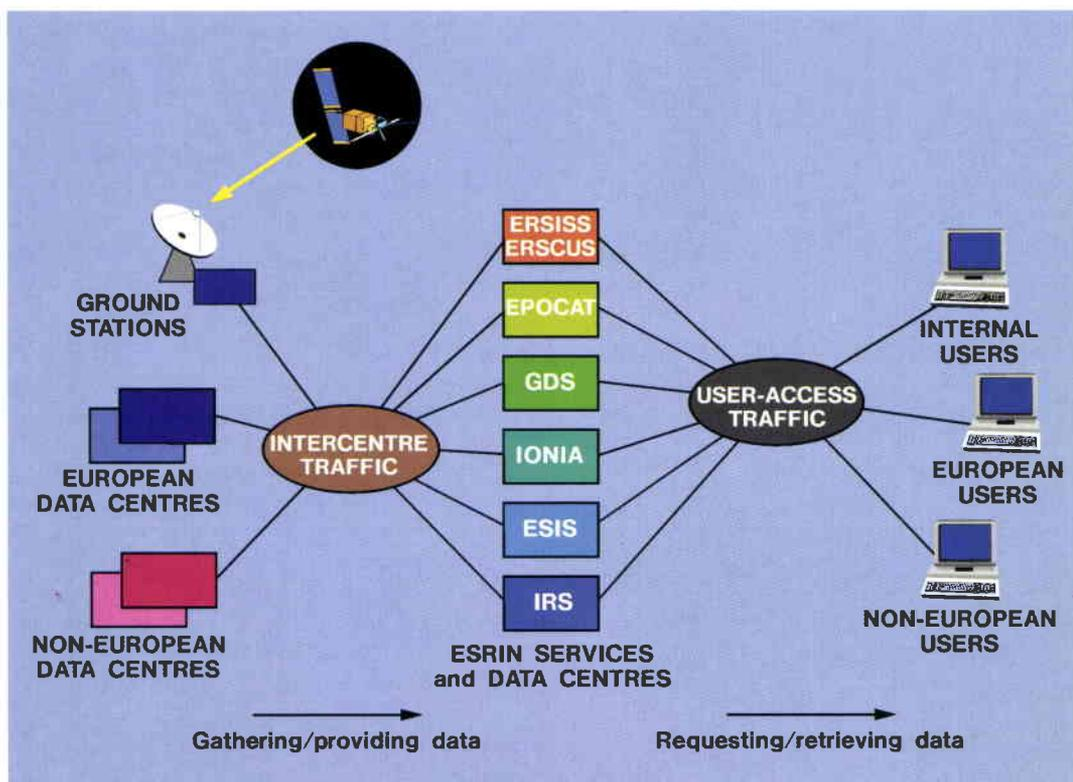
Figure 1. The Data Dissemination Network (DDN) via which ESRIN's services are made available on-line to users around the world
