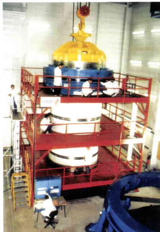
**Figure 2. Preparing for the testing of the booster joints**
