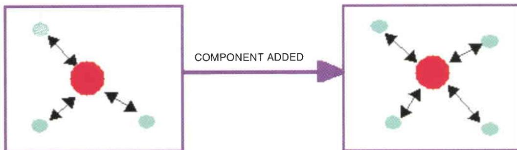
**Figure 2. Client-server communication between software components. The addition of a new component means that only the interface with the new component must be provided.**
