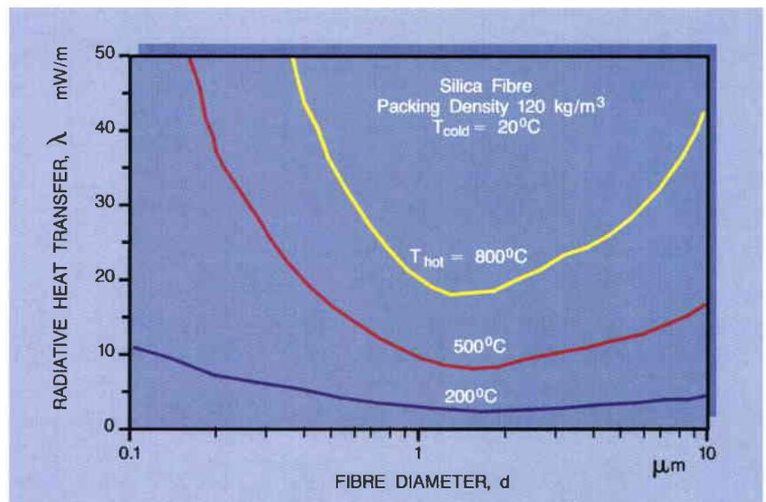
Figure 6. Mass-related resistance to heat radiation as a function of the diameter of the fibres used for the blanket's core
