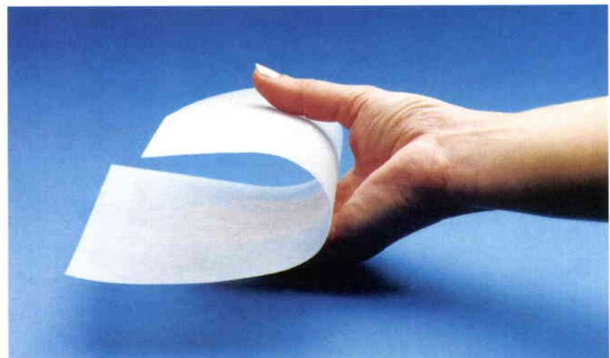
Figure 12. The ceramic substrate foil after firing
