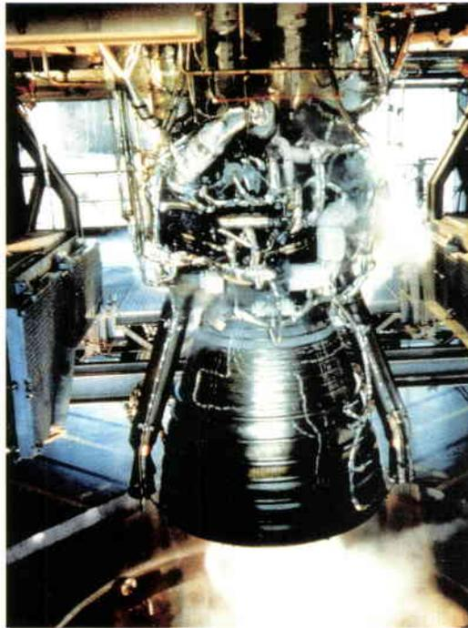
**Figure 5. The Vulcain engine during a firing test**
