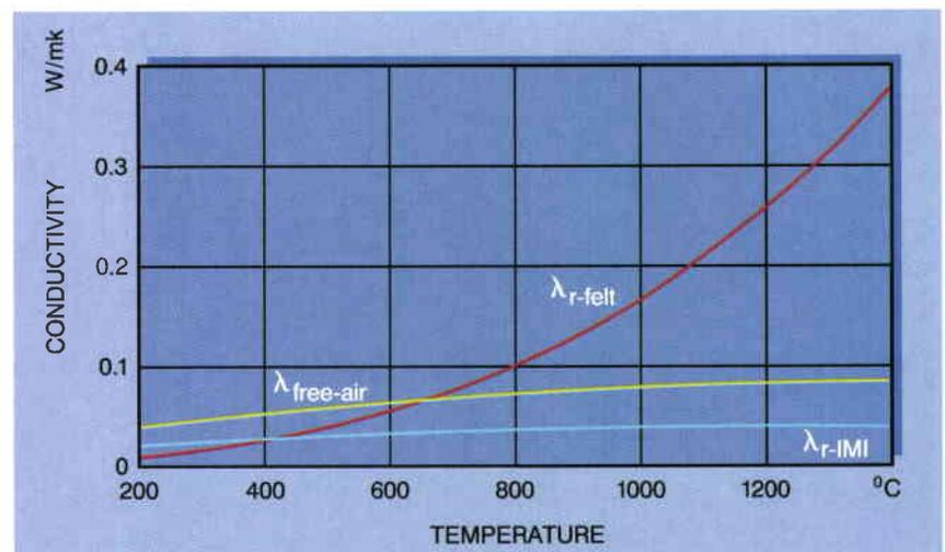
Figure 11. Conductivities of felt- and IMI-type insulations as a function of temperature
