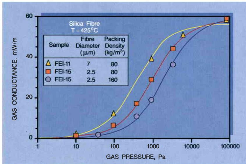
Figure 7. Gas conductance as a function of pressure
