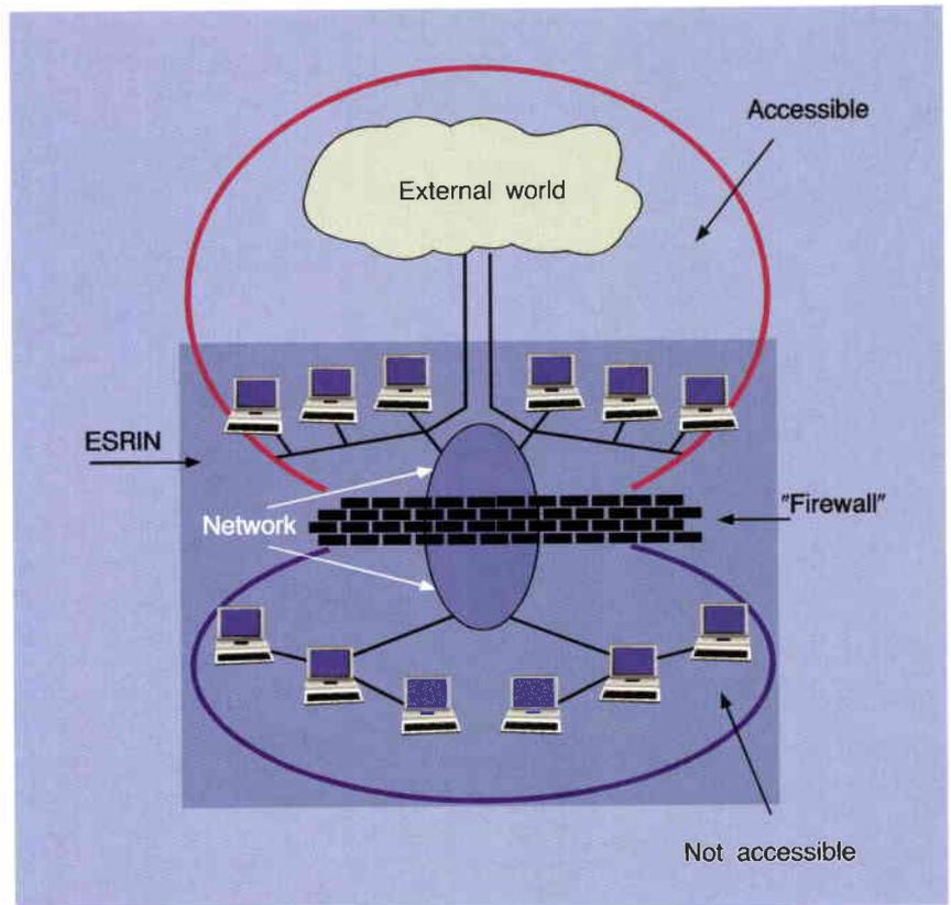
Figure 3. A logical 'firewall' separates ESRIN's systems and services that do not have to be accessible to the external world from those that must be accessible
