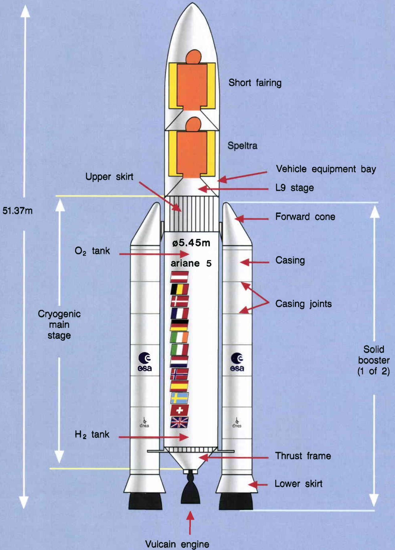
Figure 1. The components of the Ariane-5 launcher
