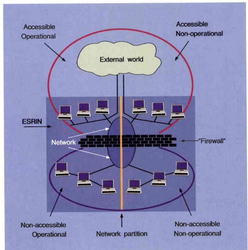
Figure 4. Four categories of network have been created. All host computers offering an operational service, whether they are accessible or non-accessible, are connected to different networks than those used for development or office support (non-operational)
