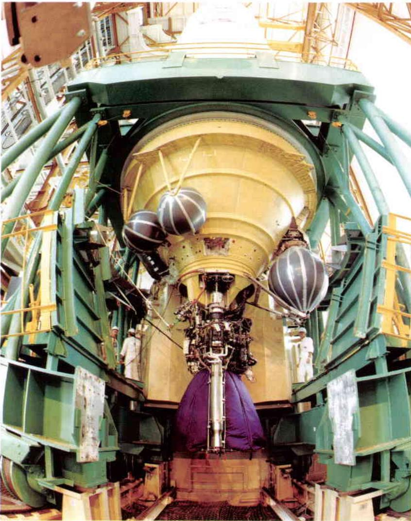
**Figure 6. The 'battleship' version of the cryogenic main stage being assembled in the Launcher Integration Building. This reinforced stage will be rolled out to the launch pad for static hot firing tests ('battleship test campaign')**
