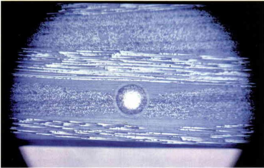
**Figure 3. Optical fibres embedded in a woven CFRP skin**
