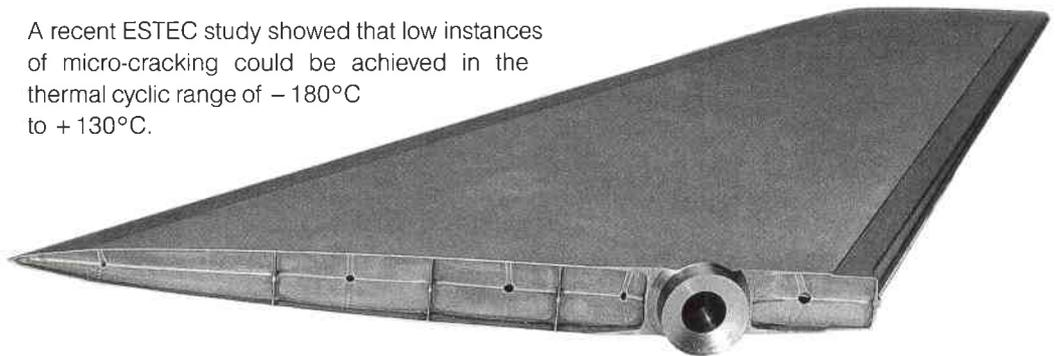
**Figure 1. Extensive use of diffusion bonding and superplastic forming is made in the manufacture of the Rafale fighter's highly loaded titanium canard. This incorporates a diffusion-bonded spigot and a hexagonal corrugated core structure. A substantial mass saving is realised compared with other manufacturing methods (Photo courtesy of Dassault Aviation)**
