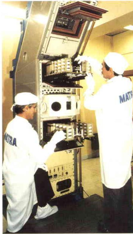
*The Biorack, with two incubator drawers and the cooler/freezer (top) open*
