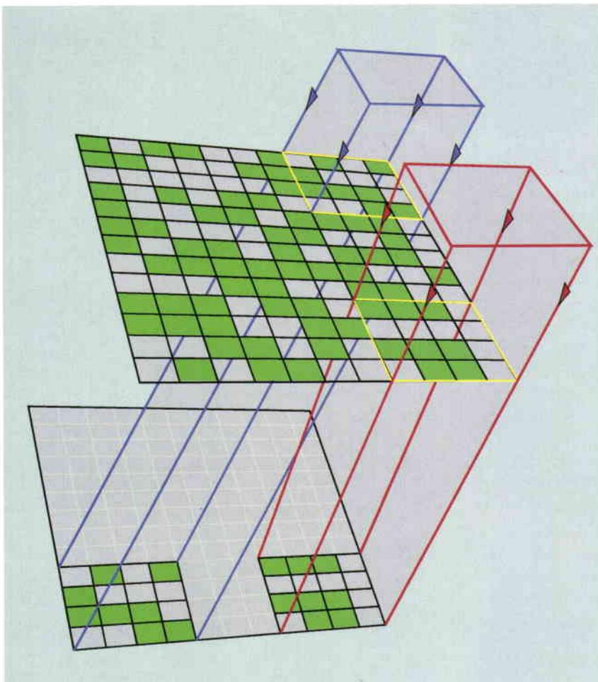
region of the sky, the difference is taken between the signal in all those detector elements that have a clear view of a source at the position under consideration, and that from detector elements for which the source is obscured by opaque regions of the mask. Thus, the detector background is measured exactly contemporaneously, using a subset of the detector elements intermingled with those observing the source.
