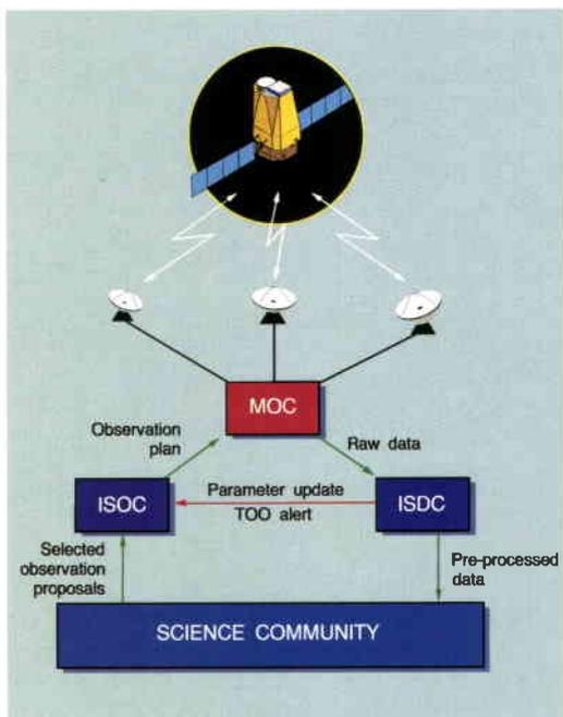
Figure 7. The Integral ground segment
