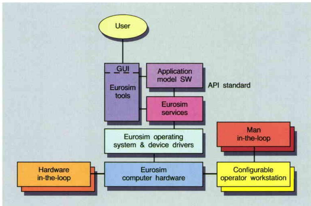
Figure 2. Layout of the Eurosim simulator
