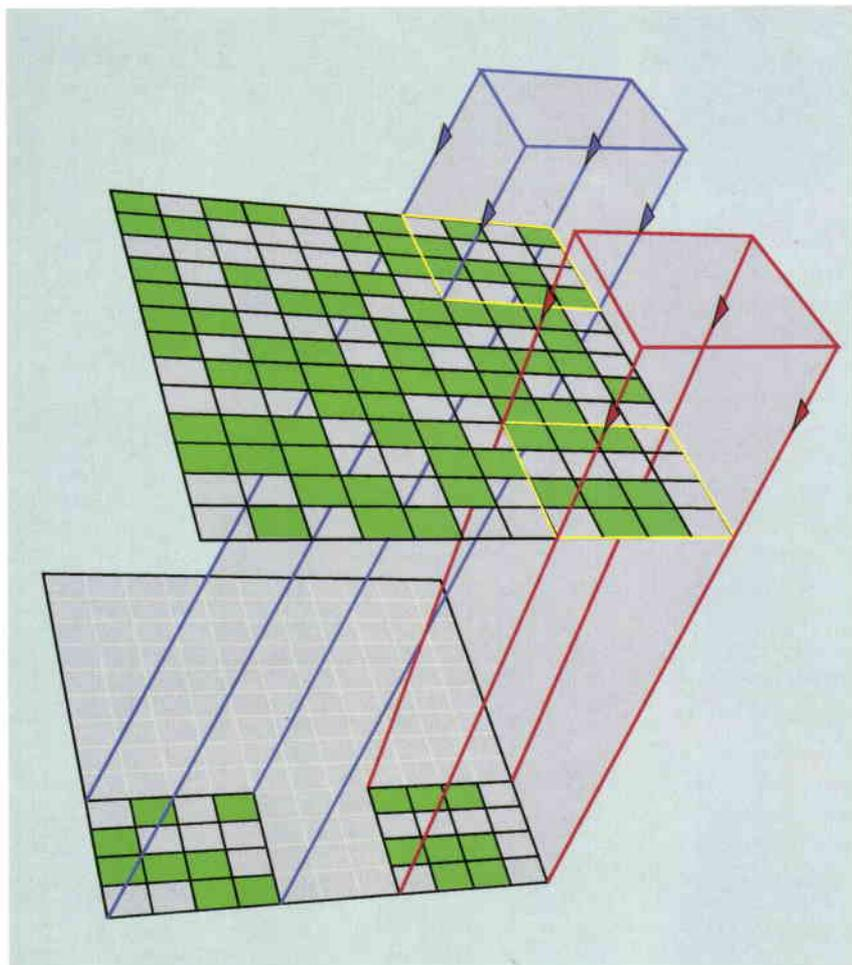
region of the sky, the difference is taken between the signal in all those detector elements that have a clear view of a source at the position under consideration, and that from detector elements for which the source is obscured by opaque regions of the mask. Thus, the detector background is measured exactly contemporaneously, using a subset of the detector elements intermingled with those observing the source.
