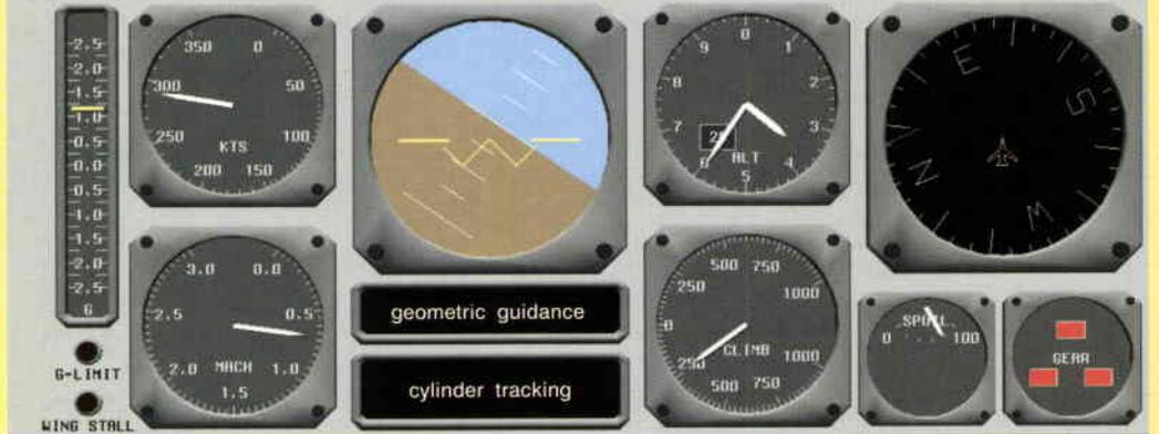
Figure 7. The screen as the pilot sees it during the cylinder tracking phase, with a visualisation of the local landscape (top), a simplified model of the head-up display (top, yellow overlay), and the instrumentation panel (bottom)
