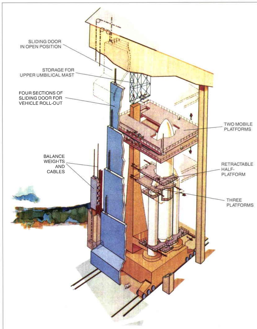
Figure 7. An artist's impression of the integration hall in the Final Assembly Building, with a launcher mounted on the mobile launch table, and staff on mobile access platforms working at different levels
