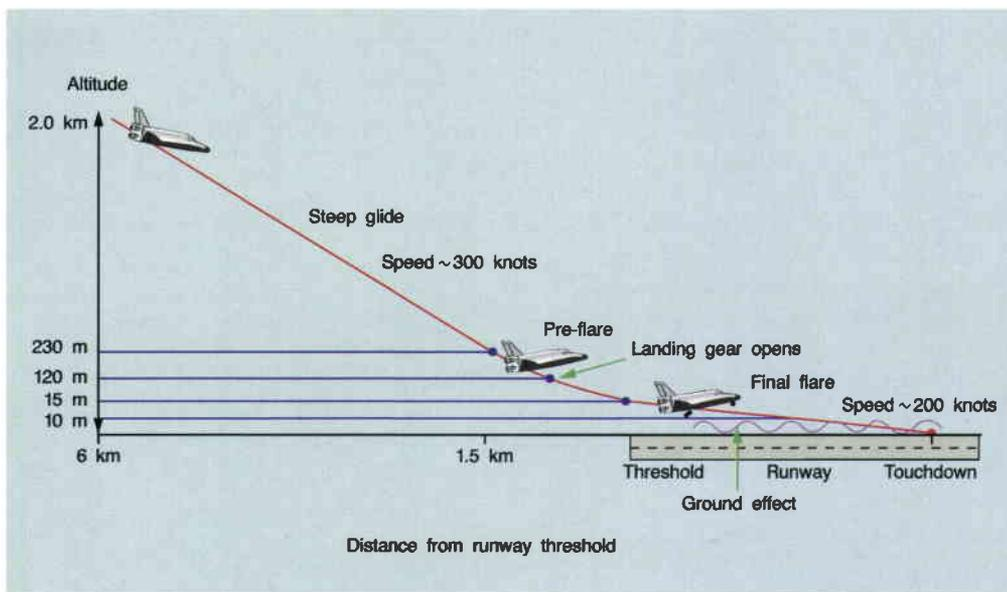
**Figure 4. The vertical trajectory during the final landing phases**
