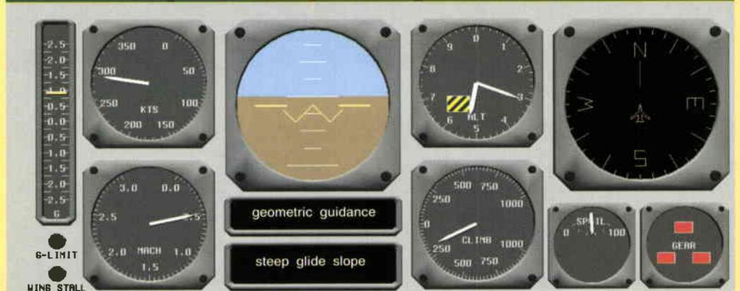
Figure 8. The screen showing a simplified model of the head-up display during the final phase before landing on the runway
