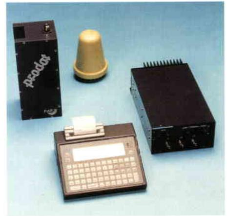
Typical mobile Prodat equipment that is installed in a truck, including the antenna (centre, back) and the keyboard which the driver uses to send and receive messages
