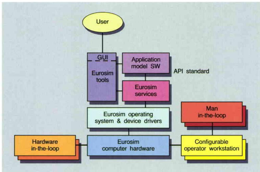
Figure 2. Layout of the Eurosim simulator
