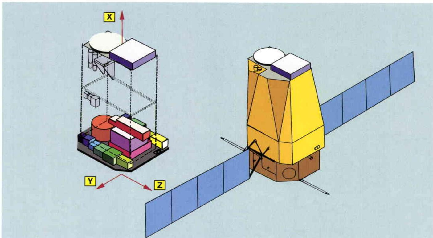
**Figure 4. Integral's payload configuration**
