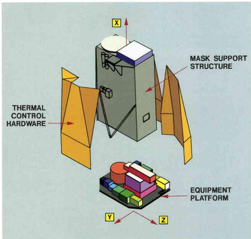
Figure 6. The Integral Payload Module – Exploded view
