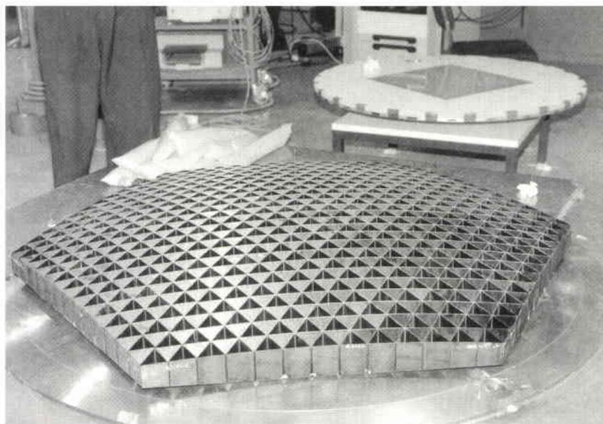
**Figure 5. Machined all-CFRP core for a highly dimensionally stable reflector (Photo courtesy of Dornier, Germany)**
