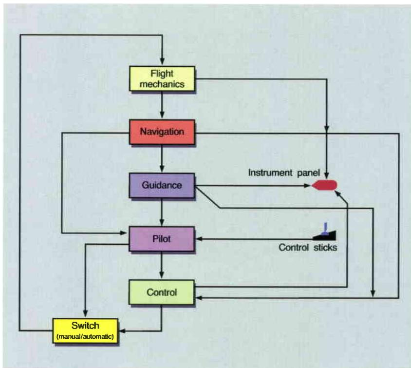
**Figure 5. Block diagram of the simulation**
