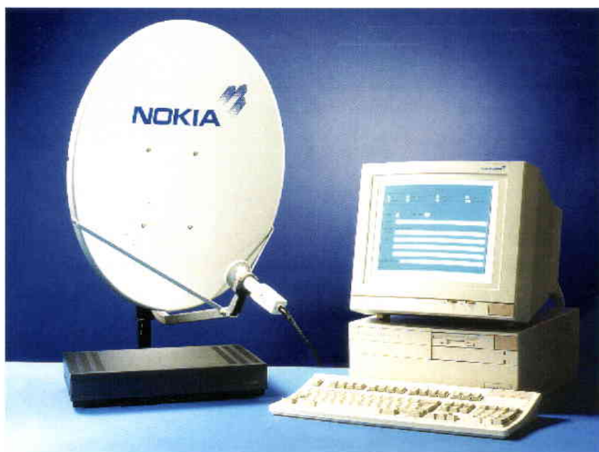
Figure 4b. A D2-MAC data receive terminal implementation. (In some implementations, the tuner/demodulator is integrated into the interface board). (Courtesy of Nokia Research Center, Finland)
