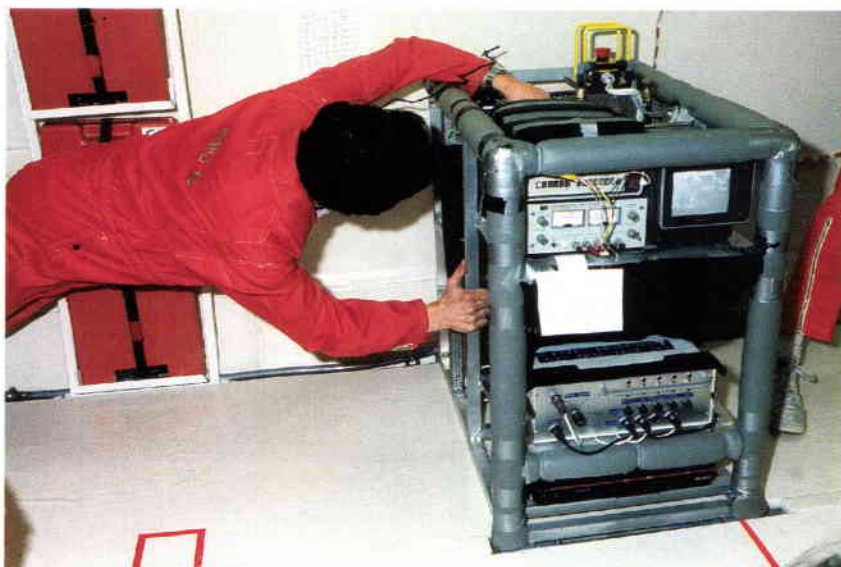
Figure 4. The gas trap during testing on a parabolic flight
