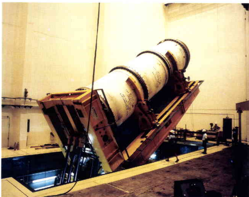
Figure 7. Airlock for the reception and tilting of the booster segments (in the BIP)
