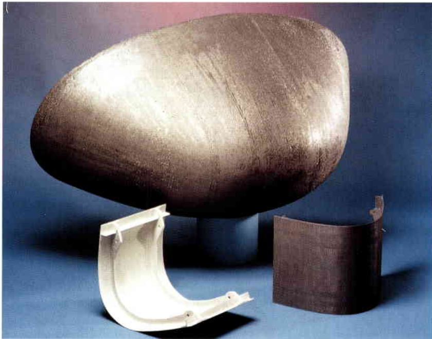
Figure 11. Full-scale carbon/carbon nose cap and leading-edge section (Courtesy of Aerospatiale)
