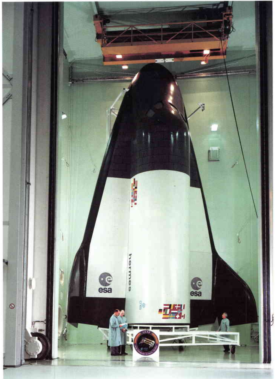
Hermes mock-up in ESTEC's Large European Acoustic Facility (LEAF) during fit-check and handling manoeuvres.
