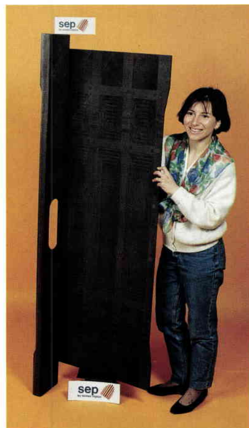
Figure 3. Skinex ® carbon/silicon-carbide (C/SiC) large thermal space-plane structure (Courtesy of SEP)
