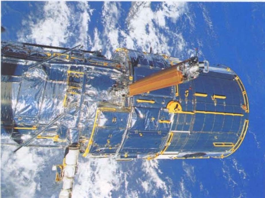
*The Hubble Space Telescope suspended in space from Space Shuttle Discovery's remote manipulator system, with one of the ESA-provided roll-out solar panels, yet to be deployed, in the foreground*
