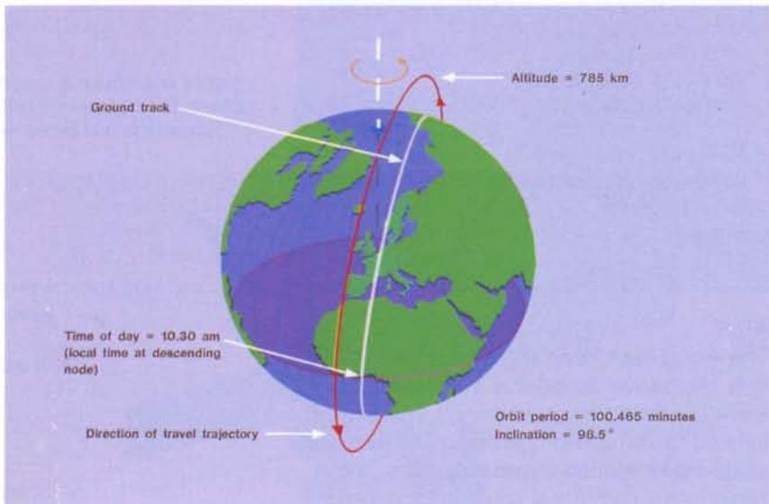
Figure 7. Geometry of the ERS-1 orbit
