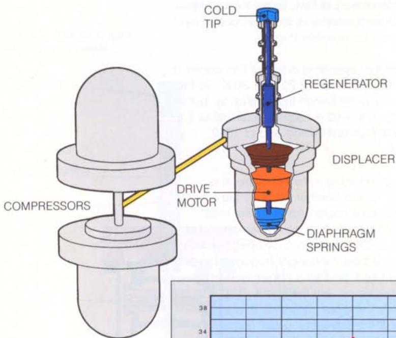
Figure 4. The 20 K dual-stage Stirling-cycle cooler
