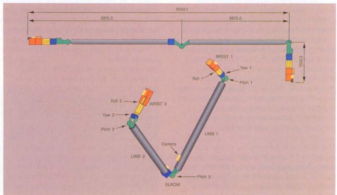
Figure 6. The HERA robotic arm
