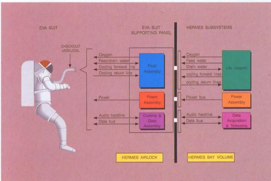
Figure 12. EVA system functional architecture and interfaces
