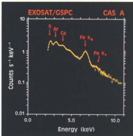
Figure 3. The X-ray spectrum of the SNR Cas A as measured by the GSPC instrument onboard Exosat. Emission lines are due to sulphur, argon, calcium and iron.
