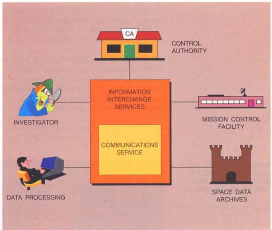
**Figure 6. The Information Interchange System (IIS) ground environment**
