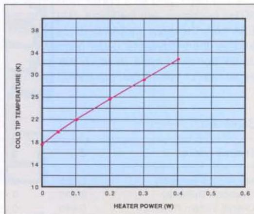
Figure 5. Performance curve for the 20 K cooler
