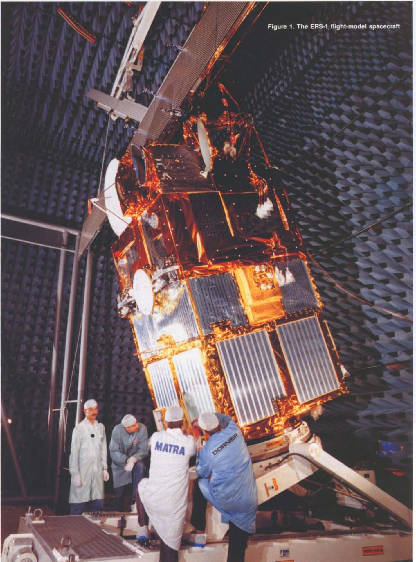
Figure 1. The ERS-1 flight-model spacecraft
