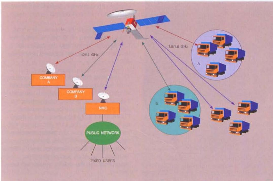
Figure 5. Land Mobile Satellite System (LMSS) configuration
