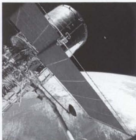
Cover: Hubble Space Telescope suspended in space from Space Shuttle Discovery's remote manipulator system, with one of the two ESA-provided roll-out solar arrays deployed in the foreground (see page 94) (photo: courtesy of NASA)
