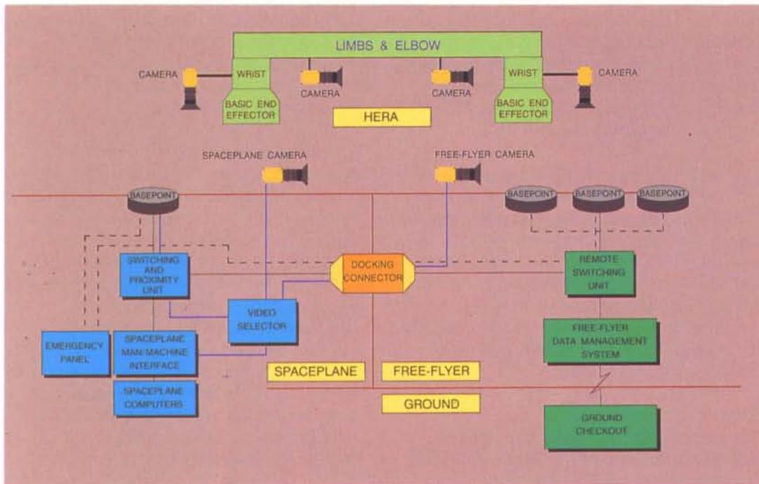
Figure 7. The HERA functional-control architecture
