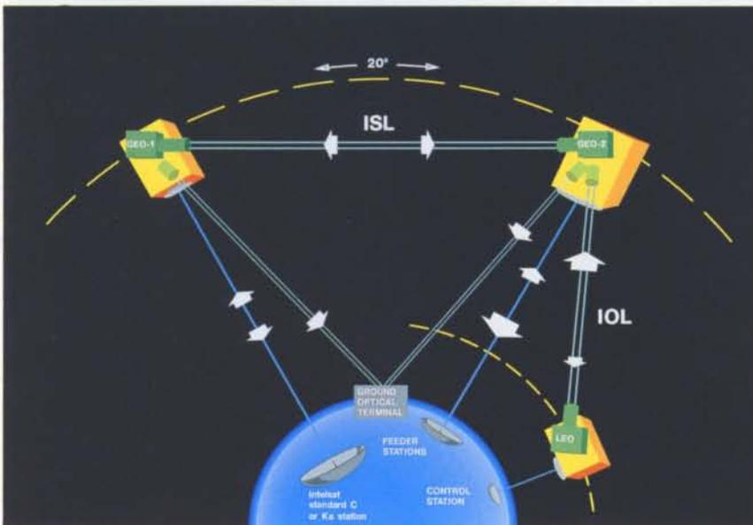
**Figure 2. The Silex system configuration**
