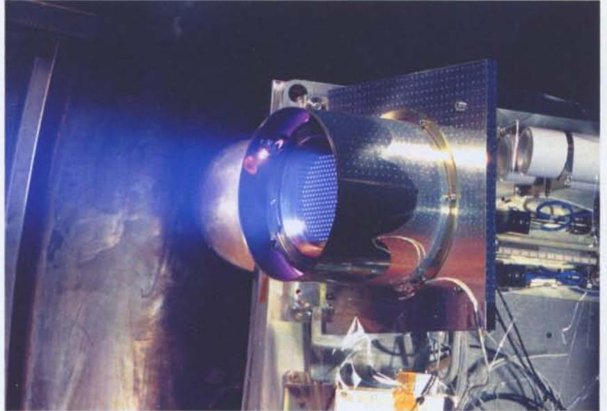
**Figure 7. A RIT ion thruster undergoing test firing in a vacuum chamber (courtesy of MBB)**
