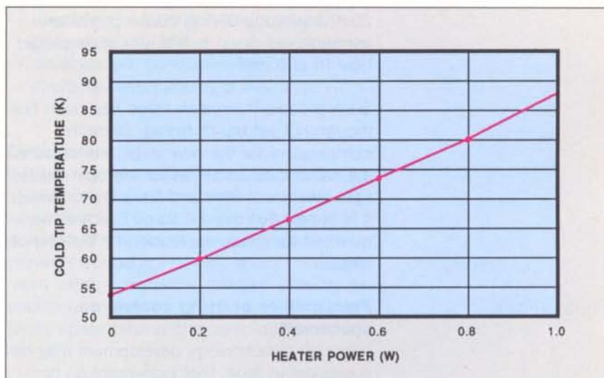
Figure 3. Performance curve for the 80 K cooler
