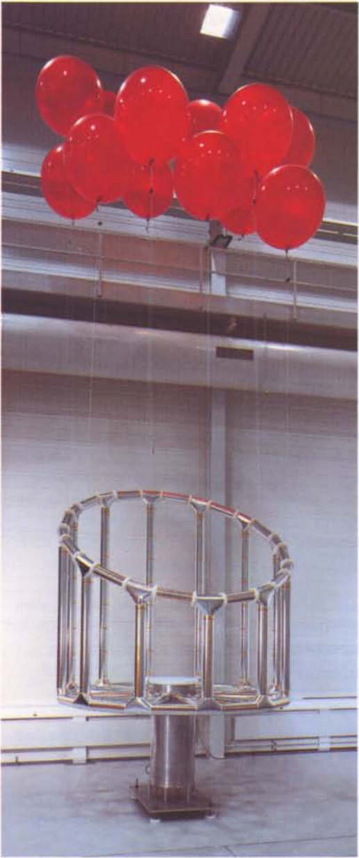
Figure 9. The Far Infra-Red Space Telescope's inflatable space-rigidised thermal shield structure
