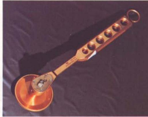
Figure 5. (a) An EVA manual tool, incorporating ratchet and mushroom head. (b) An EVA power tool, incorporating a torque limiter
