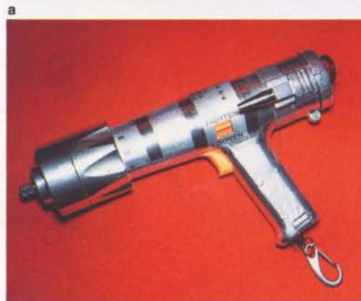
Figure 6. Fitting of Diode Box Connectors with a manual tool and torque limiter, illustrating the benefit of the 'wobble drive'
