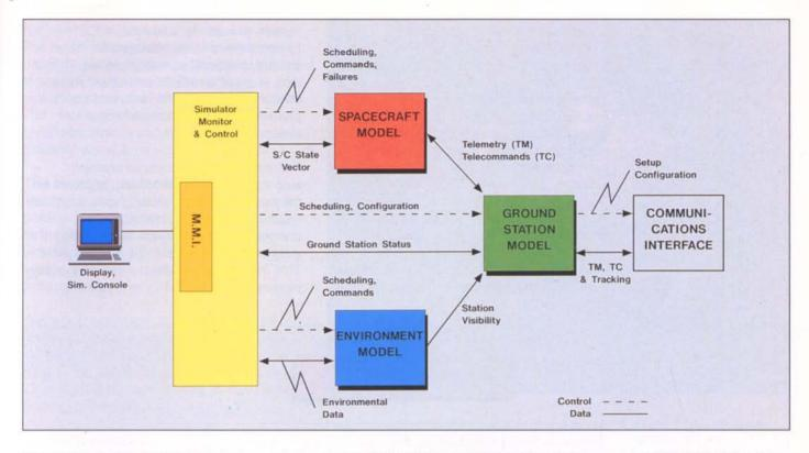
The ground-station model, the communications interface and the simulator monitoring and control function are, to a very large extent, spacecraft-independent and therefore common to all simulators. It was therefore possible to group them into a standard package, which provides a general framework to all simulator designers and ensures that a certain level of commonality is maintained in the end-user interface throughout the various simulator implementations.
