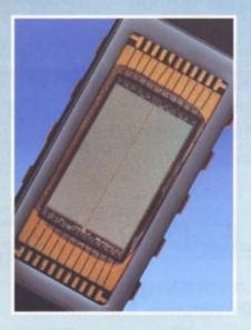
Silicon on Sapphire process. The Silicon on Sapphire eliminates the risk of latch-up and is the only commercially available technology that offers uncompromising performance in all aspects of hostile radiation environments.
