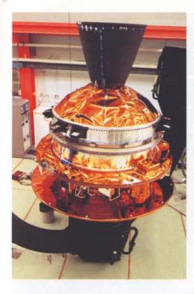
and a tether connecting satellite and deployer. It is a joint undertaking by the United States and Italy, the responsible agencies being Agenzia Spaziale Italiana (ASI) and NASA/Marshall Space Flight Center. The tethered satellite (Fig. 8) is being developed by Aeritalia Space Systems Group; Martin Marietta will provide the tether, the deployer and conduct overall system integration for NASA.
