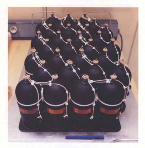
Figure 5. Nickel-cadmium batteries for the Olympus spacecraft
