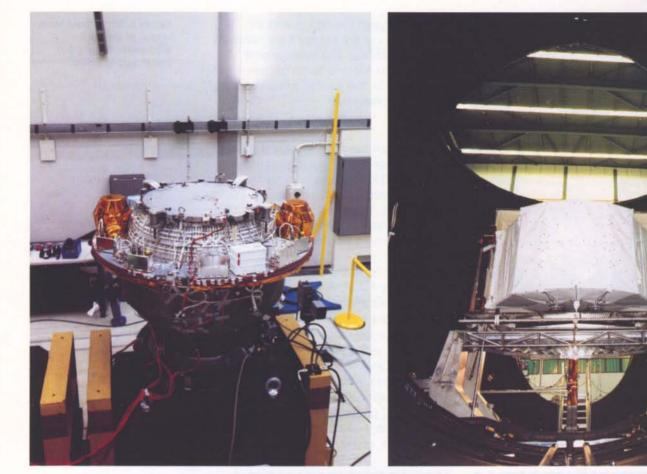
Figure 5. The IRIS ISS undergoing mechanical testing at ESTEC
