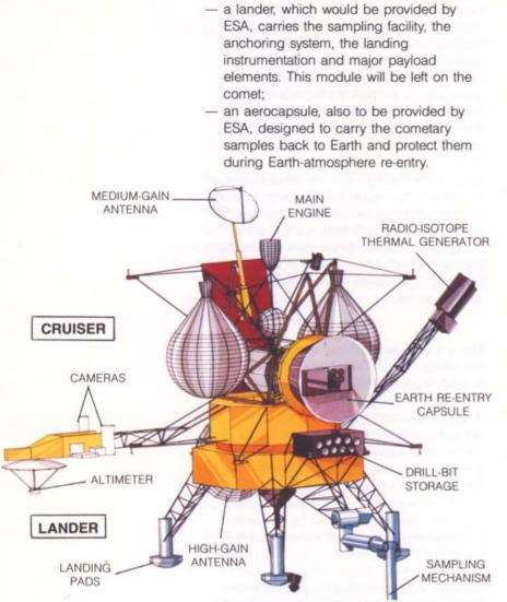
Figure 2. The Rosetta/CNSR space segment: carrier, lander and aerocapsule
