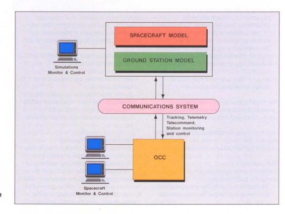
Figure 4. A typical simulation configuration at ESOC
