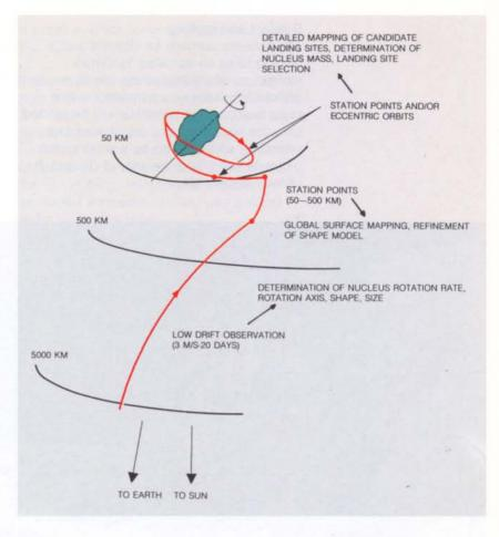
being developed and will be used to identify candidate landing sites that are suitable both from a safety (flat areas) and from a scientific point of view.
