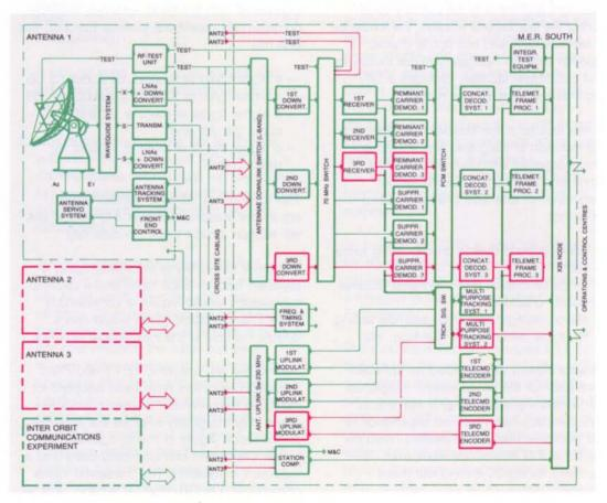
Figure 5. Block diagram of the Maspalomas Station
