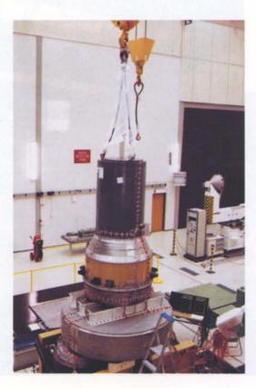
Figure 3. Structural/thermal model of the IRIS propulsion stage (ISS) under test at ESTEC
