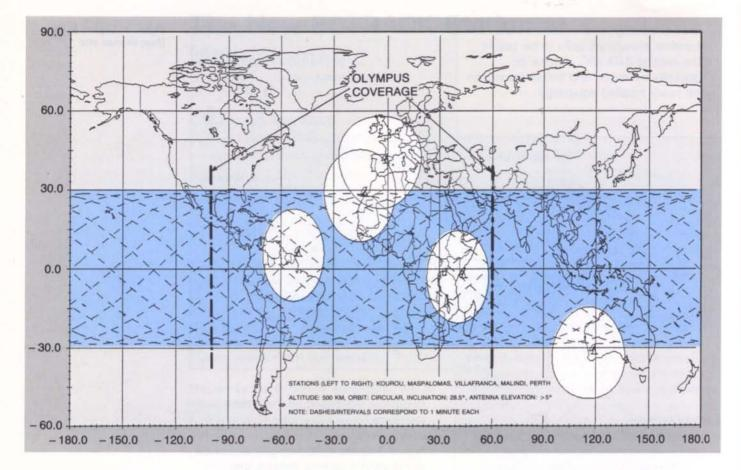
Figure 3. Ground-station coverage for Eureca
