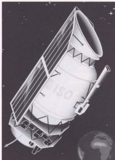
The satellite weighs 2400 kg and is about 5.3 m long and 2.5 m wide. Its short-term pointing accuracy (jitter) will be about 2 arcs. The downlink data rate will be 33 kbit/s, of which about 24 kbit/s will be dedicated to the scientific instruments.
