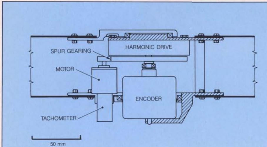
arm segments and hinges occupies a significant part of the working volume and restricts the very operation of the arm itself, so every possibility was pursued to minimise the size of the arm.
