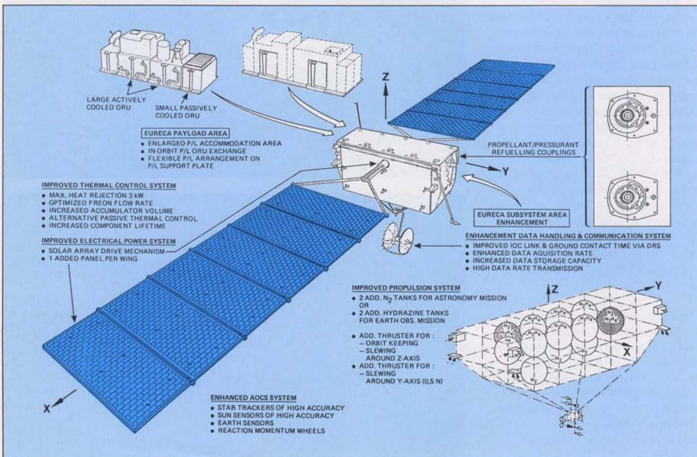
Figure 7 — Artist's impression of a Eureka carrier being serviced aboard the Space Shuttle
