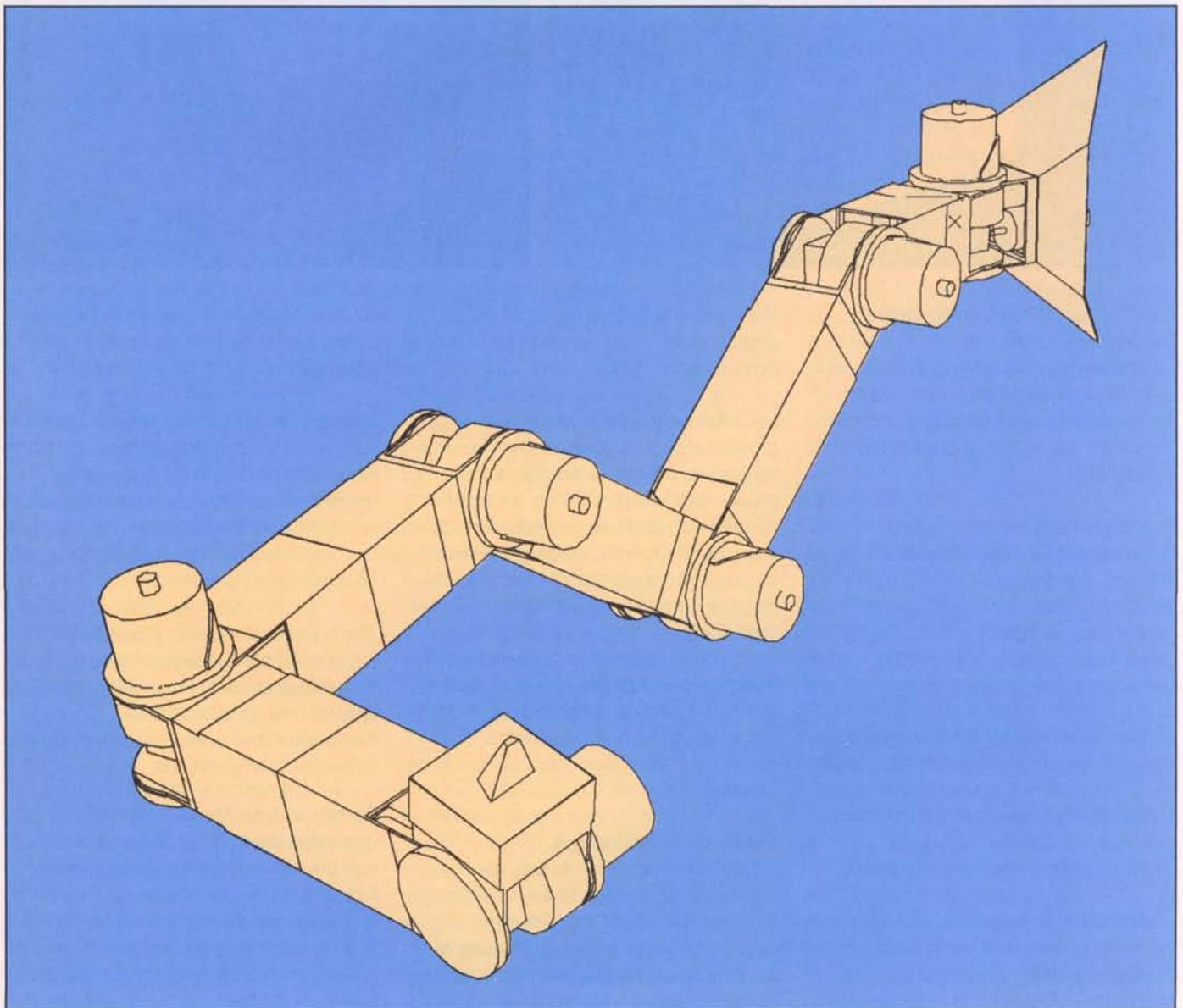
Figure 8 — Computer-graphics-generated view of an advanced manipulator servicing a number of facilities
