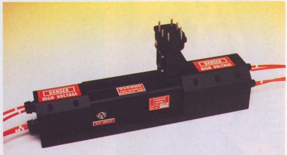
Figure 9 — Breadboard of a heterodyne spectroscopy receiver for the 300–1000 GHz band
