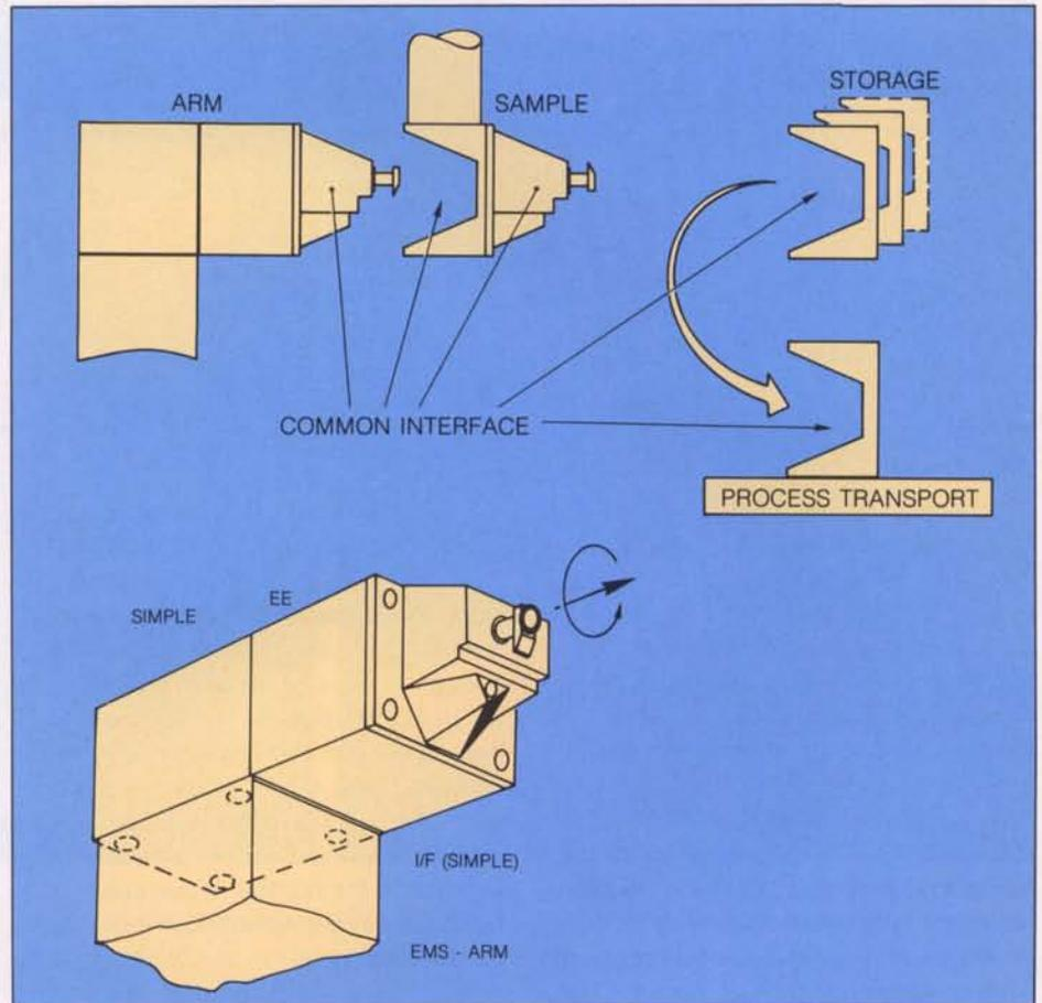
Using a similar grapple-fixture interface on the process transport mechanism would enable the same device to be used for the attachment of the sample, thus minimising the hardware.
