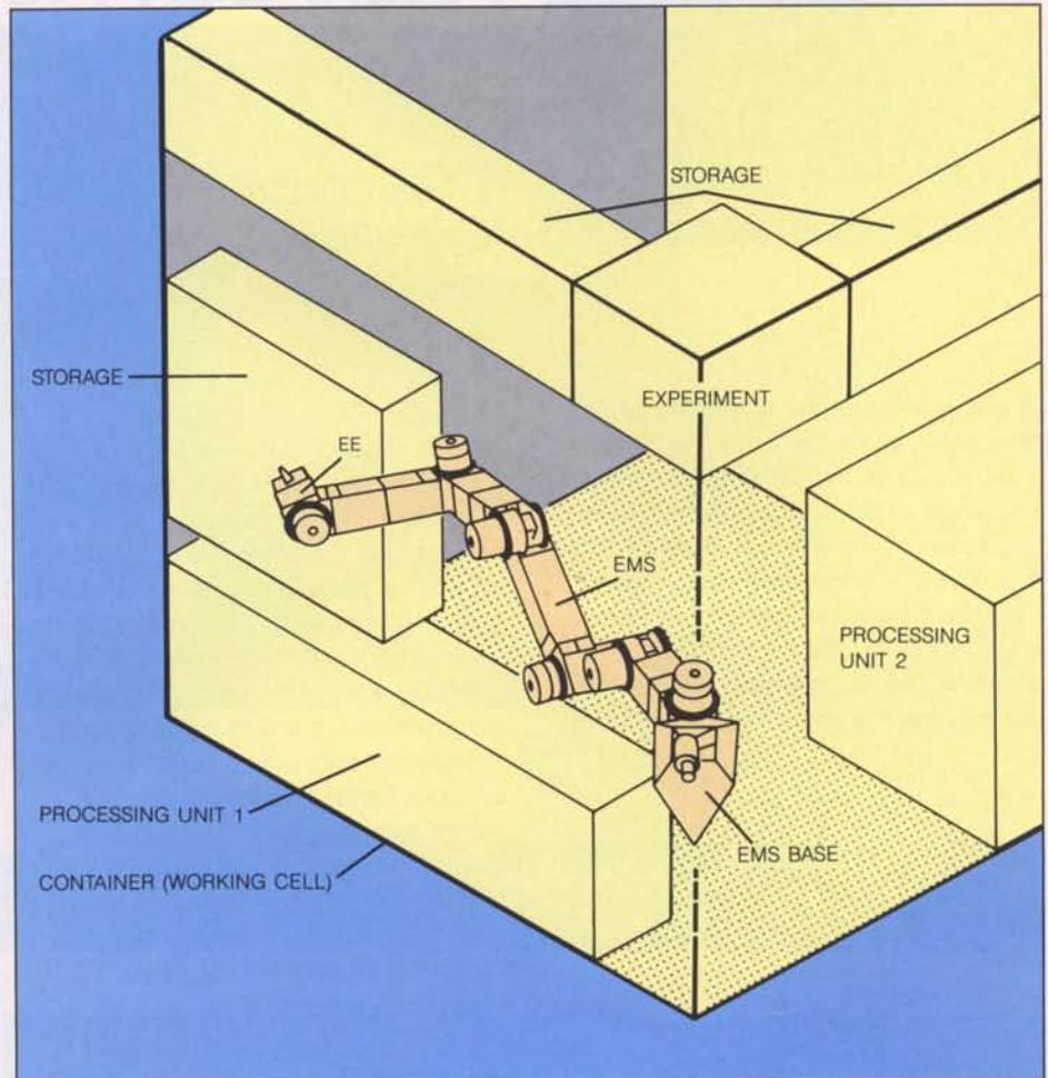
The reliability demands would be higher in this event, so the proposed configuration includes redundant drive-sets at each articulation and redundant electronics and wiring. Individual blocking means could be implemented on each joint.
