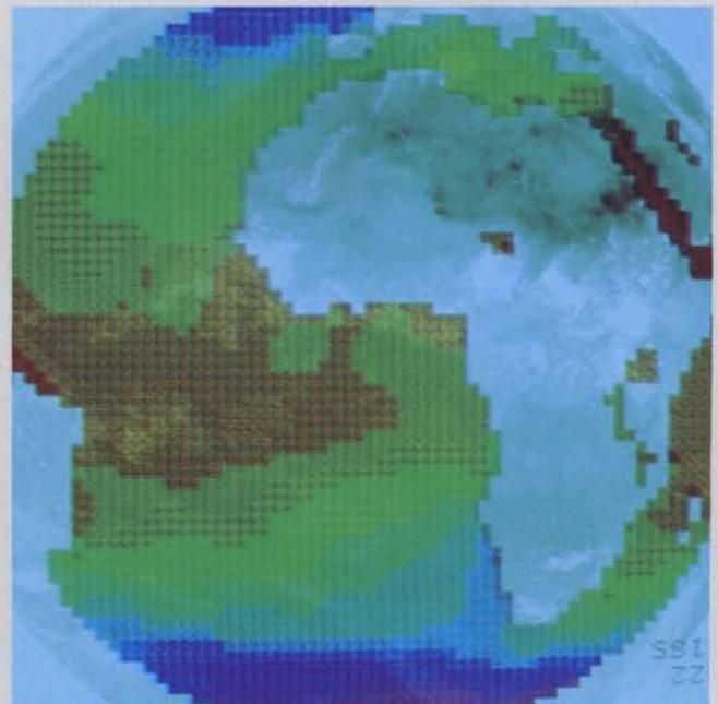
Figure 6 — Upper Tropospheric Humidity (UTH) derived primarily from Meteosat water-vapour channel data
