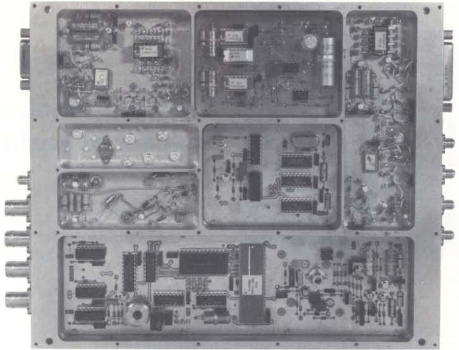
select the system's operational or test-mode configuration. In the test mode, the relays enable the user to apply to the converter a spectrum centred on the 70 MHz carrier either from the modulator ('short loop' configuration) or from the station front-end ('uplink test' configuration). In both cases the converter applies the same spectrum, centred on a 10 MHz carrier, to the demodulator.
