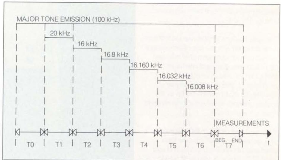
The frequencies used in the tone-ranging system are: 100 kHz (major tone), 20 kHz, 4 kHz, 800 Hz, 160 Hz, 32 Hz and 8 Hz (minor tones). Since each of these tones is obtained from the previous one by simple frequency division, the 8 Hz minor tone serves as the time-base reference for all the other tones. The 8 Hz tone is therefore also called the 'reference tone'.
