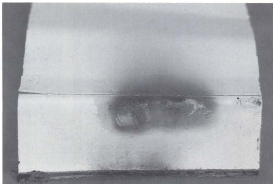
proposed rebuild alternative, the polyimide foil referred to above with the polyurethane paint was suggested, but this combination too was shown to be highly flammable.
