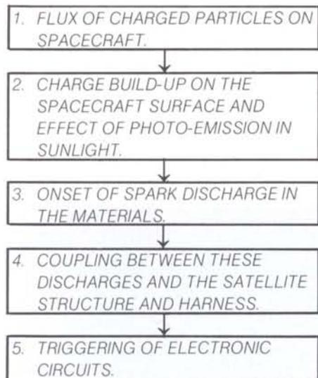
The most poorly understood links in this chain are items 3 and 4. Despite all the progress that has been made in investigating items 1 and 2, there is still no means of predicting or reconstituting where the discharge occurred and how it was coupled to the spacecraft structure and electrical cabling.
