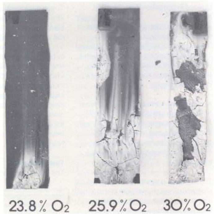
Figure 3 – Configuration Flammability Tests on thermal-blanket material
