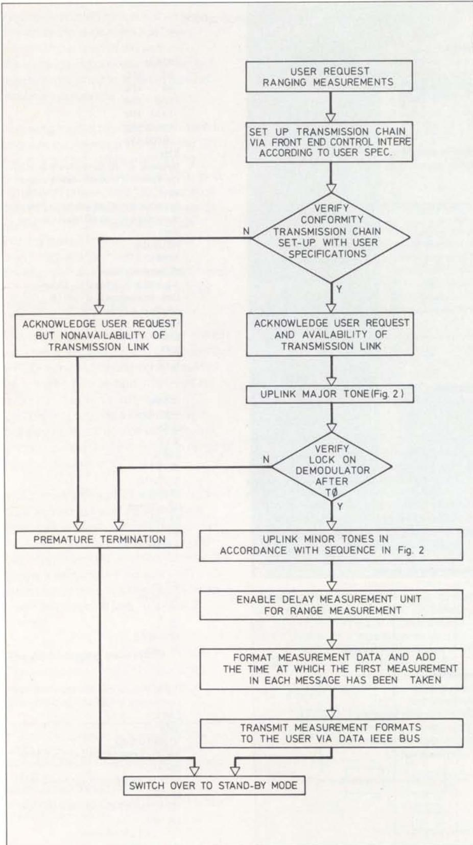
measurement is available to the control unit for formatting. Each format contains the results of 32 successive measurements (one group of measurements) and the time at which the first measurement in the message was started. A summary of parameters indicating the status of the system during the measurement is also included in the format, to provide the user with a means of analysing the system's behaviour in the case of abnormal measurement results.
