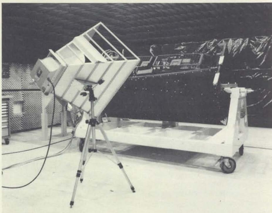
Space Telescope Faint Object Camera (FOC) undergoing EMC testing at ESTEC
