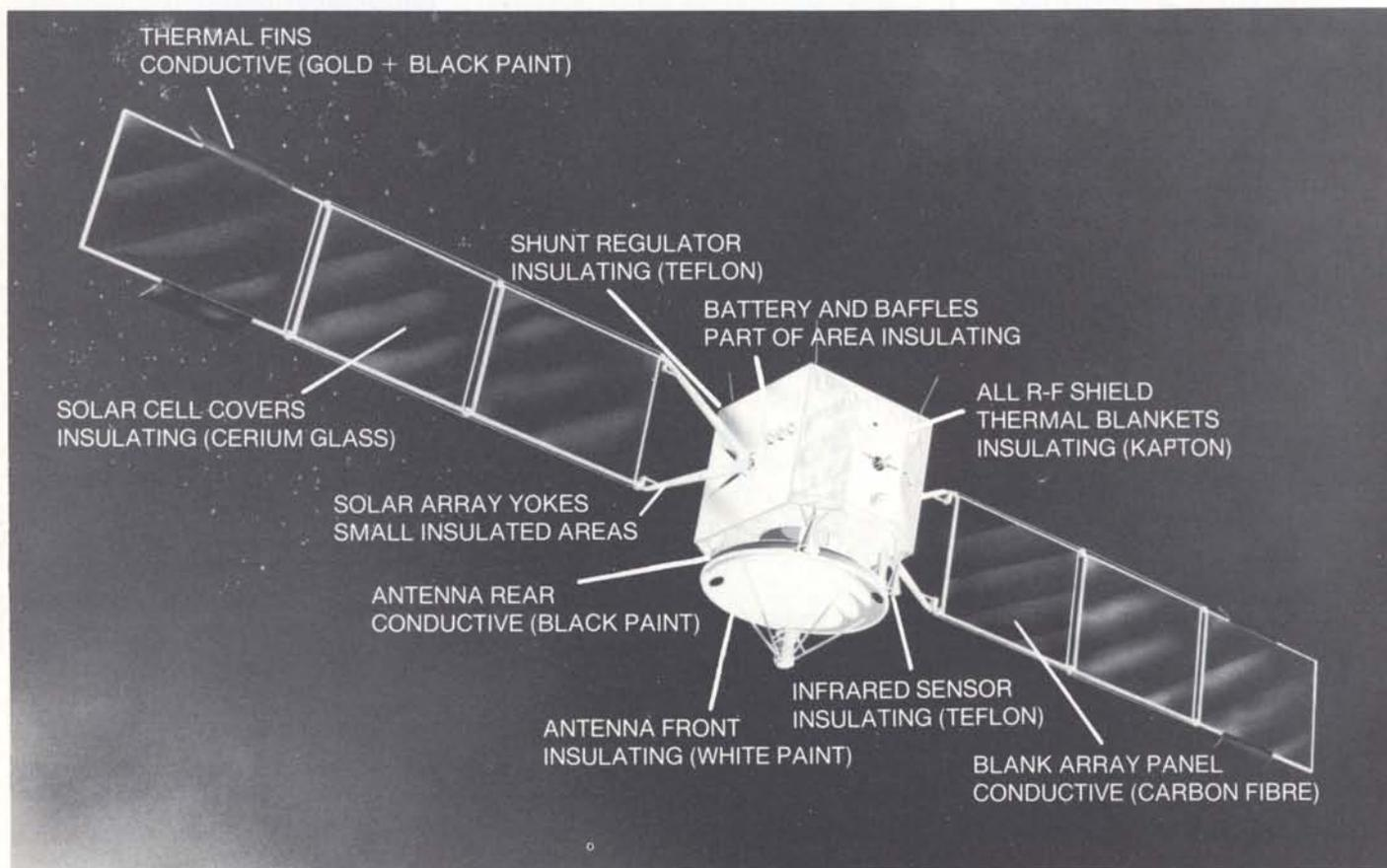
Figure 4 – North wall of the Marecs spacecraft, showing the shunt regulator, battery baffles, and infrared Earth sensor.
