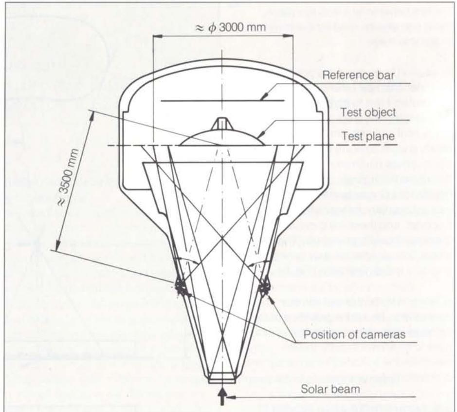
The new ESTEC photogrammetry system described in the following paragraphs came about as a result of a thorough investigation of the topic, started in 1979. This new system provides an accuracy of  $\pm 0.2$  mm in deformation measurements for tests in the HBF-3 facility. Moreover, the system could be applied without major difficulty to other vacuum facilities, such as the ESTEC Dynamic Test Chamber (DTC) and it can also be used under ambient conditions.
