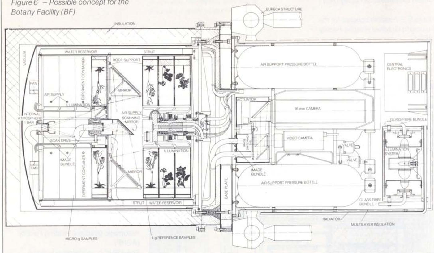
will consist of an experiment module, which is effectively a single temperature-controlled chamber to contain all experiment equipment and samples, and a service module, providing life support, illumination, data handling, etc.
