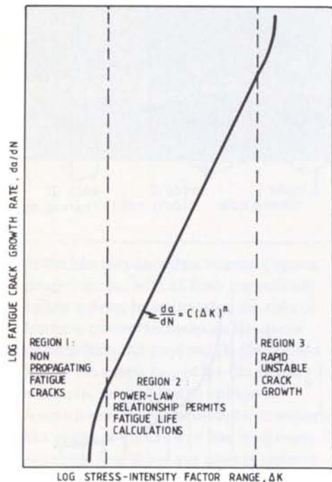
propagate under cyclic stress fluctuations. In region 2 the fatigue-crack propagation behaviour beyond  $K_{th}$  can generally be expressed as:
