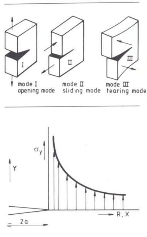
$K_I$  is the stress intensity factor for fracture mode I. It correlates the material properties, the crack geometry, and the stress field.  $K_I$  is the most important parameter in fracture mechanics and can be expressed in a general form as
