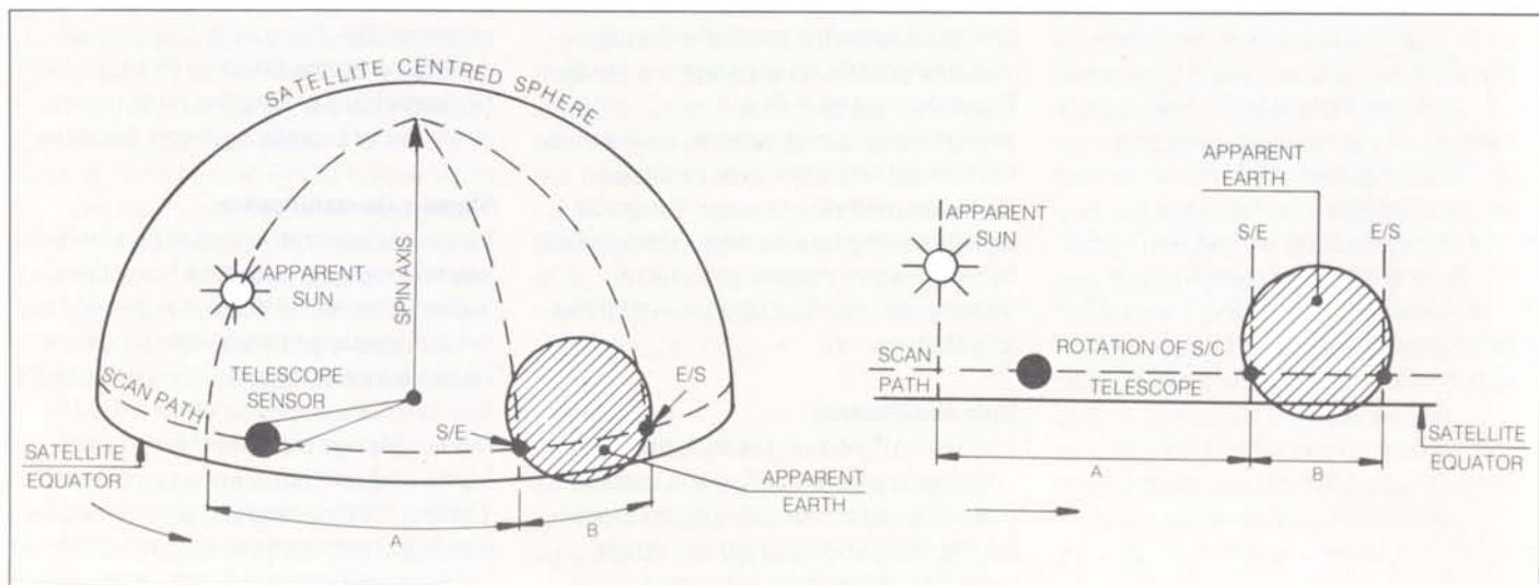
Figure 2 – Operating principle of a fan-beam sensor
