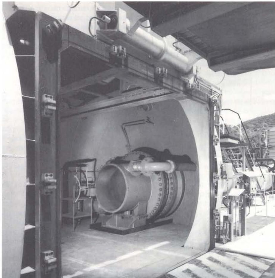
*Figure 4 – The test bench, on which the motor under test is mounted in a cantilevered position. The carbon-felt blanket on the nozzle of the motor is used to protect the surroundings from the intense heat radiated by the exit cone*
