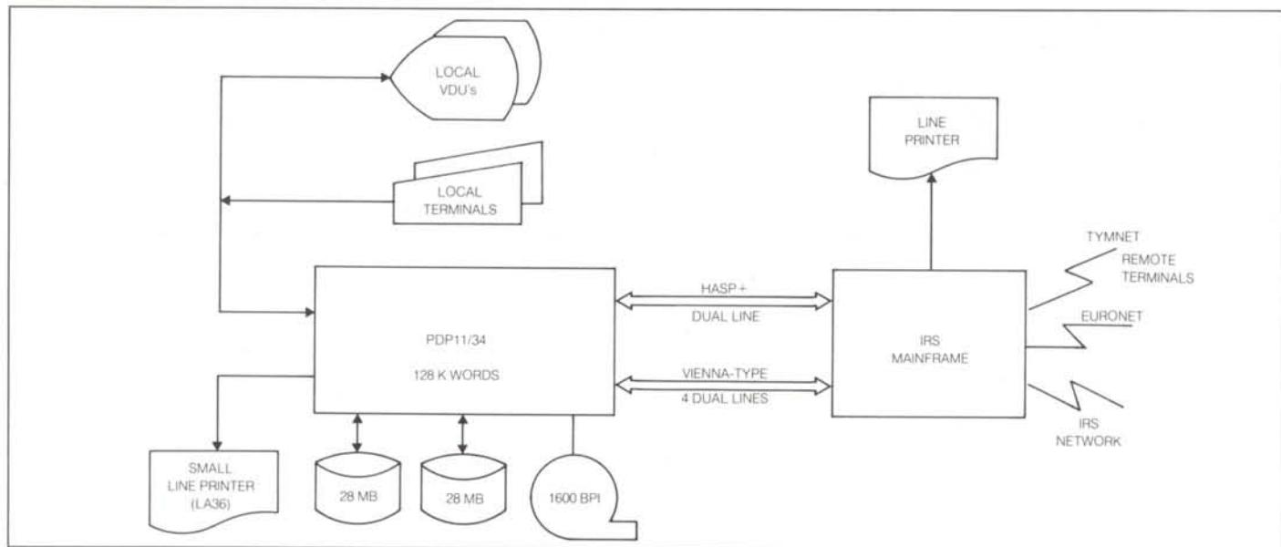
'Vienna-type' connection\* allows IRS users to interrogate the PDP 11/34 interactively.
