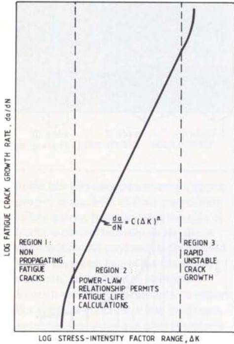
propagate under cyclic stress fluctuations. In region 2 the fatigue-crack propagation behaviour beyond  $K_{th}$  can generally be expressed as:
