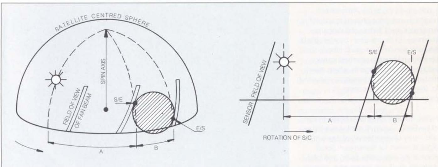
related to an instrument-fixed reference event on the cone, which is directly linked to the position of a satellite-body axis (Fig. 3b). The deviation between the mid-point of the Earth scan and the reference event, established via an on-board control loop, provides a measure of the depointing.
