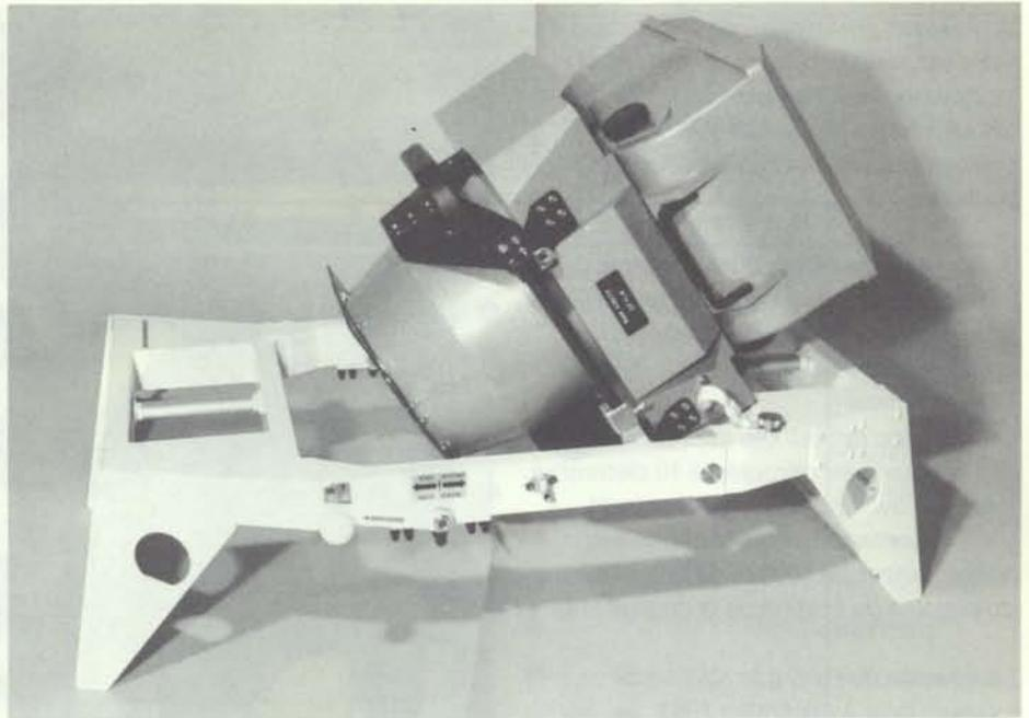
Last-minute hardware changes are under investigation for the Microwave Remote Sensing Experiment (MRSE). It had been originally assumed that, in the event of a power failure in the antenna motors, the antenna would return to its safe position due to the deceleration effect when the Shuttle enters the atmosphere. This can, however, no longer be considered sure and other means of returning the antenna to its safe position have to be found.
