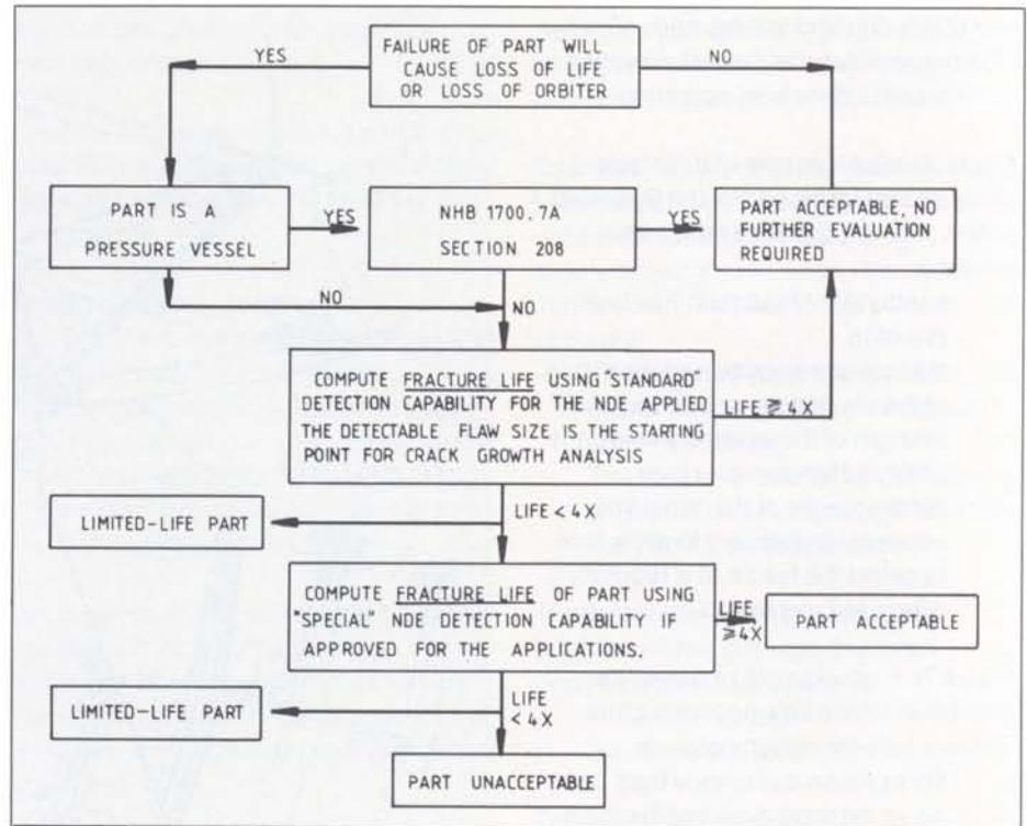
work and new stress-intensity solutions have been generated to predict the crack-growth behaviour of some critical items more accurately.
