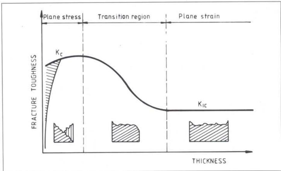
thickness. Only after a plain stress condition is reached in the material does the fracture toughness become independent of thickness and purely a property of the material itself.
