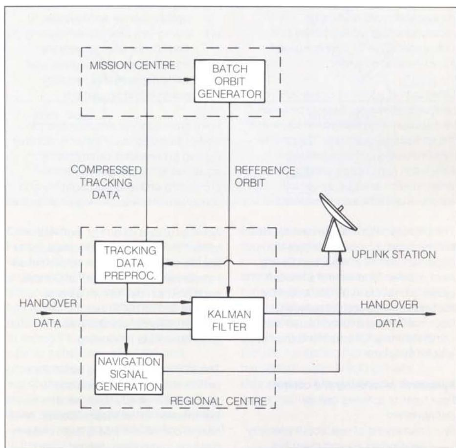
further-reduced data-transmission needs between Mission Centre and Regional Centres, but this has to be traded-off against increased data processing and the danger of discontinuity between segmented orbit-estimation data computed at different installations.
