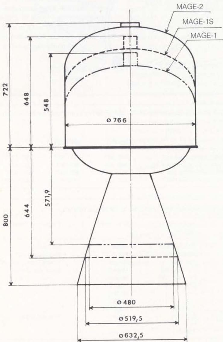
basically of a pressure vessel and an attachment skirt that allows the motor to be mated with the spacecraft.
