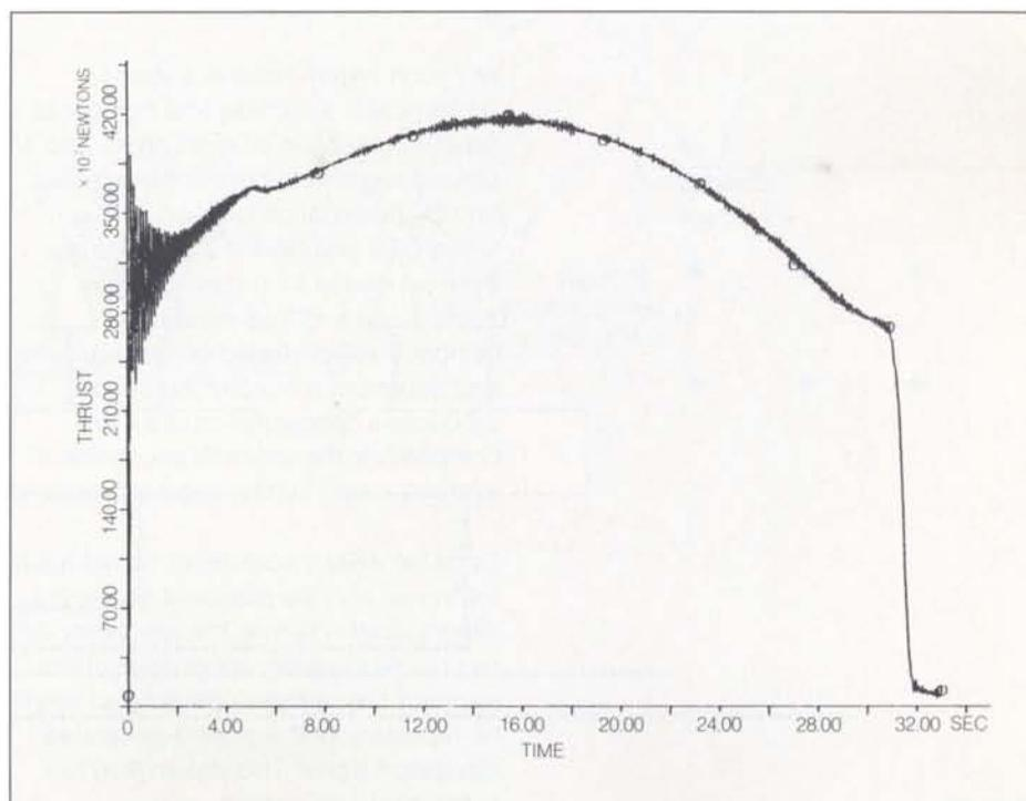
This motor was loaded with 490 kg of composite propellant type CTPB 1612 and produced a maximum thrust of 41.2 kN at a combustion-chamber pressure of 4464 kPa. The burn time was approximately 32 s and the maximum gas flow rate 15 kg/s. The motor was spun at 90 rpm during the test firing.
