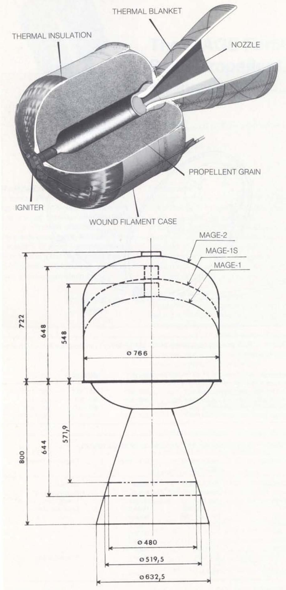
basically of a pressure vessel and an attachment skirt that allows the motor to be mated with the spacecraft.
