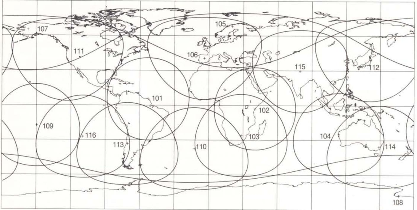
continuous visibility as the satellite moved in its orbit (Fig. 2). This basic tracking network which we call the 'Mission Execution (MEX) network', includes the central data-acquisition station mentioned earlier.
