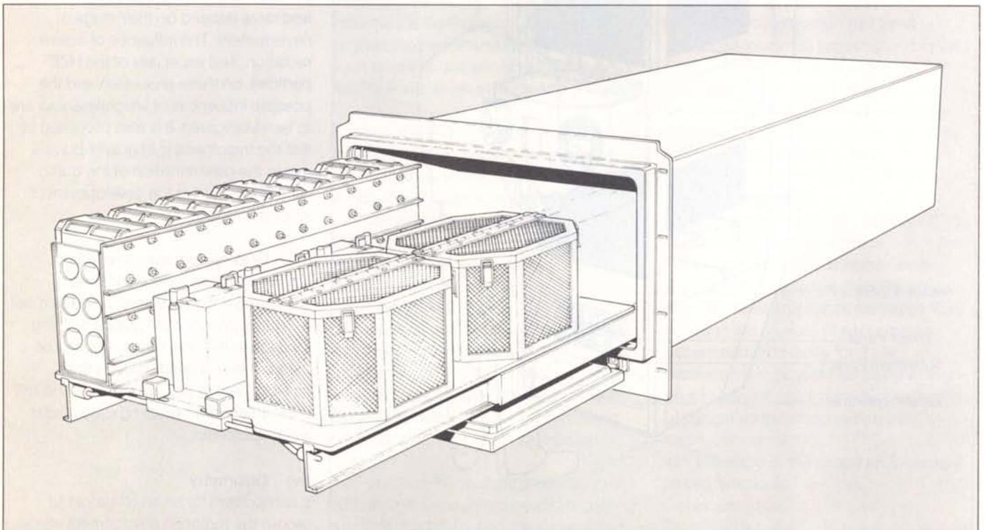
Figure 3 — Breadboard model of the cooler/freezer unit
