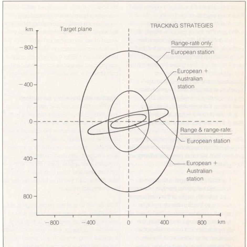
comparison of the results verifies once more that a combination of range and range-rate or angular data drastically reduces the size of the window.
