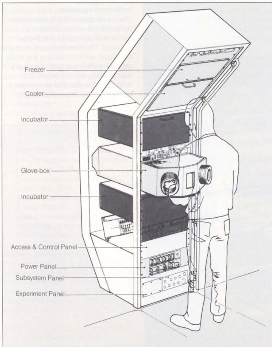
Figure 2 — Layout of an experiment incubator
