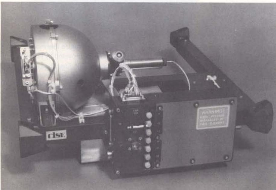
Figure 8 – The reactor chamber for the crystal-growth from solution experiments (ES 332/333)
