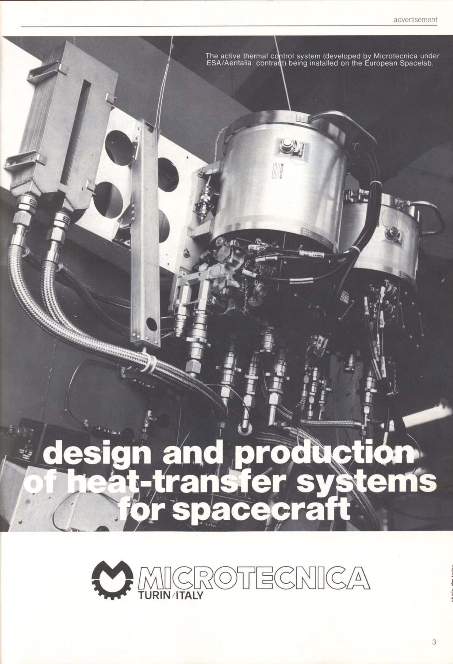
The active thermal control system (developed by Microtecnica under ESA/Aeritalia contract) being installed on the European Spacelab.
