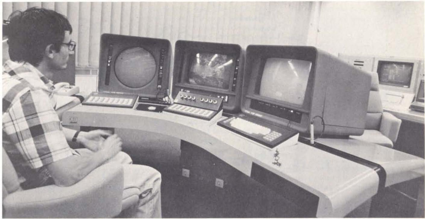
Figure 7 – The animated, coloured display used for manual editing of the MIEC winds. The short solid lines on the screen are wind vectors computed automatically from the cloud fields (light tones)
