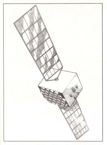
Figure 9 – Multibeam array concept permits communication with aircraft, ships and other mobiles from the same payload.
