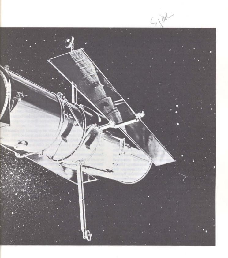
In addition, relative astrometric observations of stars can be performed using the fine guidance system of the spacecraft. This system will give a pointing accuracy of about 0.03" and a pointing stability of 0.007 arc sec (rms).
