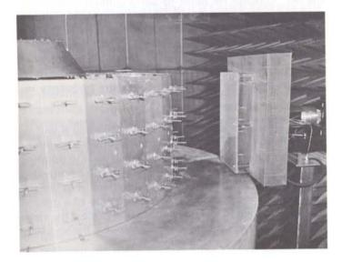
Figure 7 – This 'near-field' probing system was set up to verify the performance of the electronically de-spun Meteosat antenna after environmental testing. This verification, with the accompanying computer calculations shown in Figure 8, made it unnecessary to return the antenna for far-field testing.
