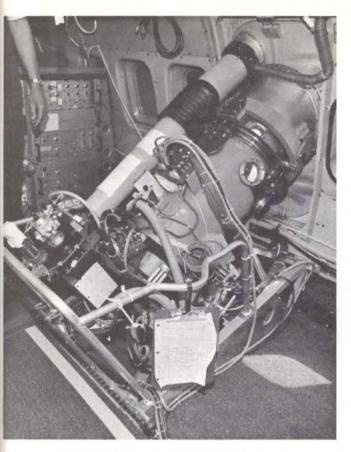
Figure 2 – Meudon IR telescope attached to open port of aircraft.
