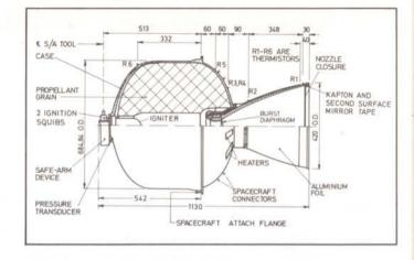
Figure 2 – Apogee boost motor configuration
