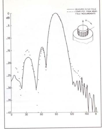
Figure 8 – Results of 'near-field' probe measurements on Meteosat transformed to 'far-field' values and compared with direct measurements; this represents one of the first uses of the near-field test principle.
