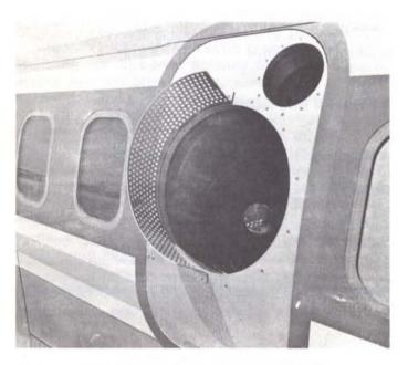
Figure 3 – Telescope viewing port and aerodynamic fence.
