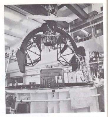
Figure 3 – OTS Spot Beam antenna about to be lowered into a vacuum chamber for thermal distortion tests. Stereo cameras allow recording of distortions in three dimensions. To minimise errors, the cameras are mounted with the antenna and go inside the chamber.
