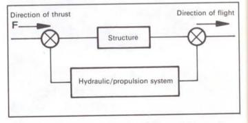
Figure 1 – Concept of vibrational coupling and POGO effect.
