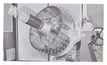
Figure 5 – A total of 138 individual radiators and slotted waveguides are used in Meteosat's antenna subsystem.
