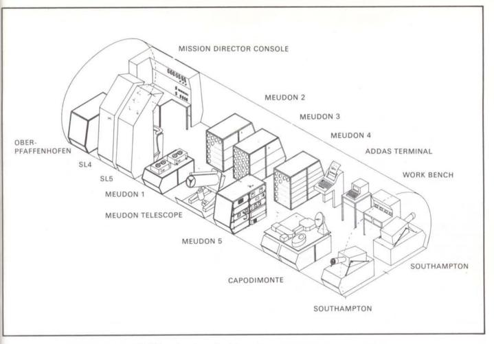
Figure 5 – Layout of DFVLR's planned CV-990 mock-up for payload integration.
