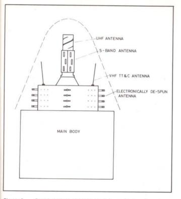
Figure 4 – Four independent antennas make up Meteosat's antenna subsystem (dimensions in mm).
