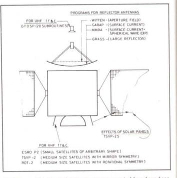
Figure 1 — The standard computer programs noted here have been developed for antenna design and to evaluate the influence of satellite structure on radiation pattern. These programs, verified extensively by comparison with measurements, are available to European industry and research organisations for use in space work.
