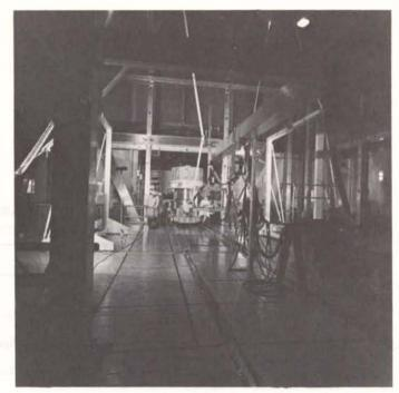
Figure 2 – Large Magnetic Test Facility at IABG, Munich. (Facility is capable of creating, within a spherical volume of 3m diameter, a residual magnetic field one hundred thousand times smaller than that of the earth. The magnetic coils are 15 m × 15 m × 15 m).
