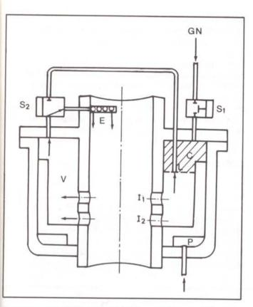
Figure 2 - Schematic of the POGO Correction System (PCS).
