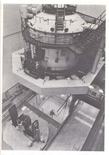
Figure 3 – Large Space Simulation Chamber at CNES, Toulouse, used for heat-balance tests. (Dimensions (main chamber): 7 m diameter × 9 m height. Parallel solar beam of 3 m diameter and max. solar intensity 1.4 times that in earth orbit. Shroud temperature 100-360 K. Motion simulator has continuous spin motion).
