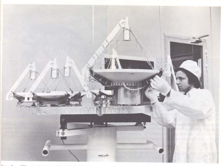
Figure 2 – OTS payload antennas will be the first on-board antennas to employ frequency re-use. Each antenna can handle dual polarisation in the same frequency band and in the same beam.
