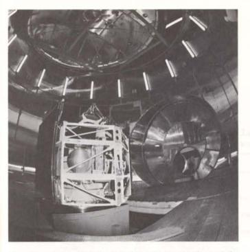
Figure 1 – Large Dynamic Test Chamber at ESTEC, used for deployment and spin tests and mass-properties measurements under vacuum. (Dimensions: 10 m diameter × 14 m height; vacuum to 10<sup>-2</sup> torr, internal mounting table connected to 90 ton seismic block).
