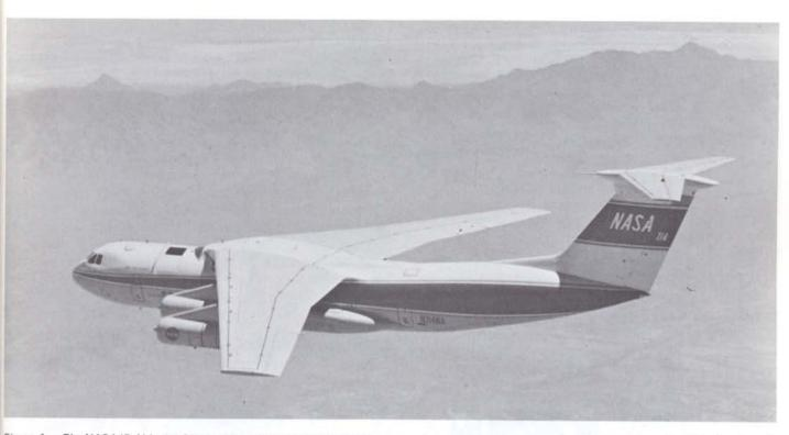
Figure 1 — The NASA IR Airborne Observatory. A 91 cm diameter IR telescope and star tracker are accommodated in a sealed section of the fuselage of the C141 jet aircraft. Observations are made by astronomers on board (Fig. 4) from altitudes above 12 km to reduce atmospheric interference.
