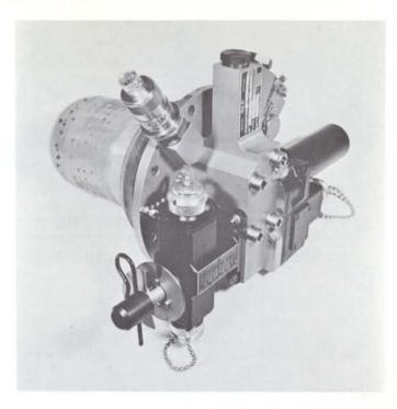
Figure 4 – Igniter/safe-arm device combination
