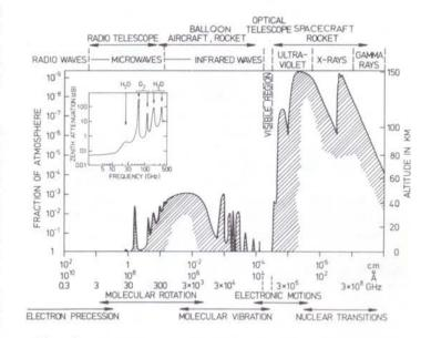
Figure 3 – Attenuation of electromagnetic radiation in the earth's atmosphere for the different wavelength ranges. The solid curve indicates the altitude at which the intensity of incoming radiation is reduced by 50%, illustrating the importance of going to space observation platforms for IR astronomy.
