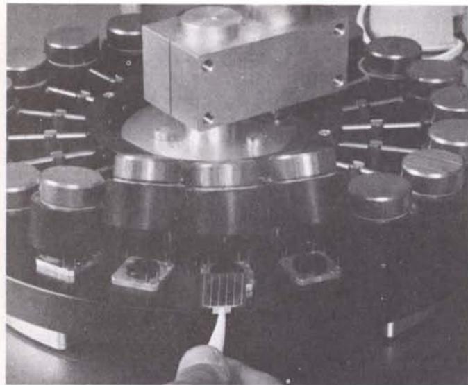
Figure 5 - Close-up of solar-cell covering with cover sheet.
