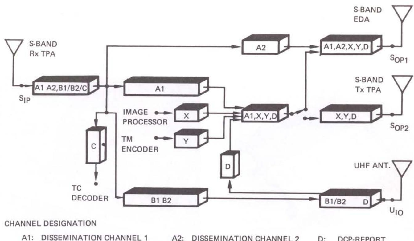
Figure 7 – Block diagram of Mission-Performance Telecommunication Subsystem.
