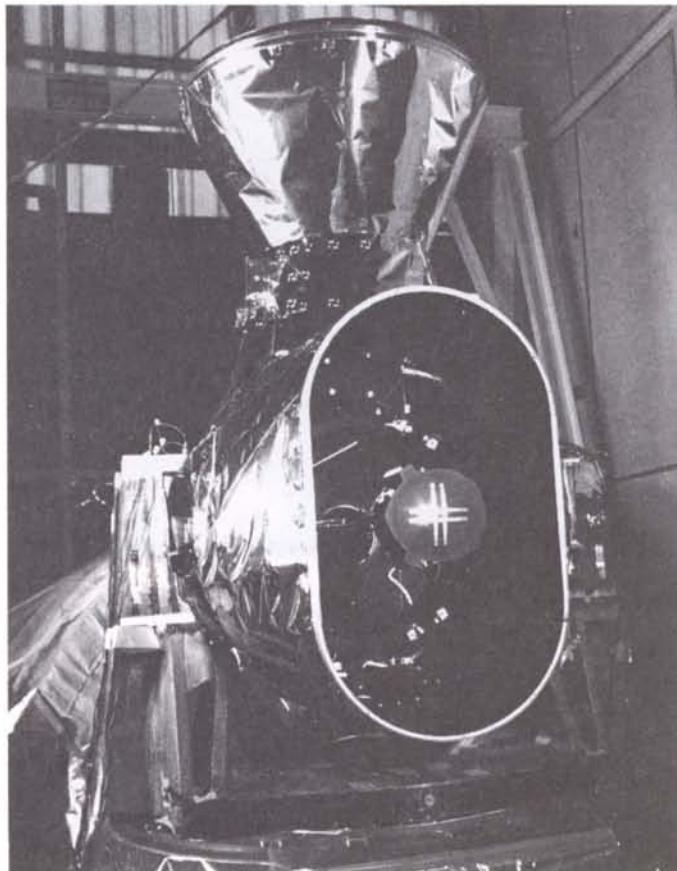
Figure 1 – The Meteosat radiometer during vibration testing in Toulouse.
