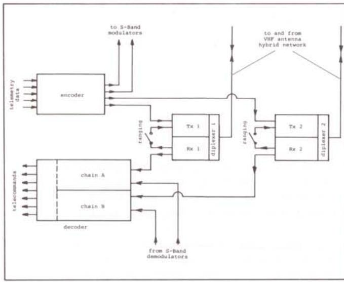
Figure 6 – VHF block diagram.
