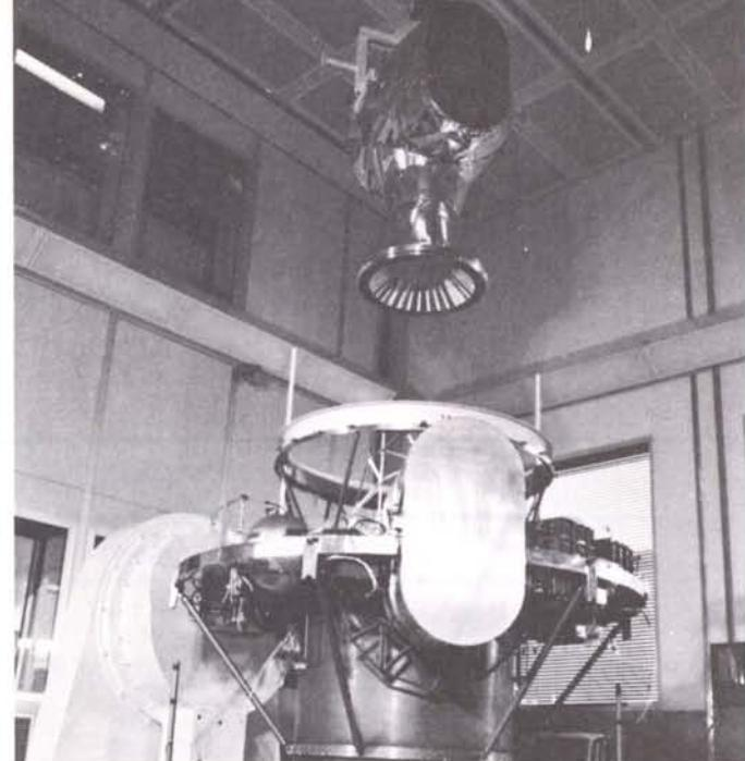
Figure 5 – Installation of the radiometer.
