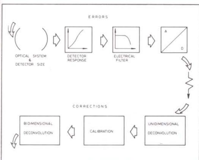
Figure 2 – Amplitude-processing scheme.
