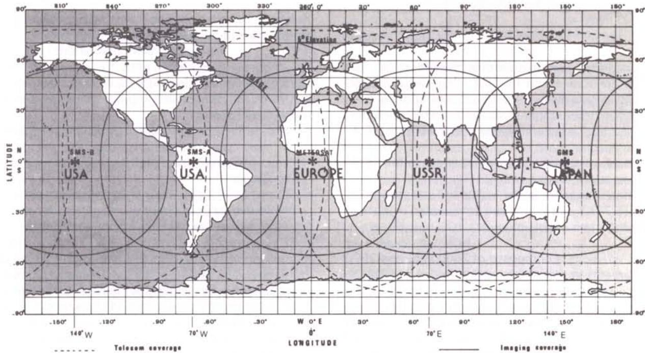
Figure 1 – Coverage of the geostationary meteorological satellites participating in the GARP experiment.
