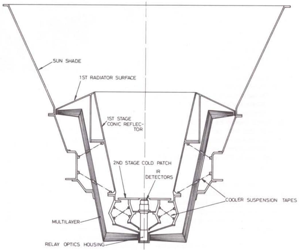
Figure 4 – Radiometer cooler (schematic)
