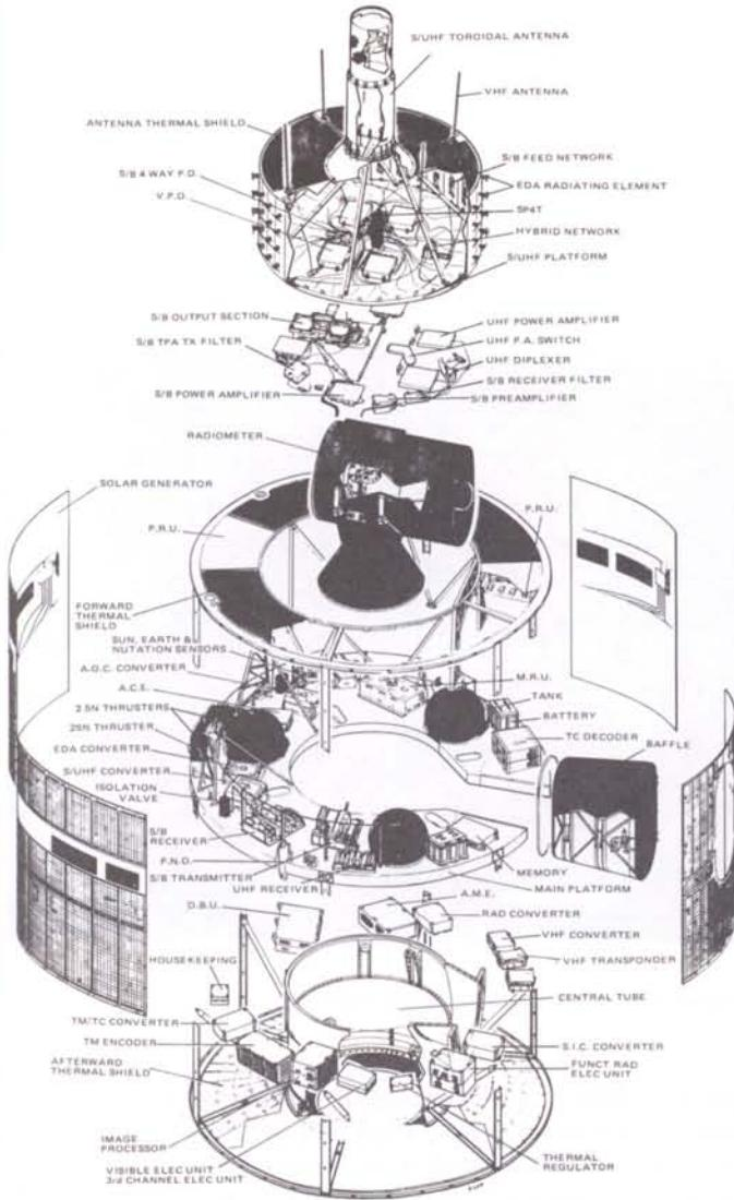
Figure 2 – Exploded view of the satellite.
