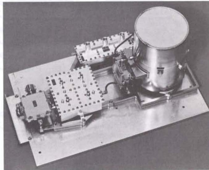
(b) S-band transmitter up-converter.
