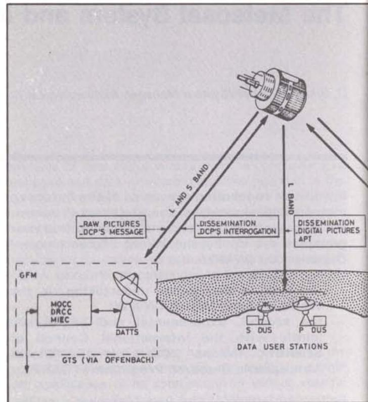
Radiance data are produced at the rate of one visible picture and one infrared picture of the complete earth's disc every 30 min. They are transmitted in quasi-real time, after on-board line stretching (explained later), to the Meteosat ground facility, where they are subjected to a correction process prior to the extraction of the meteorological information. The main characteristics of these images are summarised in Table 1.
