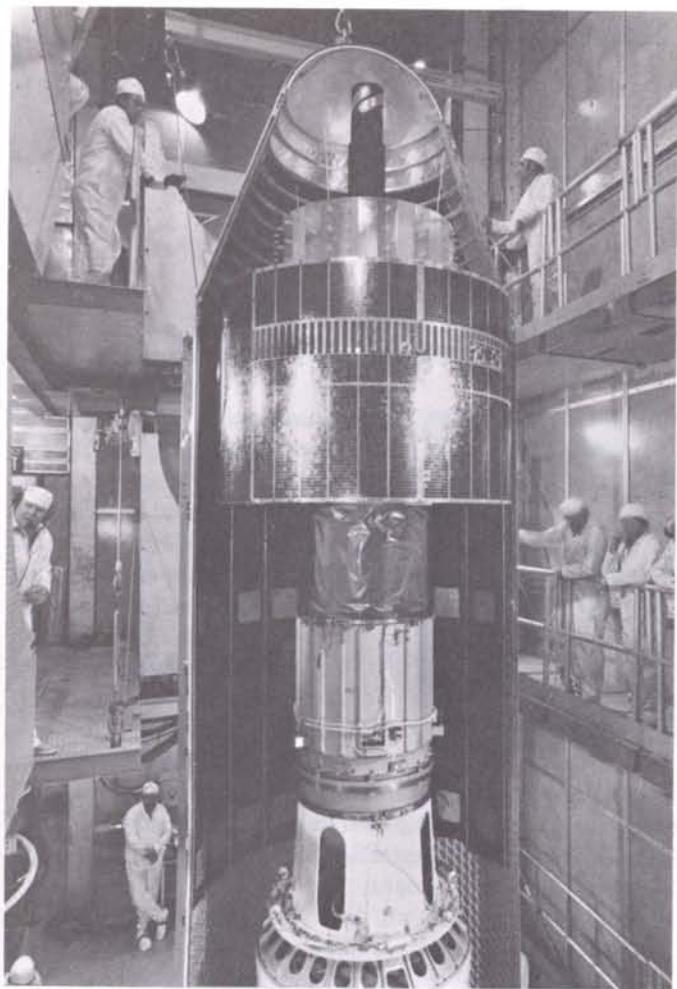
Figure 5 – Fairing installation.
