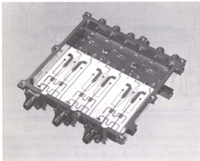
Figure 8 – (a) S-band transmitter multiplexer
