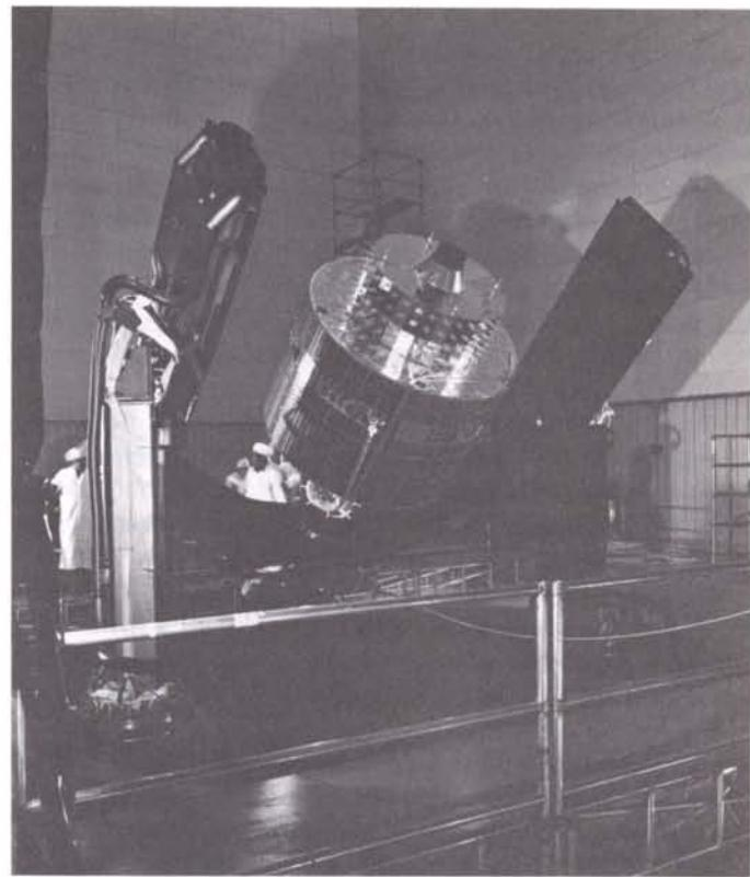
Figure 3 – Thermal model in preparation for solar vacuum test – transfer-orbit configuration.
