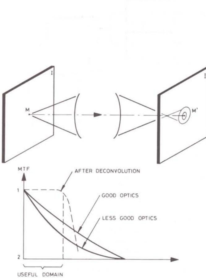
Figure 3 – Modulation transfer function.
