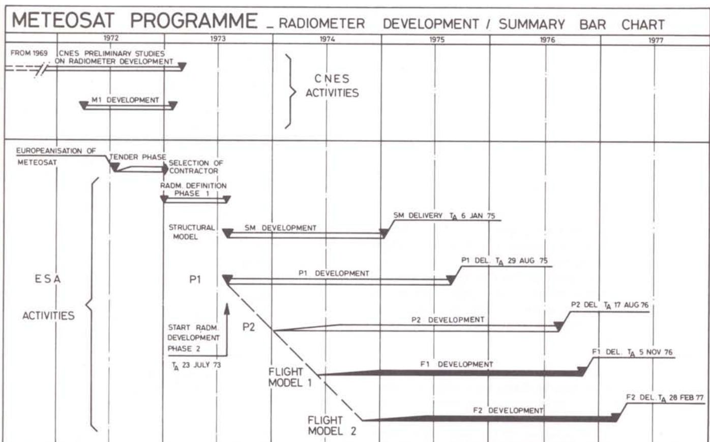
Figure 2 – Radiometer development/summary bar chart.
