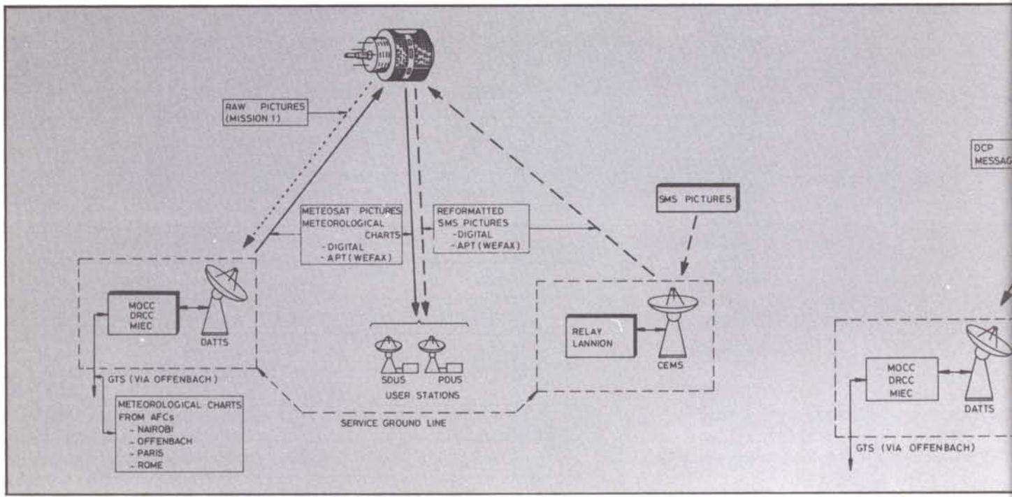
The DCPs, which may be installed either at a fixed site on land, or on mobile supports such as ships, buoys or balloons, will be
