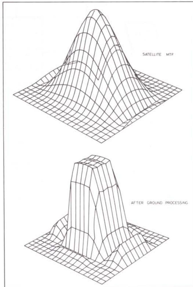
Figure 4 – Meteosat Modulation Transfer Function (infrared channel).
