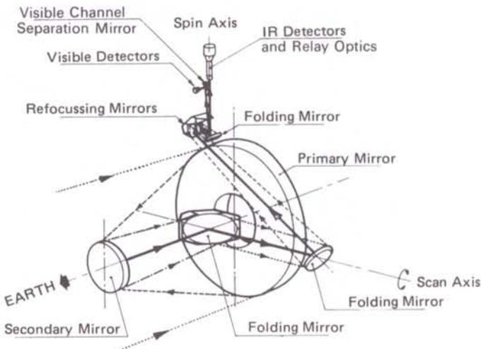
Figure 3 – Radiometer optics (schematic)
