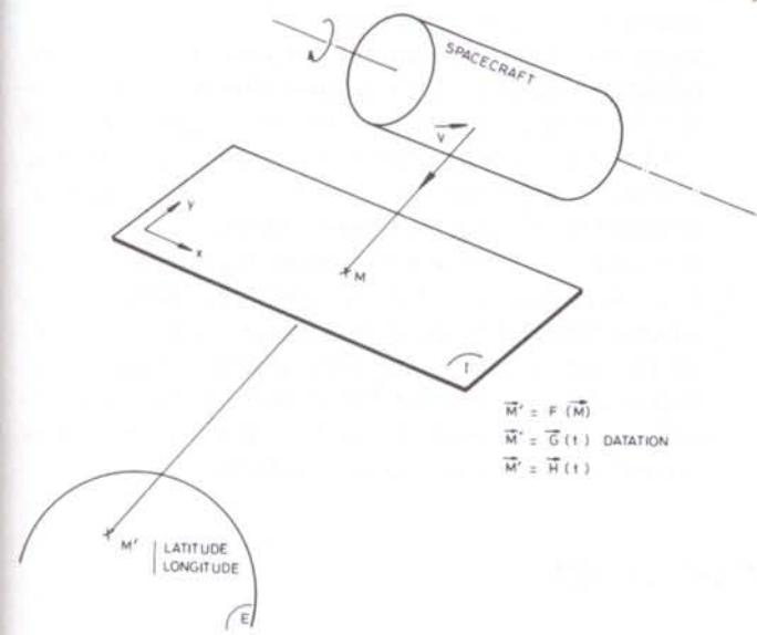
Figure 5 – Correspondence between image plan and the earth's surface.
