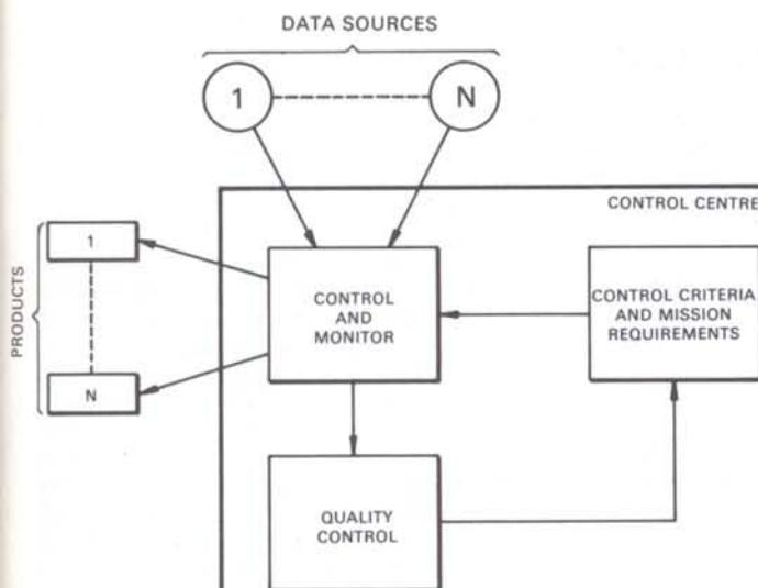
Figure 2 – The tasks of the Control Centre.
