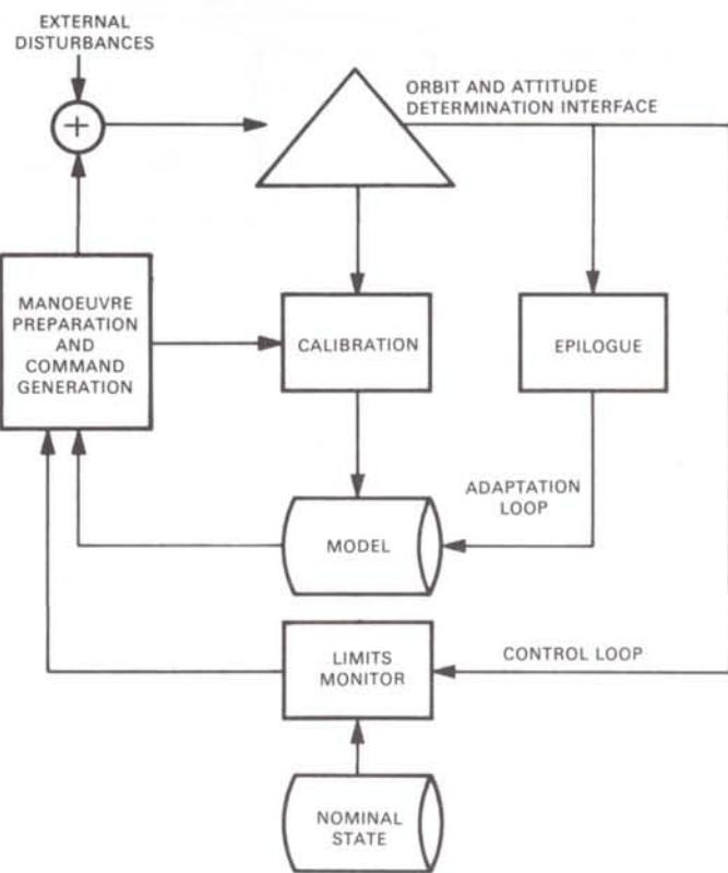
Figure 4 – Control flow for the orbit attitude control system.
