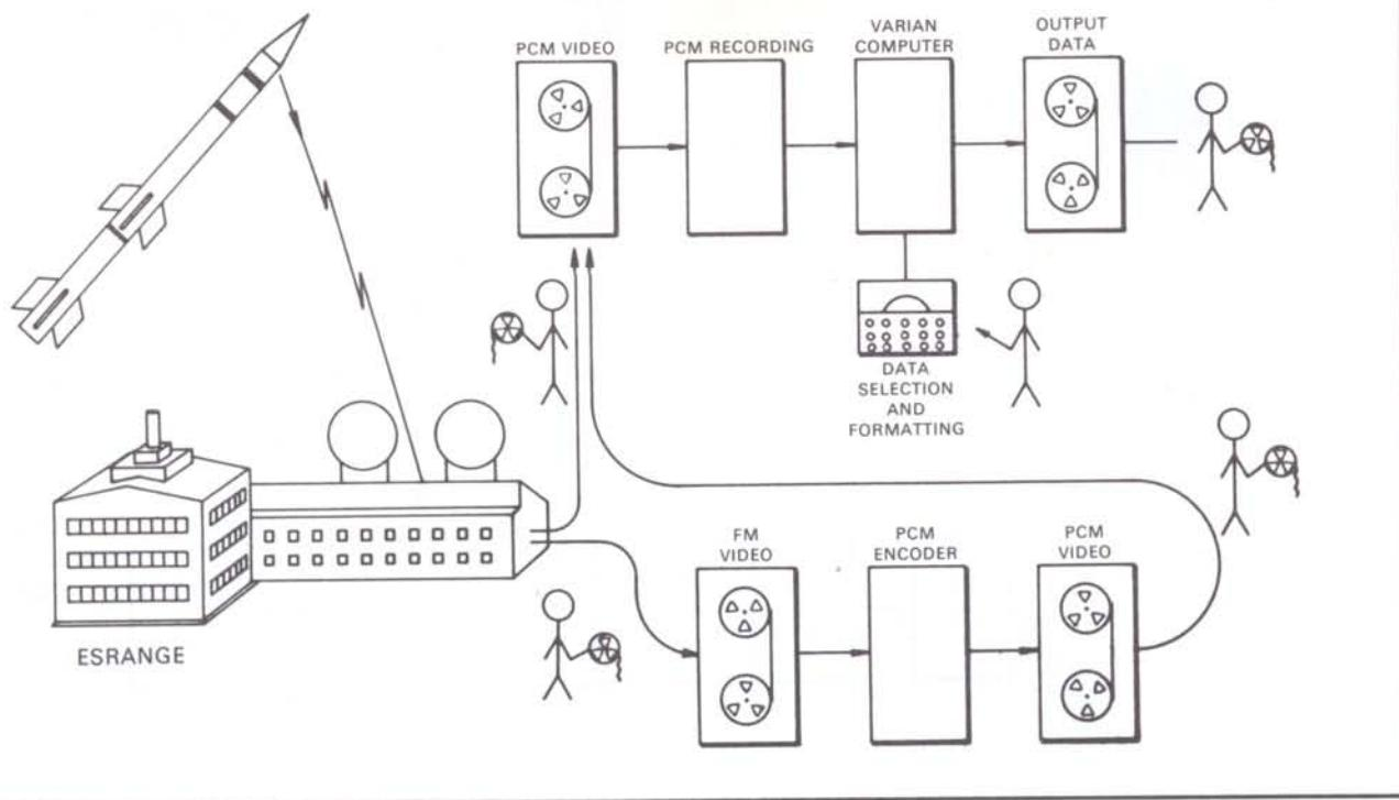
Figure 1 – Esrange telemetry data-handling system.
