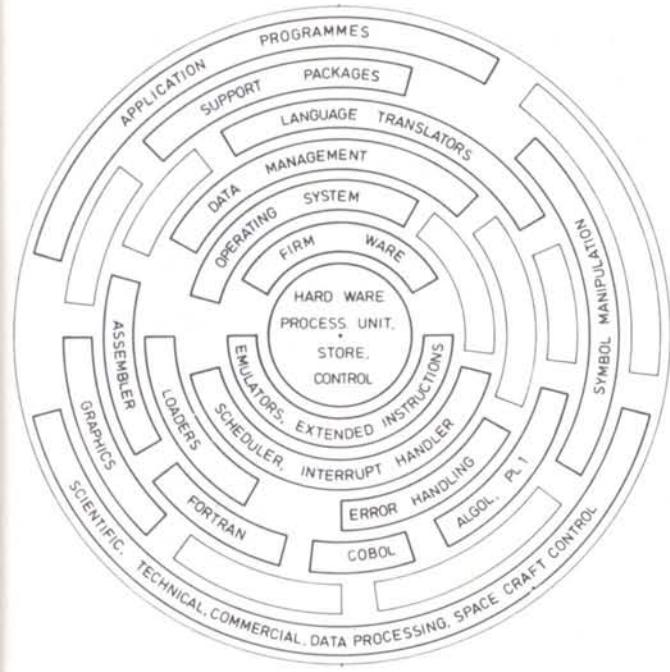
Figure 1 — Model of the relationship between hardware and software in a computer.
