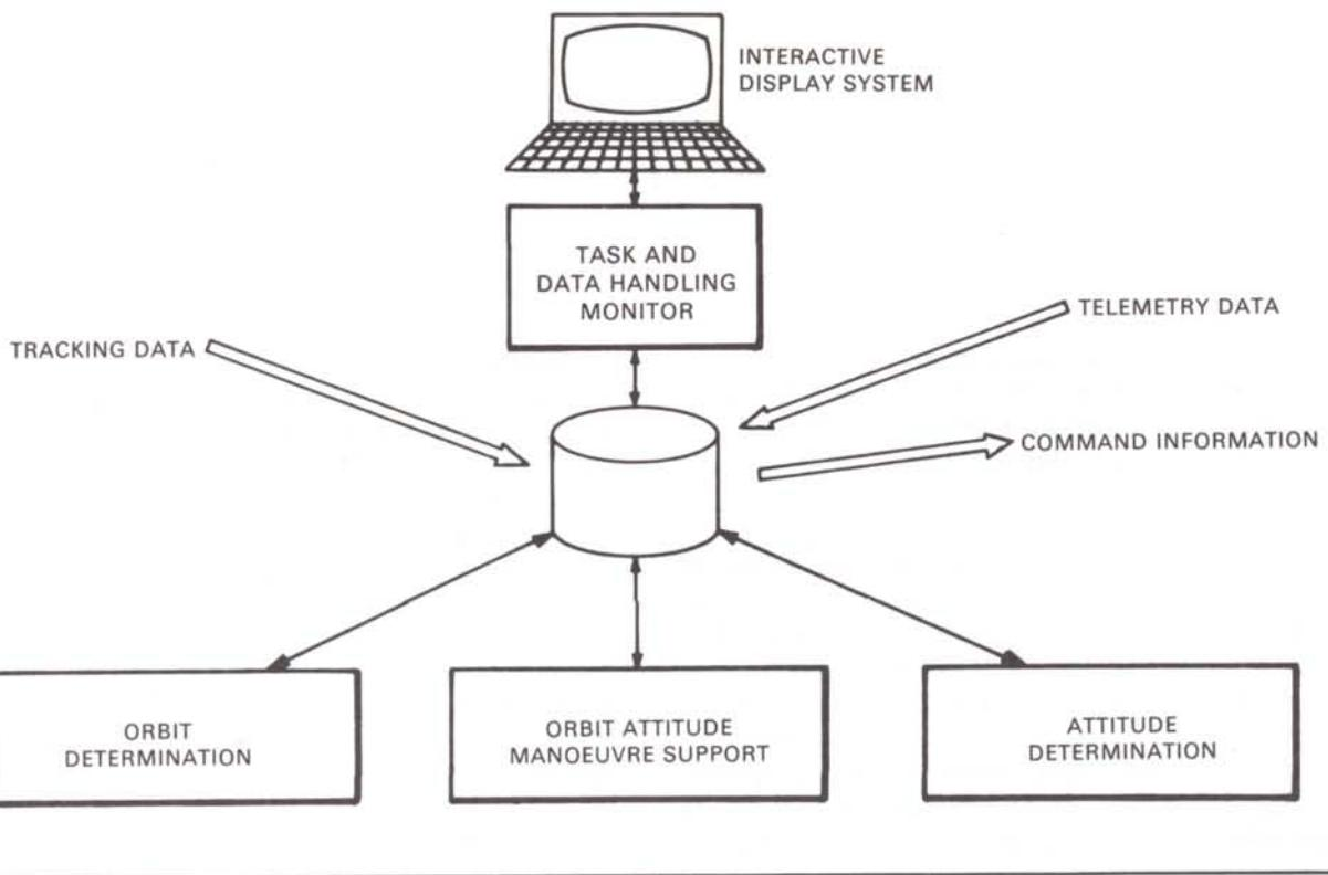
Figure 1 – MSSS orbit attitude system.
