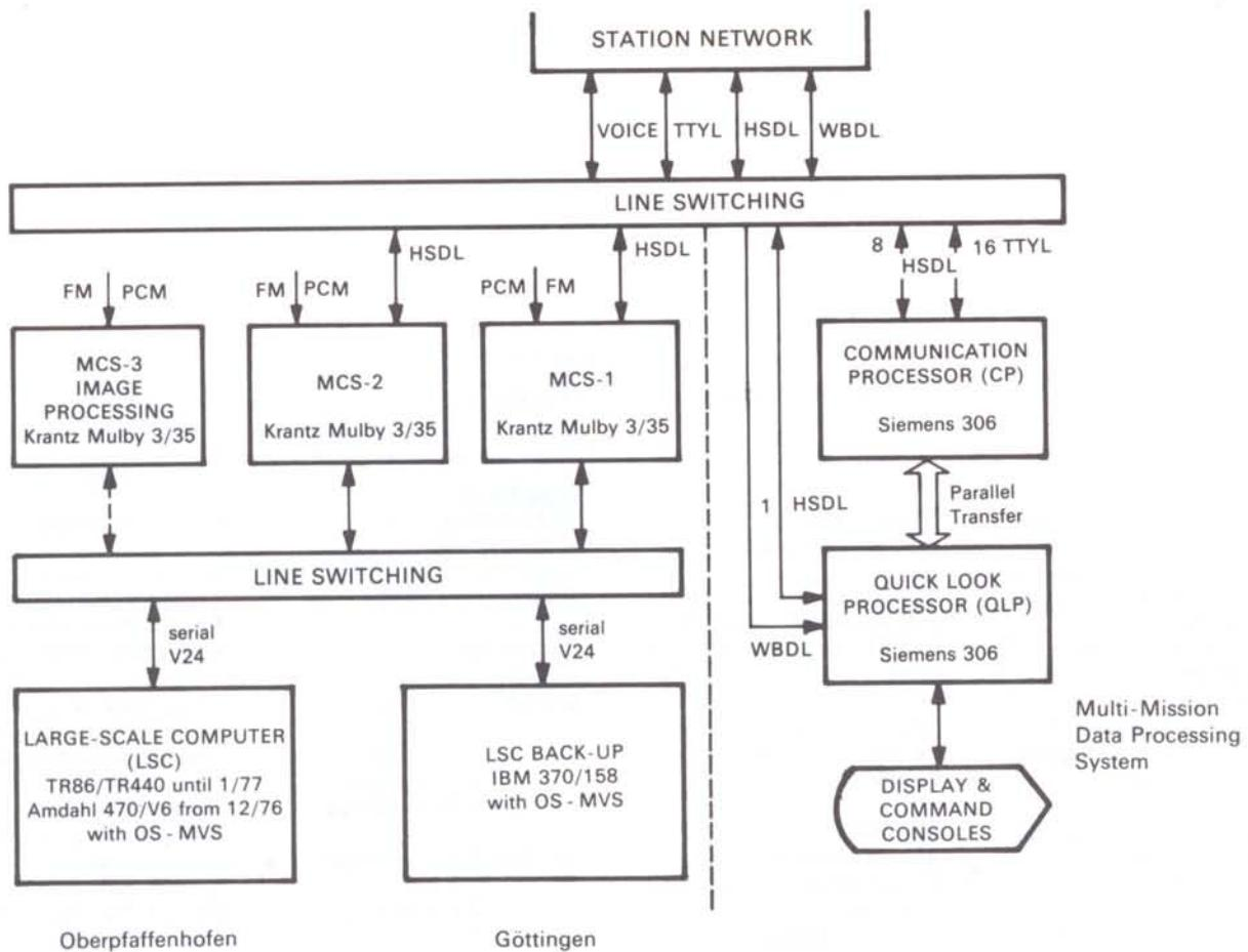
Figure 1 – DFVLR-GSOC computer configuration.
