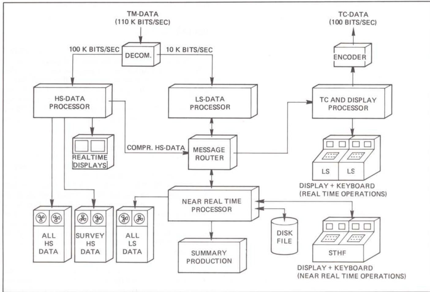
Figure 2 – GEOS spacecraft-control and data-handling facilities available at ESOC.
