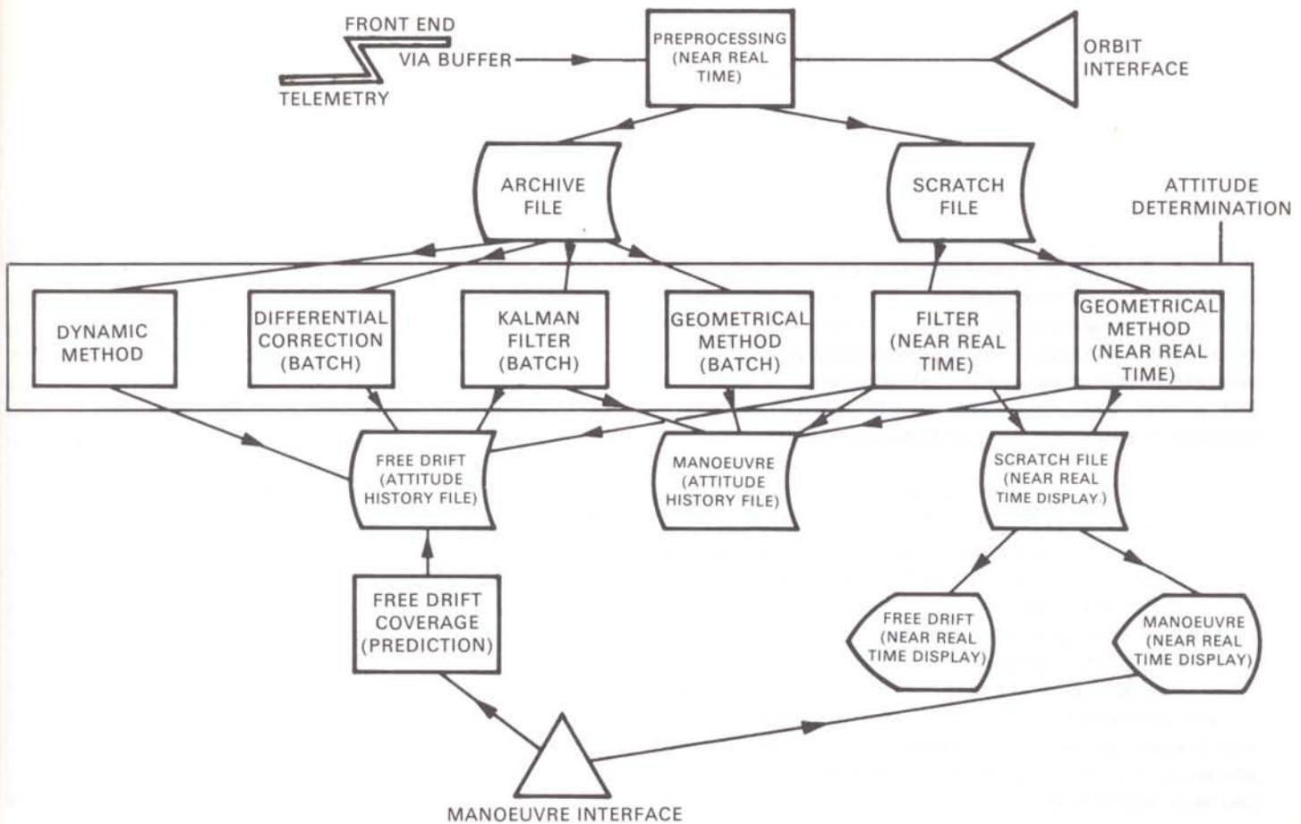
Figure 3 – MSSS attitude determination subsystem (spin-stabilised satellites).
