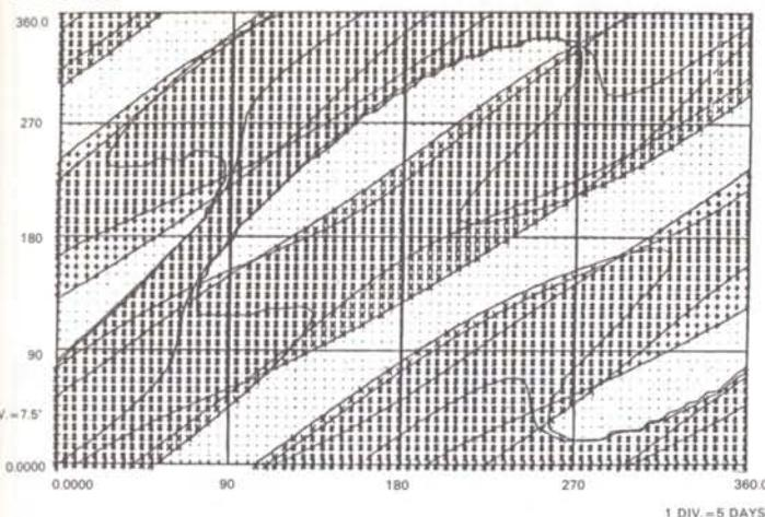
Figure 2 – Launch window into transfer orbit for a synchronous satellite, open in the lightly dotted regions which comply with all constraints.
