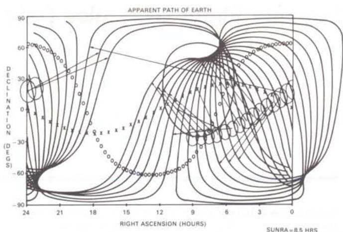
Figure 3 – Computer graphics generates the regions of sky obscured from a satellite in orbit. The envelope of the occulting earth's disc, enlarged by a safety zone, and the hazard caused by the sun are shown.
