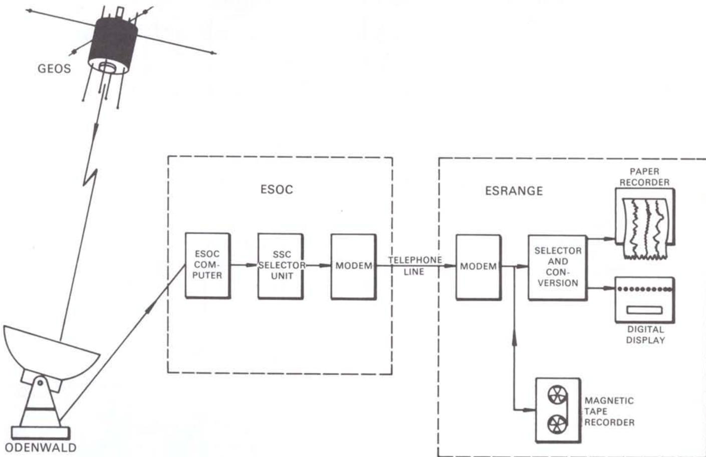
Figure 3 — Real-time satellite data link between Esrange and ESOC.
