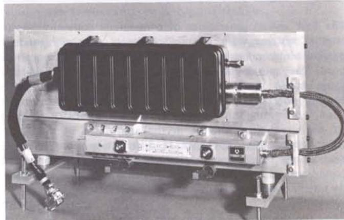
Travelling-wave-tube amplifier developed by Thomson-CSF, France and CGE-Fiar, Italy.
