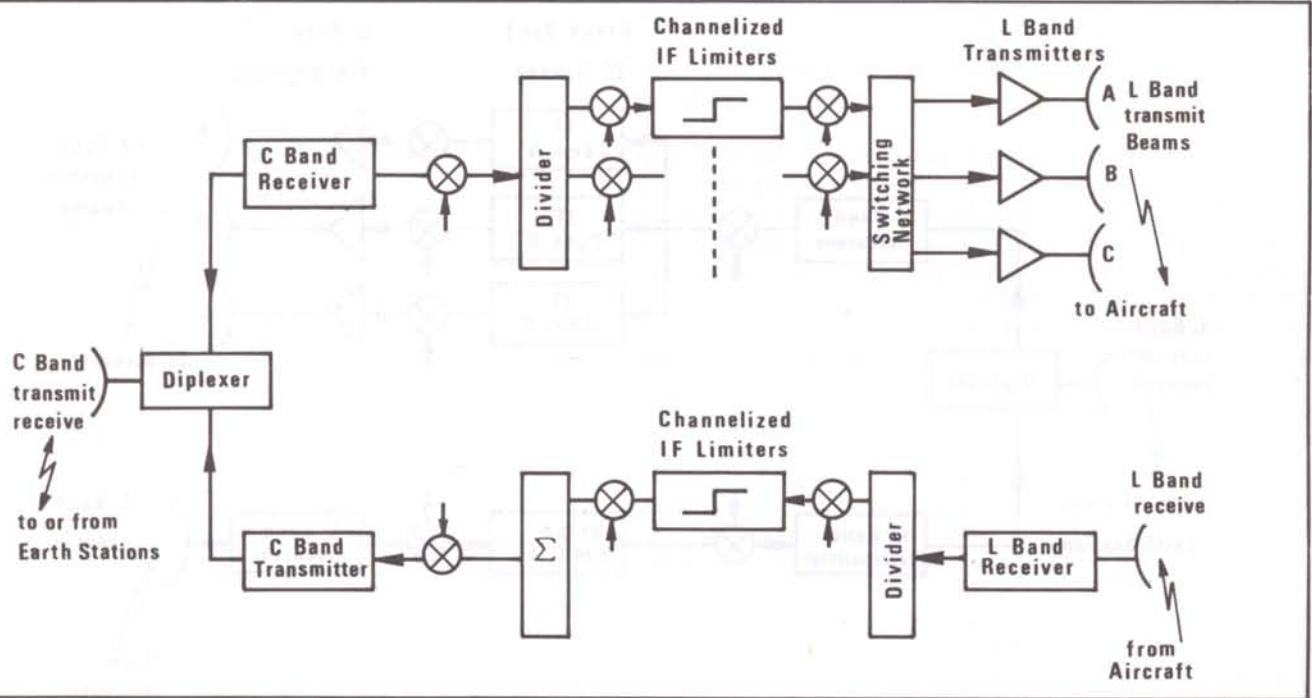
Figure 7 – Possible channelised transponder for Aerosat
