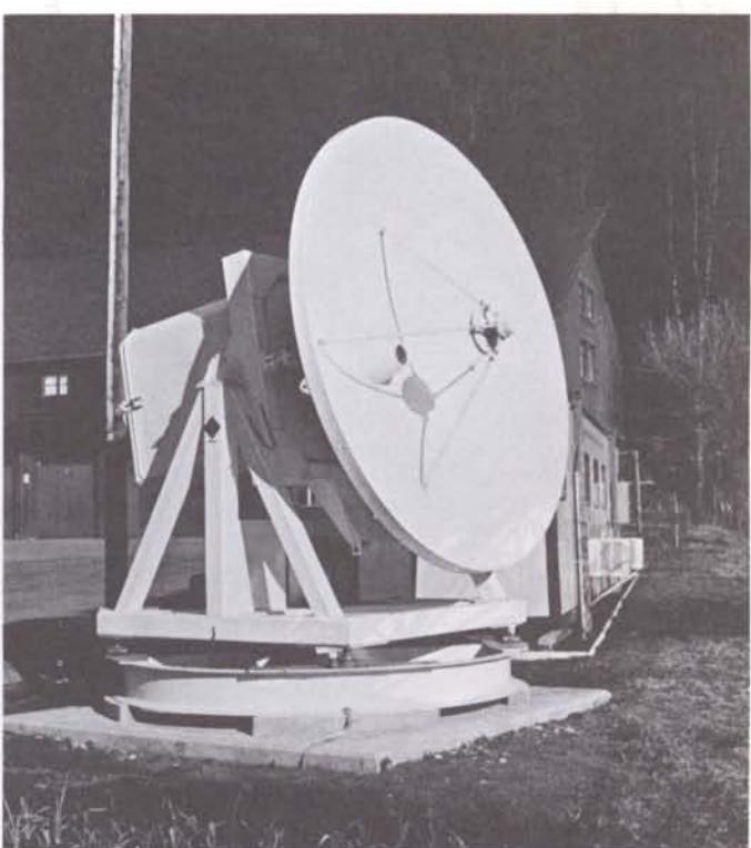
Figure 5 — Auxiliary 3 m diameter antenna
