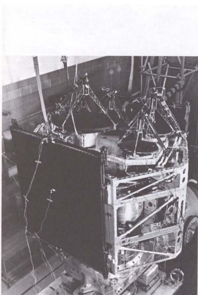
Structural-model vibration testing of OTS at IABG, Munich.
