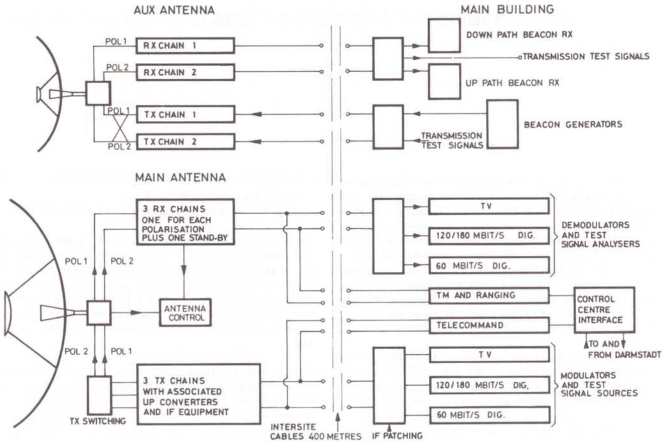
Figure 3 – Simplified block diagram of the SCTS facility at Fucino
