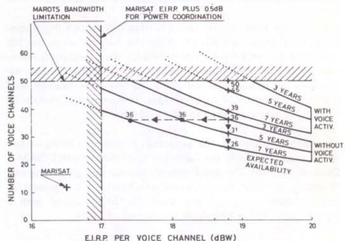
Figure 5 – Radiated power as a function of number of voice channels for Europe's Marots satellite and the USA's Marisat.
