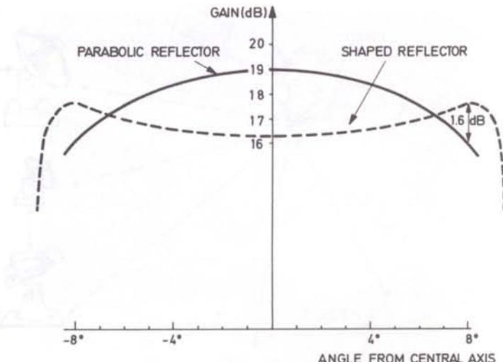
Figure 3 – Shaped-beam and parabolic antenna radiation curves, showing shaped reflector's superior edge-of-coverage performance.
