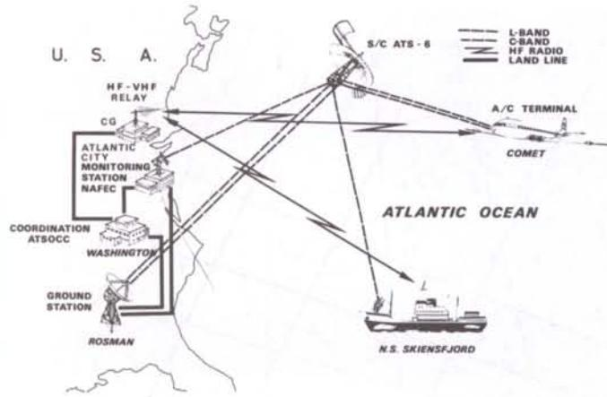
Figure 1 – Experiment configuration during the first, Atlantic City campaign.
