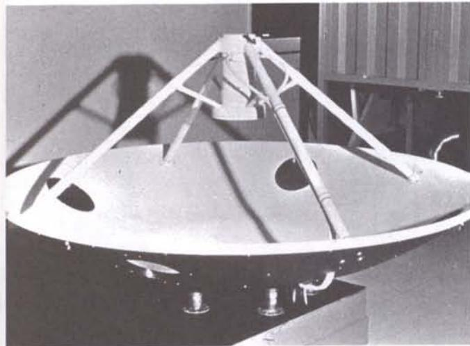
Figure 4 – Shaped-reflector antenna to be used on Marots.
