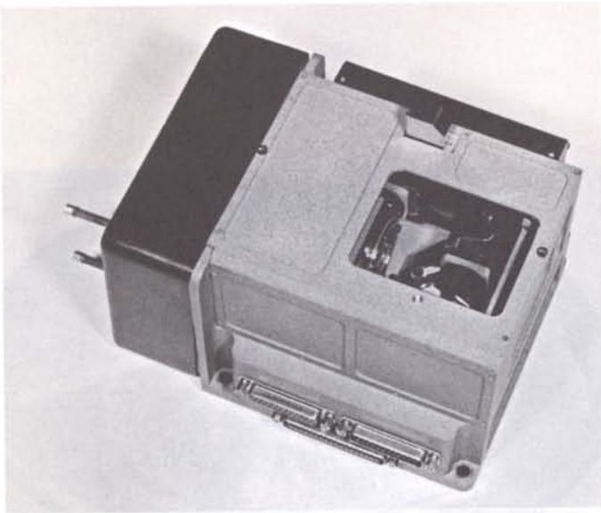
Infrared horizon sensor developed by Galileo, Italy.
