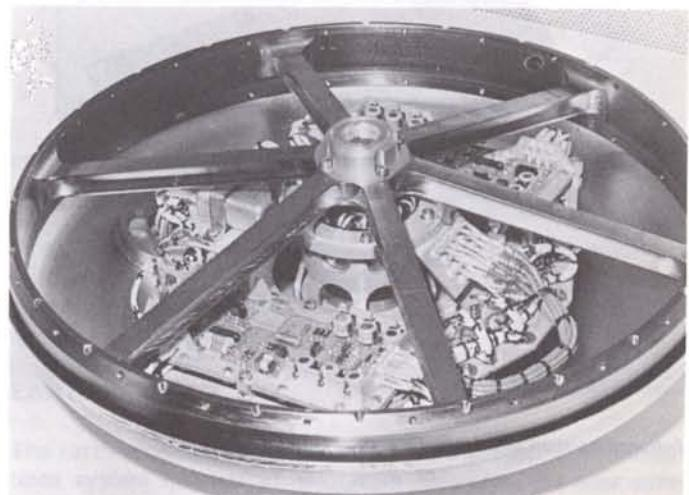
OTS fixed momentum wheel developed by Philips, The Netherlands.
