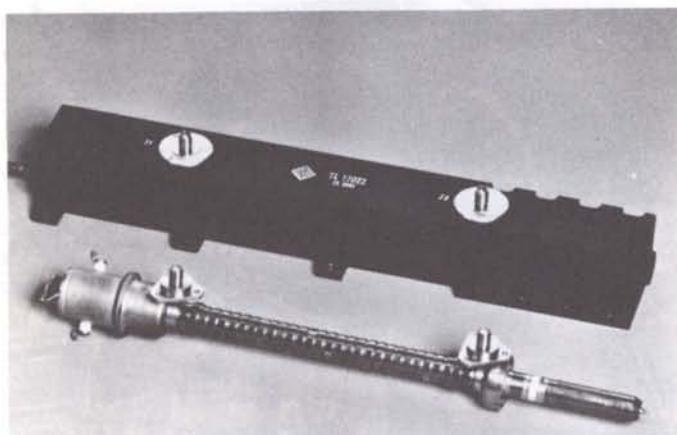
Travelling-wave tube developed by AEG, Germany.
