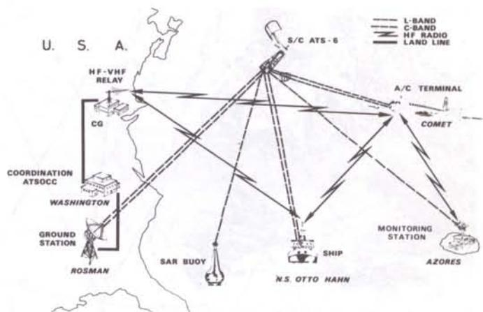
Figure 2 – Experiment configuration during the second, Azores campaign.
