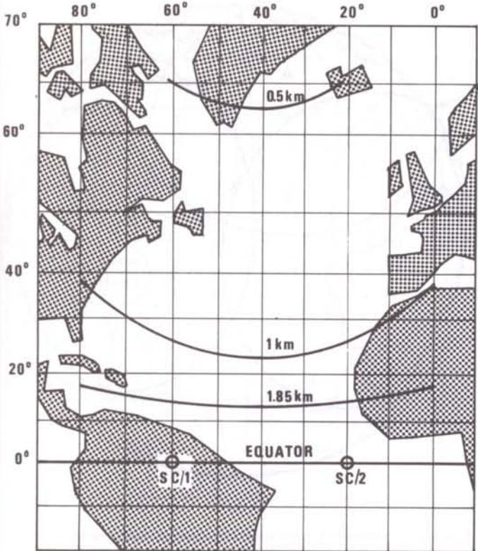
Figure 4 — Location errors over the Atlantic for two-satellite ranging system
