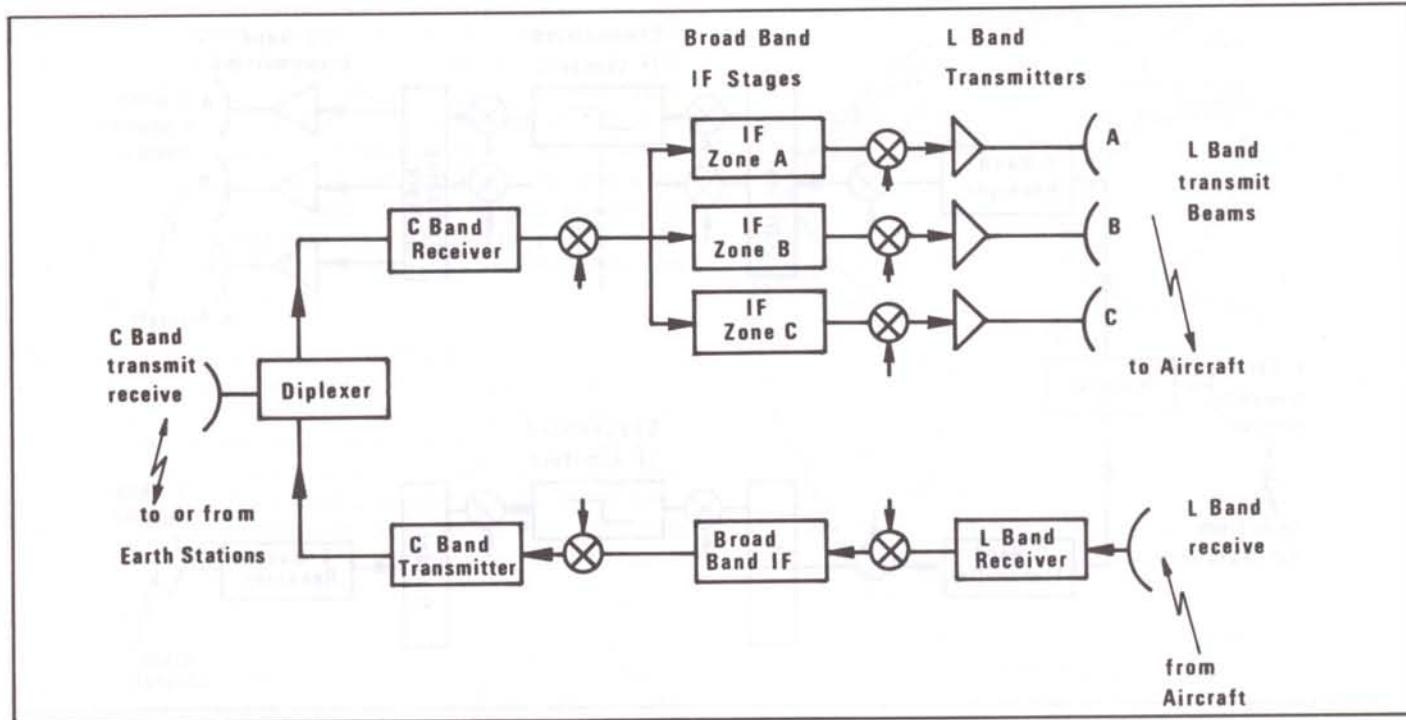
Figure 8 – Possible alternative broad-band transponder for Aerosat
