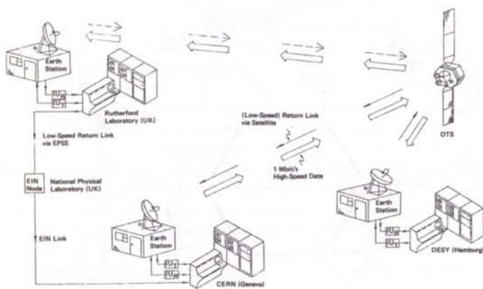
Figure 4 — Example of wideband satellite data distribution.
