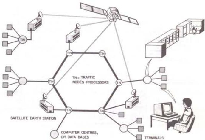
Figure 3 – Computer communication network employing satellite links.
