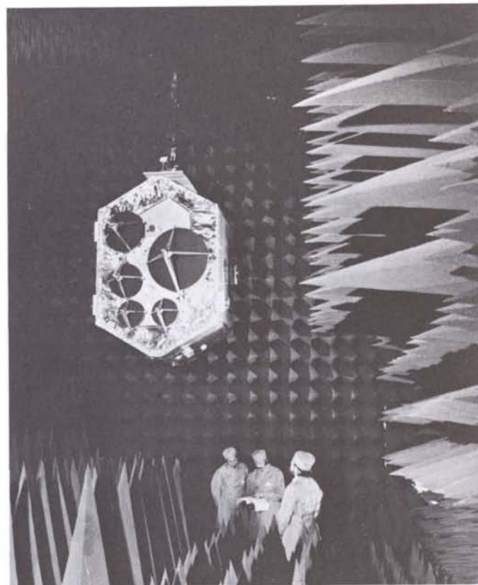
OTS model in acoustic chamber.
