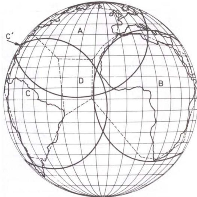
Figure 6 – Aerosat L-band transmit coverage, using three  $10^\circ \times 12^\circ$  ellipses (spacecraft at  $15^\circ W$ ).
