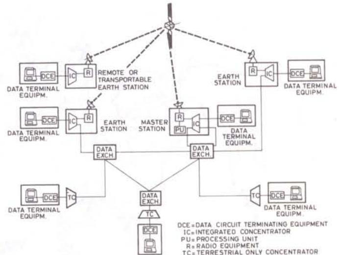
Figure 2 – Integrated terrestrial and satellite data communication system.
