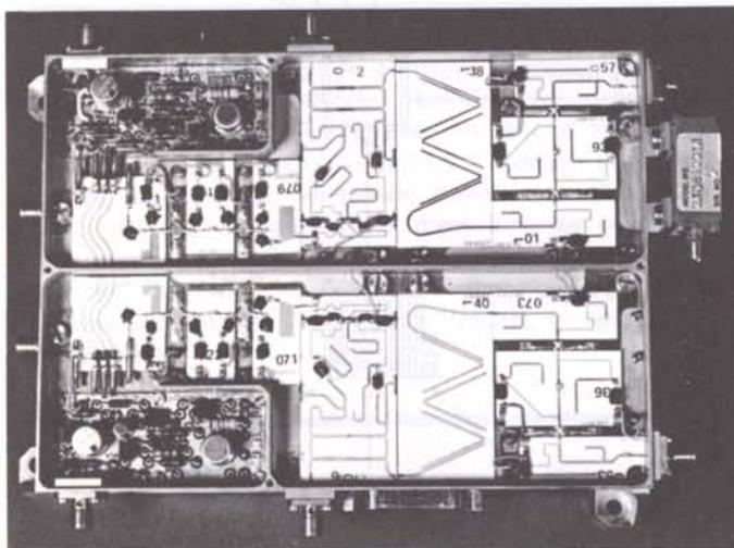
Figure 2 – Example of Marots payload integrated circuitry; the L-band receiver.
