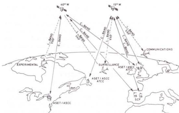
Figure 2 — The Aerosat communications system.
