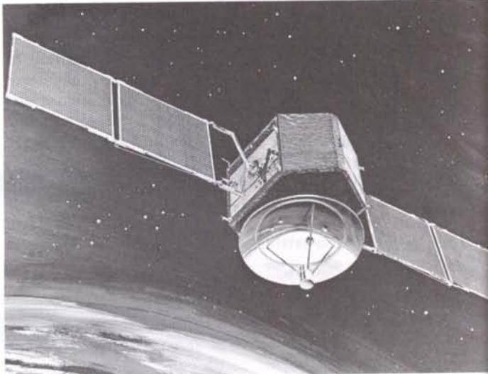
Figure 1 — The Marots three-axis-stabilised spacecraft.
