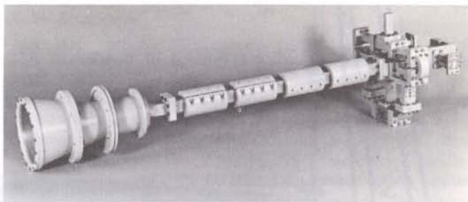
Figure 4 — Feed horn for the auxiliary 3 m antenna
