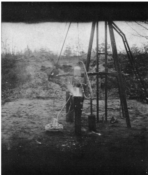
XI. Alcohol-oxygen rocket motor of the VFR, built in 1930. The photograph was taken from the observation dugout, about 25 feet from the test stand assembly. The thrust of the rocket blast was just above 130 pounds, and test runs were limited to thirty seconds because of the capacity of the oxygen tank. (See Fig. 29.)
