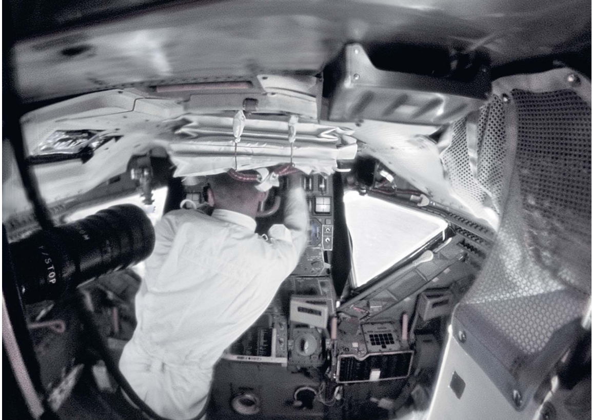
Aldrin looks through the Alignment Optical Telescope (AOT) during initial checkout. Armstrong would hook a strap to this to provide support for his legs in an attempt to sleep on the lunar surface. The live TV camera lens can be seen, left.
