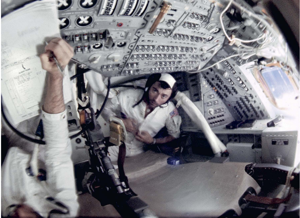
Stafford makes notes on the flight plan with his space pen as Command Module Pilot Young buttons up his coverall jacket. The Apollo coveralls had reinforced holes for medical connectors to pass and a slippery Teflon coating, which helped the astronauts dress with ease in a weightless environment.
