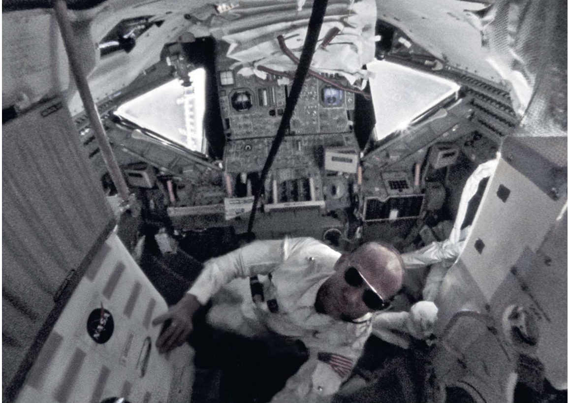
Aldrin in LM Eagle during initial checkout. His right hand is on Armstrong's PLSS backpack, which Armstrong would wear on the lunar surface. During descent and ascent from the surface Aldrin will occupy the right side of the cabin.
