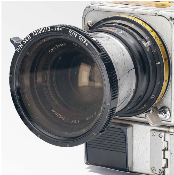
60MM BIOGON (WITH POLARIZING FILTER) ON THE HDC.
