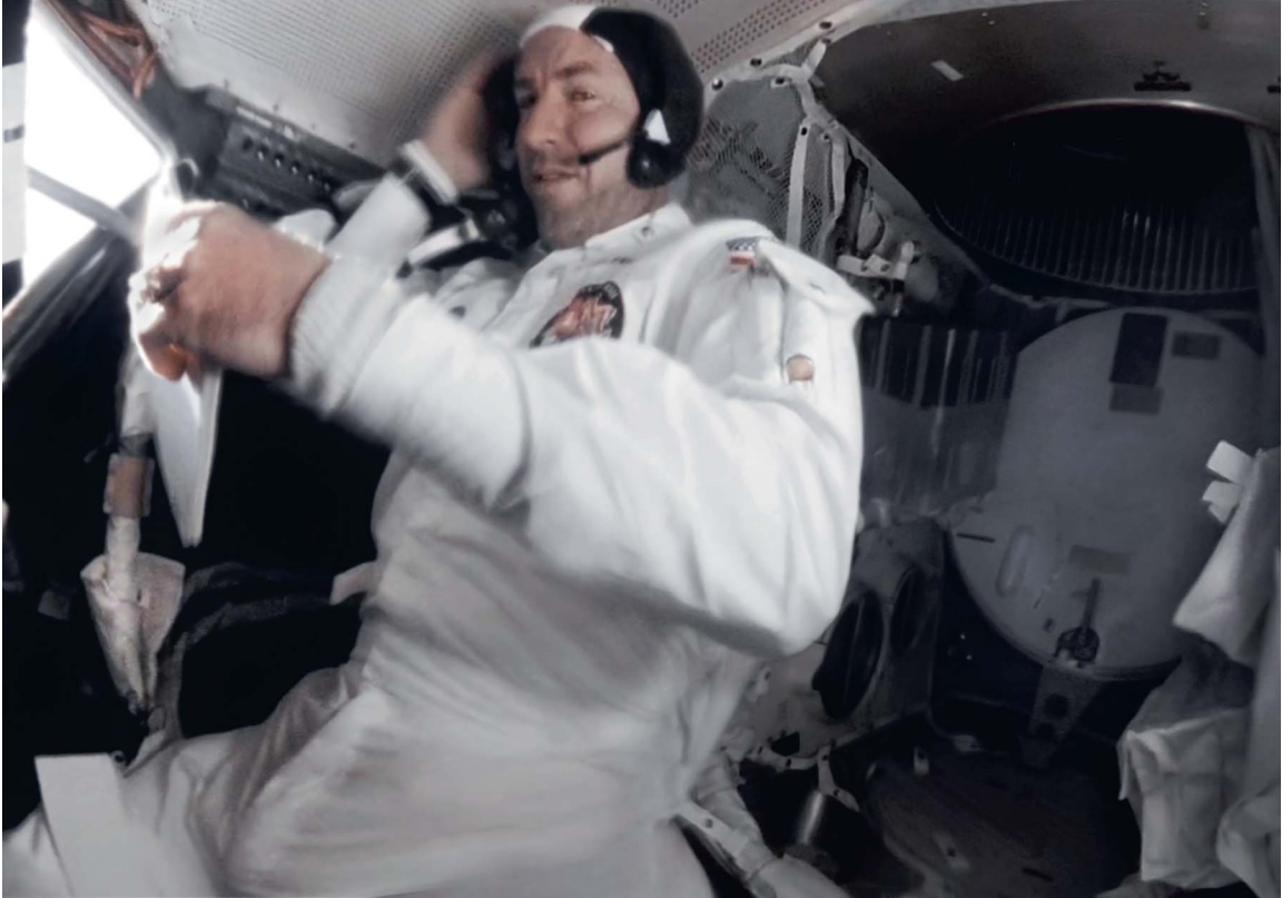
Lovell adjusts his communications headset; the “mailbox” scrubber and hatch/tunnel are behind him.
