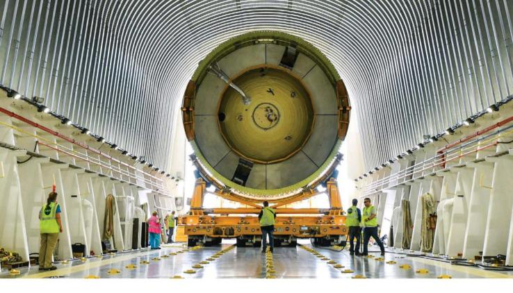
↑ Last June a test model of the 70-foot-long LOX tank was loaded on the Pegasus barge for transfer from Michoud to Marshall. For the SLS core stage, NASA needed a bigger boat and added 50 feet to the Pegasus.
